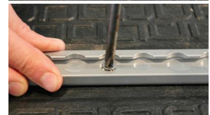
**NOTE:** Even if you've been careful, some track holes won't be perfectly centered over the interior dimples. That's OK, you're still mounting into the steel tubes
