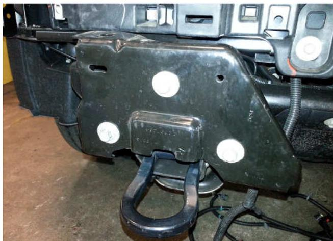
10. Remove the tow hook bolts if present. Tow hooks will be reinstalled.
