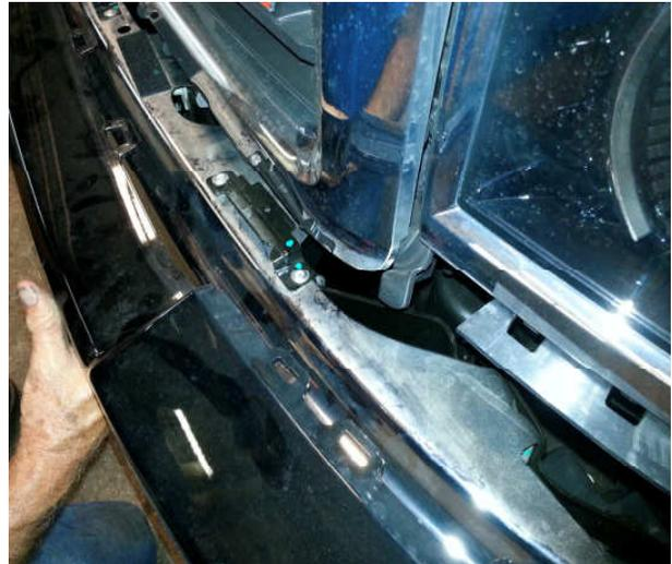
5. Open the hood and remove the plastic radiator cover. There will be several push clips.
