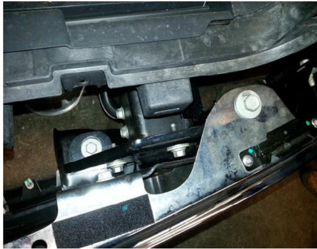
8. Lay the bumper down then remove the sensor and fog light wires (if present) from the bumper. **Do not unhook sensor plug.**
