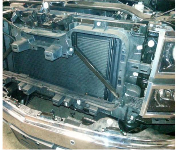
7. Remove the factory bumper by removing the two 18mm bolts from each side of the frame. They will be facing down. *See photo*
