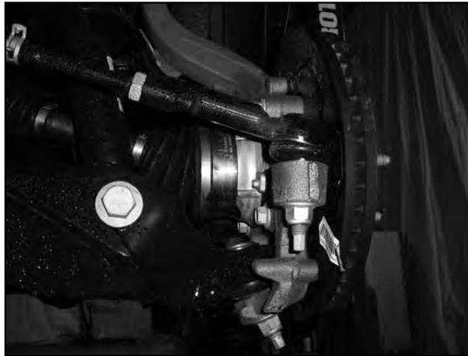
9. Remove the upper ball joint nut and thread back on a couple of turns by hand. Strike the knuckle near the ball joint to dislodge it from the knuckle. (Fig 5) Remove the nut and remove the ball joint from the knuckle. Save nut. Allow the knuckle to rest back away from the front strut.
