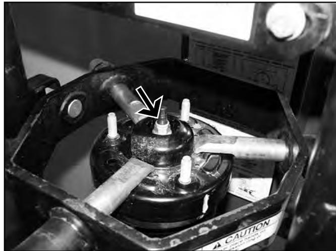
14. Working on the upper strut mount, remove the rubber isolator (Fig 9) from the strut mount and install the provided preload ring (02082 - Fig 10). Reinstall the rubber isolator and line up the align marks made earlier.
