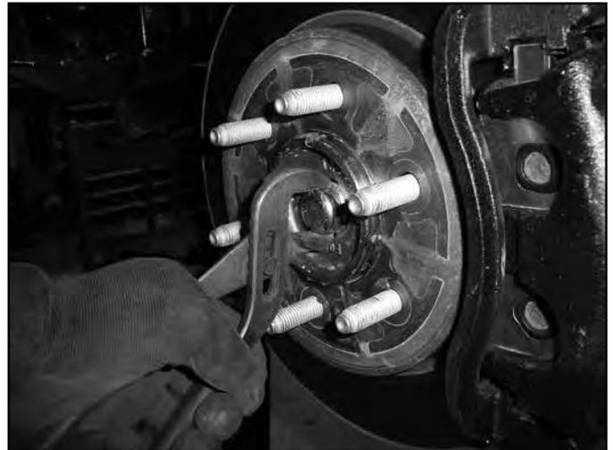
6. Locate the small dust cap on the hub. (Fig 3) Carefully remove the cap using a pair of channel lock (or any wide jaw style) pliers. Save dust cap.
