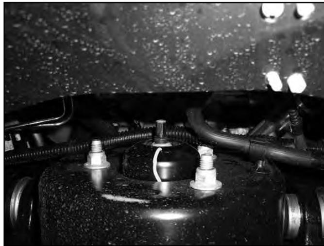
11. Remove the lower strut mount bolt/nut at the lower control arm. (Fig 4) Lower the control arm and remove the strut from the vehicle. Save lower strut hardware.
