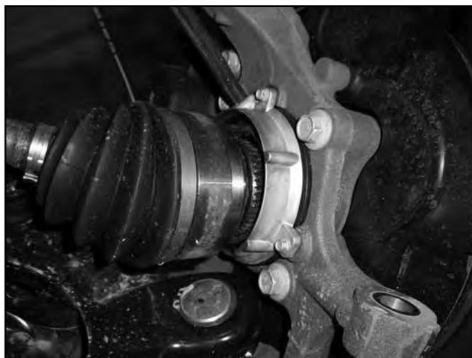
21. Be sure the CV is properly seated in the hub and reinstall the original retaining nut. Torque nut to 20 ft-lbs. Reinstall the hub dust cap by tapping in place with a small hammer.
