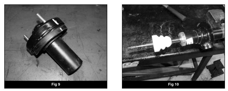
17. Set the modified strut mount aside and locate the OE strut. Remove the bump stop from the strut rod and set aside (Fig 10). Slide the coil seat up the strut body so it rests against the upper strut seal cap (Fig 11). Note: There may be corrosion present holding the coil seat in place. If so tap it with a hammer to break it loose.
