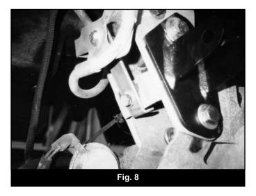
30. Loosen the turn buckle clamps on the drag link and rotate 180 degrees. This will allow the drag link to be connected with the new pitman arm. Install drag link into pitman arm and tighten OE nut. Be sure to use a new cotter pin. Rotate the turn buckle clamps to the top side of the drag link to gain clearance for the steering stabilizer. Tighten turn buckle clamps to 45 ft.lbs.
