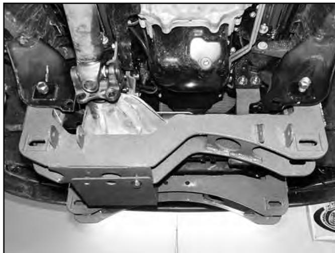
46. Install the new differential skid plate to the front crossmember with  $\frac{1}{2}$ " x 1-1/4" bolts and  $\frac{1}{2}$ " SAE washers (BP #660) into the welded nuts in the crossmember. Install the back of the skid plate to the rear crossmember with  $\frac{1}{2}$ " x 1-1/4" bolts and  $\frac{1}{2}$ " SAE washers (BP #660) into the welded nuts in the crossmember. Leave hardware loose.
