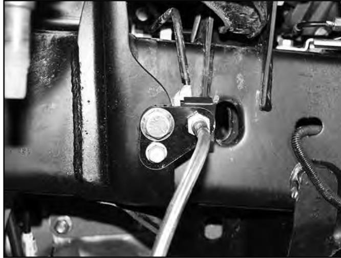
12. **6 inch kit only:** Route the new stainless steel brake line through the relocation bracket and attach it to the hard line. Tighten the fitting securely. Fasten the line to the bracket with the provided retaining clip.
