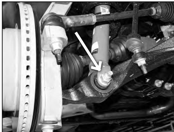
25. Remove the upper and lower ball joint nuts. Reinstall the nuts a few turns by hand. Separate the upper and lower ball joints from the steering knuckle using the appropriate puller. Take care not to damage the ball joint.
