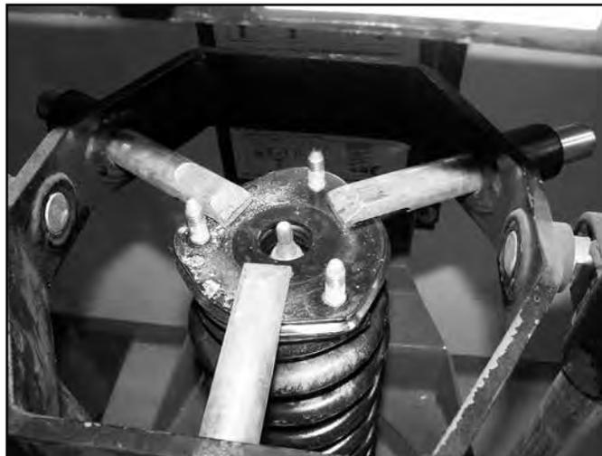
52. Place the provided preload spacer (01278) between the plastic coil seat and the rubber isolator (Fig 18).
