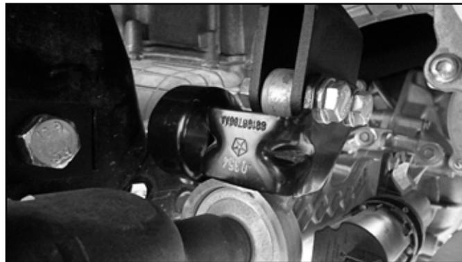
40. Using a jack (and an assistant to aid in balancing) raise the differential up to the new brackets.
