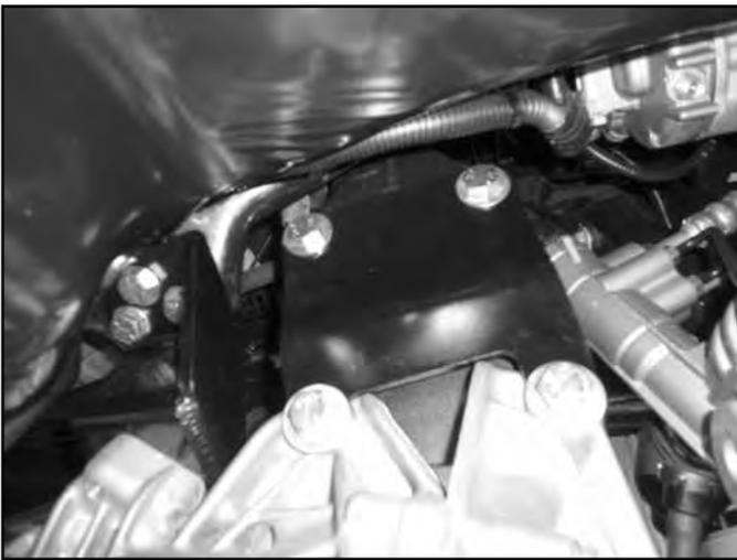
39. Install the driver's side rear differential drop bracket (01238) to the frame with three 1/2" x 1-1/2" bolts and 1/2" SAE washers (BP #660). (Fig. 12) The bracket will have the gusset plate towards the front of the vehicle. Leave hardware loose.
