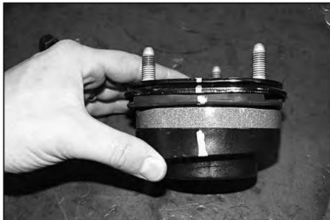
53. Reassemble the strut as it was taken apart by aligning the index marks made earlier. Fasten the assembly with the OE strut nut. Torque nut to 50 ft-lbs.
