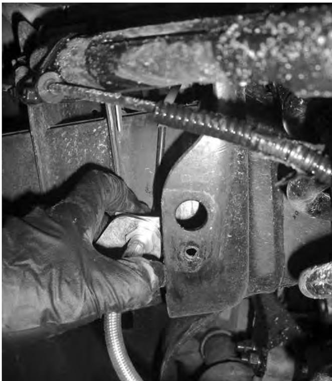
16. **4 inch kit only:** Attach the provided brake line relocation bracket to the frame where the original line mounted. The brakeline bracket will offset towards the rear of the vehicle. Torque the factory bolt to 10 ft-lbs and the 1/2" bolt to 50 ft-lbs.
