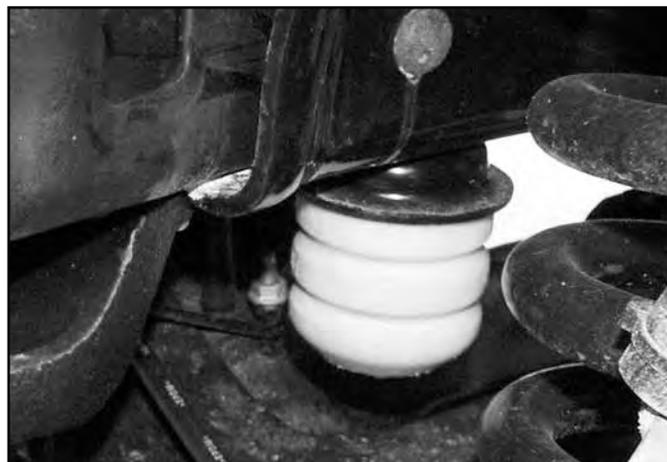
23. Install the cup on the provided bump stop extension with a 5/16" x 1" bolt, nut and 5/16" SAE washers from bolt pack #431. The alignment tab on the bump stop cup will fit in the second hole in the extension. Torque hardware to 20 ft-lbs.
