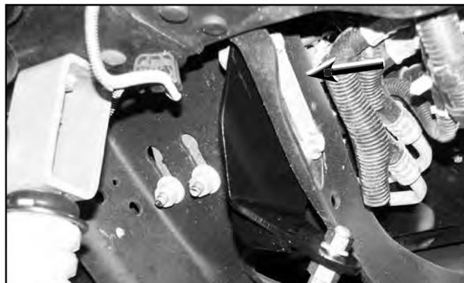
13. Install the provided shock stud in the new stabilizer bracket up through the bracket so that the stud points down (Fig 6). Torque to 50 ft-lbs.
