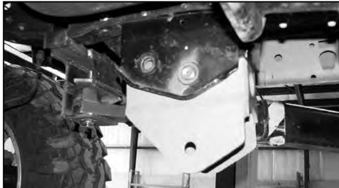
28. Swing the radius arm up into the new bracket and fasten with the original mounting hardware. Leave loose.
