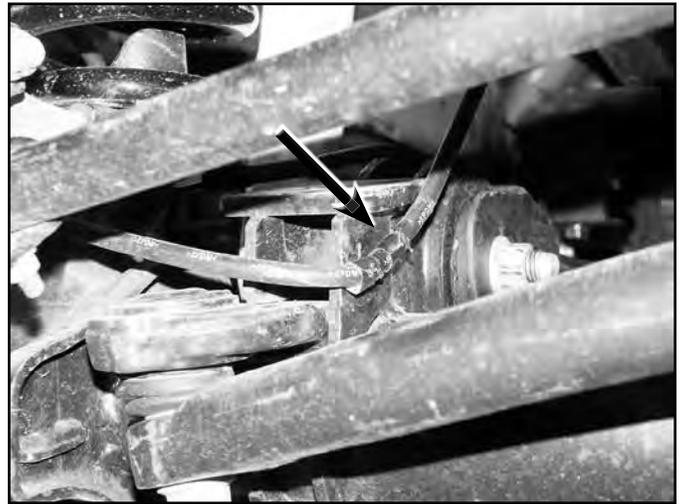
8. Disconnect the sway bar end links from the axle mounts. Retain hardware.
