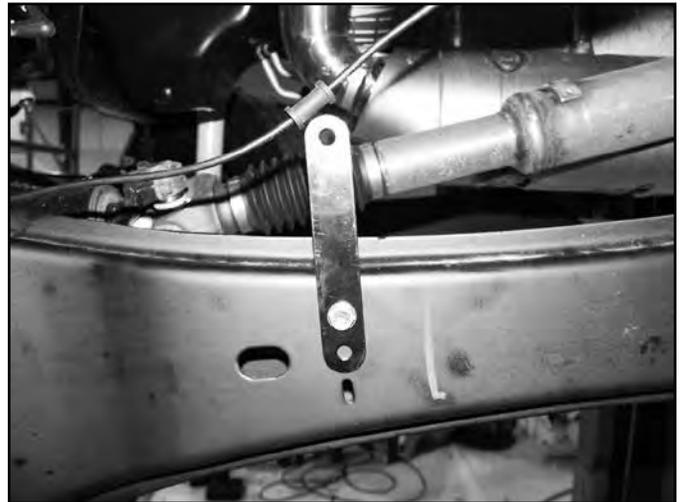
39. Install the ABS line in the retaining tab on the radius arm. Reinstall the plastic ABS tab (near the axle) to the original hole in the radius arm.
