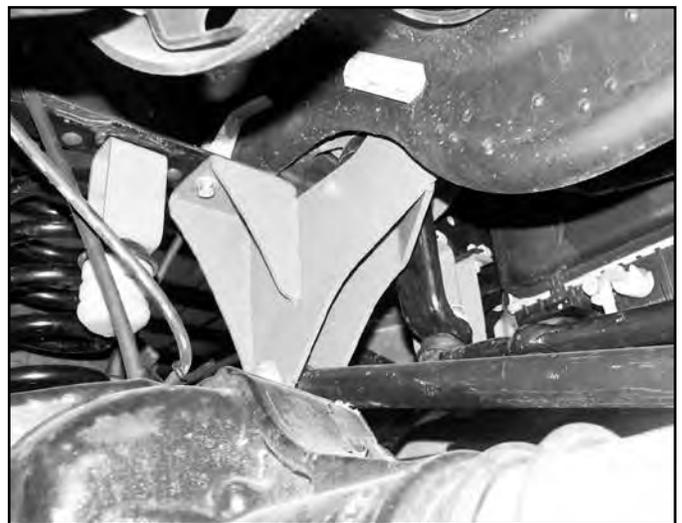
22. Pull the OE front bump stops free from the bump stop cups and remove the bolt mounting the cup to the frame (Fig 8).
