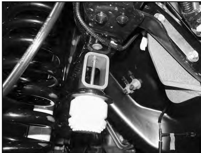
25. Loosen the four radius arm-to-axle mounting bolts but do not remove. Once again, ensure that the front axle is well supported.
