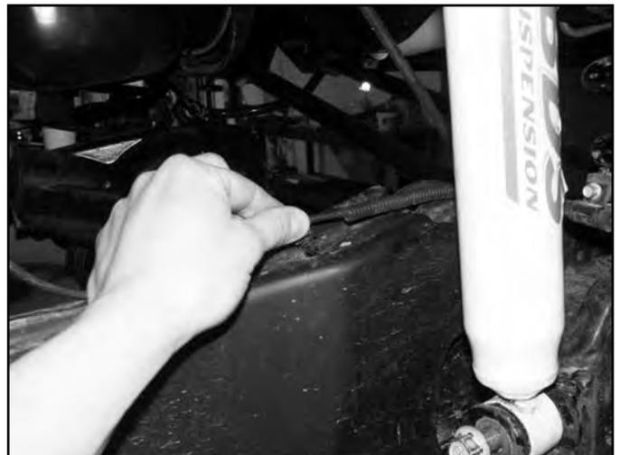
11. Disconnect the OE steering stabilizer from the drag link and the frame mount. Remove the two nuts (and bolt tab) mounting the stabilizer frame mount and remove it from the vehicle. Retain the frame bracket mounting hardware.
