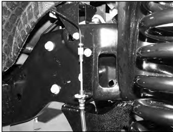
45. Properly bleed the brake system of air and top off the brake fluid reservoir with the proper type of fluid (see owners manual).
