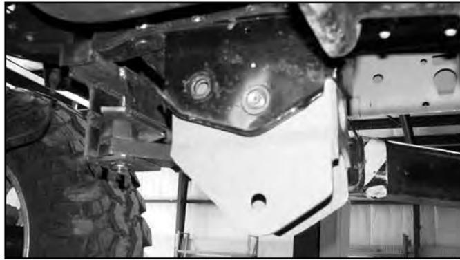
28. Swing the radius arm up into the new bracket and fasten with the original mounting hardware. Leave loose.
