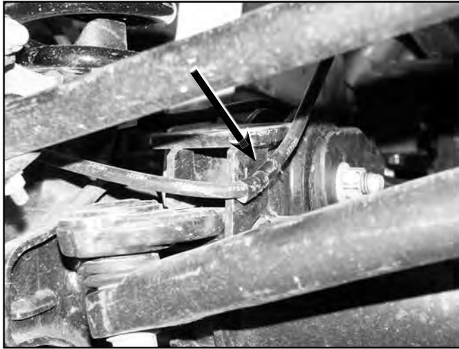
8. Disconnect the sway bar end links from the sway bar. Retain hardware.
