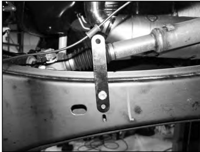
39. Attach the ABS line to the top hole in the bracket with the provided wire clamps and ¼" hardware (BP 434). Tighten hardware securely.
