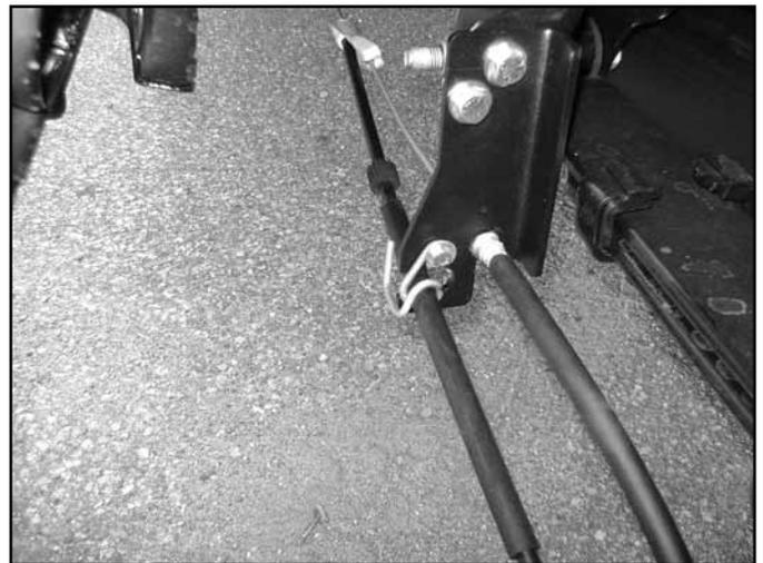
90. Reconnect the parking brake cable at the junction. When reconnected, remove the clamp to allow the cable to return to its normal tension. Attach the parking brake cable through the relocation bracket through the slot in the bottom. Note: Models with automatic retracting running boards will require an additional bracket to have the cable clear the linkage. This optional accessory bracket kit #123018 is available separately.
