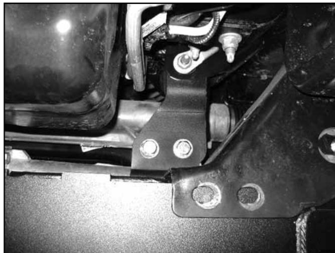
42. Torque all of the differential mounting hardware to 95 ft-lbs (10 total). Attach the differential breather tube. On 2014+ models - Remove the differential breather elbow from the plastic line and replace it with the provided hose and attach it to the differential.
