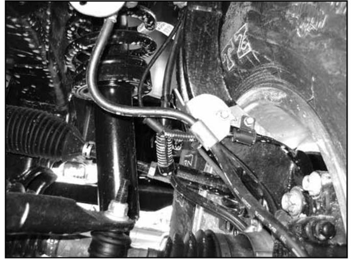
63. Install the sway bar to the new sway bar drop brackets with 7/16" x 1-1/4" bolts, nuts and 7/16" SAE washers (BP #772), run the hardware from top-down Attach the sway bar to the sway bar end links with the original hardware. Torque the 7/16" hardware to 45 ft-lbs. Torque sway bar link nut to 45 ft-lbs.
