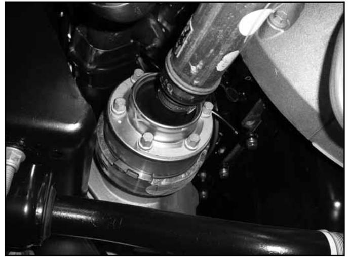
24. Remove the passenger's side CV only. Strike the shaft with a hammer to dislodge it from the splines. This will make handling the differential much easier. (Fig 12)
