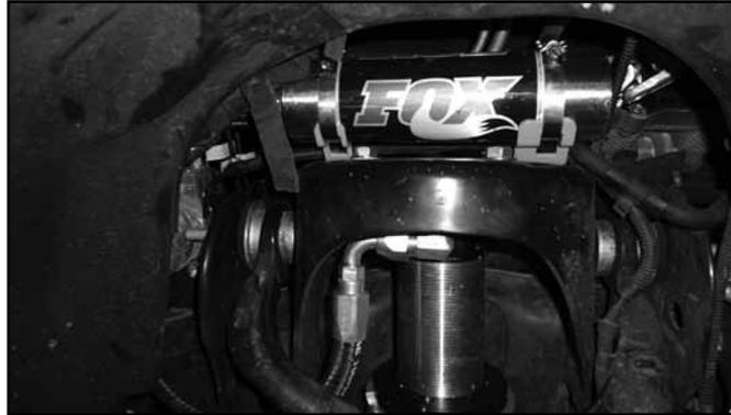
51. Remove the four hub bolts from the knuckle and remove the hub from the knuckle (Fig 24). Inspect mounting surface of the hub assembly and clean any dirt or corrosion off as necessary.
