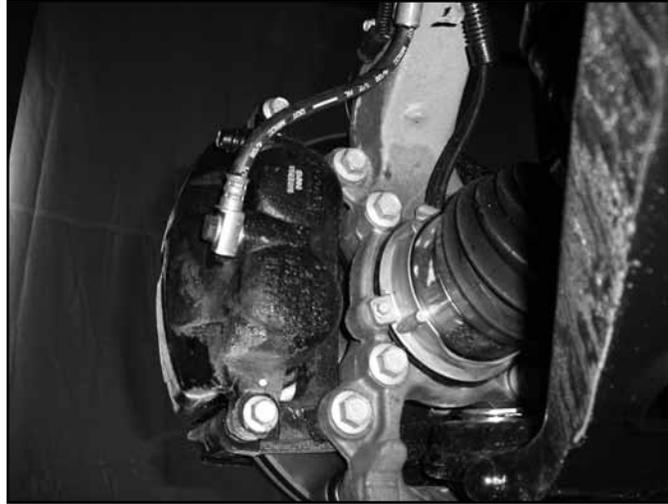
6. Remove the brake rotor and set aside.
