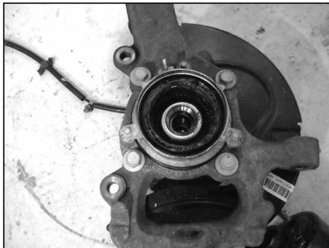
52. Install the hub into the corresponding new BDS knuckle (drv- 02065, pass- 02067) and fasten with the OE bolts. The ABS wire will be located at the 'top' of the hub. Use Loctite on the bolt threads and torque to 148 ft-lbs.
