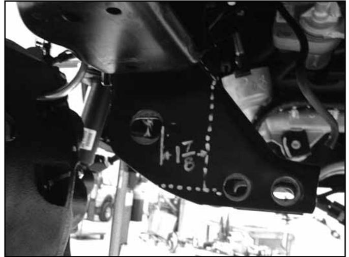
29. Connect the front cut line straight to the back face. This will require trimming minor trimming on the factory differential mount tab. (Fig 14c, 14d)
