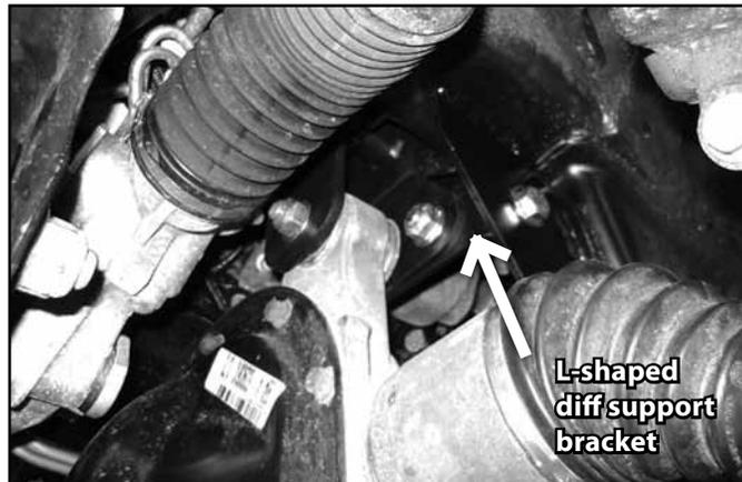
41. Install the offset differential support bracket to the backside of the passenger's side differential bracket using the hardware that was just installed and 9/16" x 1-1/4" hardware to the BDS crossmember. Leave hardware loose. (Fig 20b)
