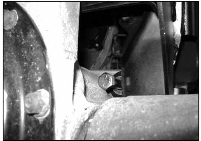
40. Fasten the L-shaped support bracket to the rear of diff drop bracket. Fasten to the passenger's side bracket with the same size hardware (BP #772). Attach all hardware from the front to rear. Leave all hardware loose at this time. (Fig 20a).
