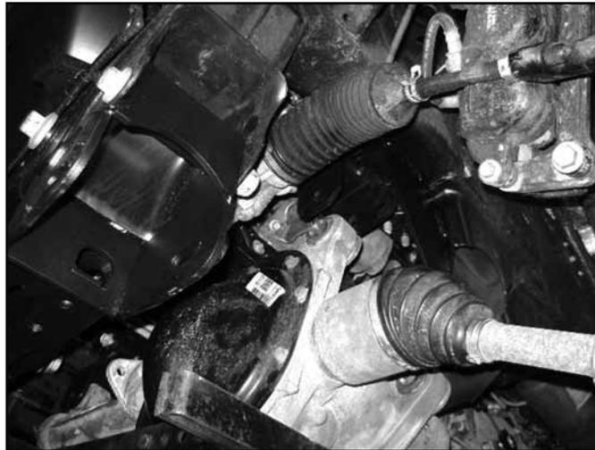
38. Install the new rear crossmember (02069) in the rear lower control arm frame pockets. Attach the rear crossmember with the sway bar drop brackets with new 18mm bolts and washers. Run bolts from rear to front (Fig 22a). Leave hardware loose. Ensure the hole that was drilled in the frame pocket lines up to the differential mounting hole in the bracket. (Fig 19a). Do not tighten hardware at this time.
