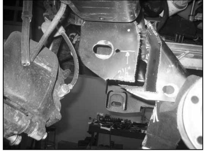
31. The passenger's side control arm pocket must also be trimmed. Measure down 1-3/4" and make a horizontal cut line. The cut will stop where the vertical offset begins. (Fig 16)
