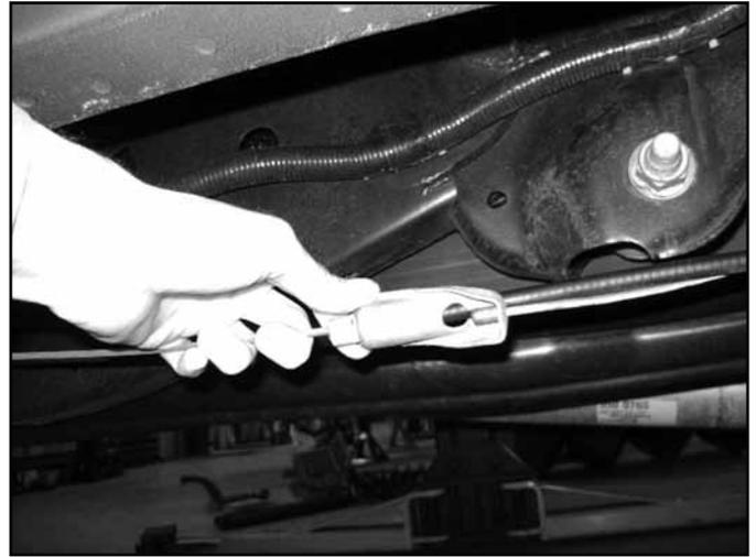
79. Compress the retaining tabs and remove the driver's side cable from the spring hanger (Fig 32). It will be relocated and reconnected later.
