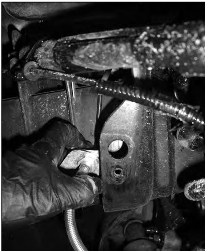
15. **4" kit only:** Attach the provided brake line relocation bracket to the frame where the original line mounted. The brakeline bracket will offset towards the rear of the vehicle. Torque the factory bolt to 10 ft-lbs and the ½" bolt to 50 ft-lbs.
