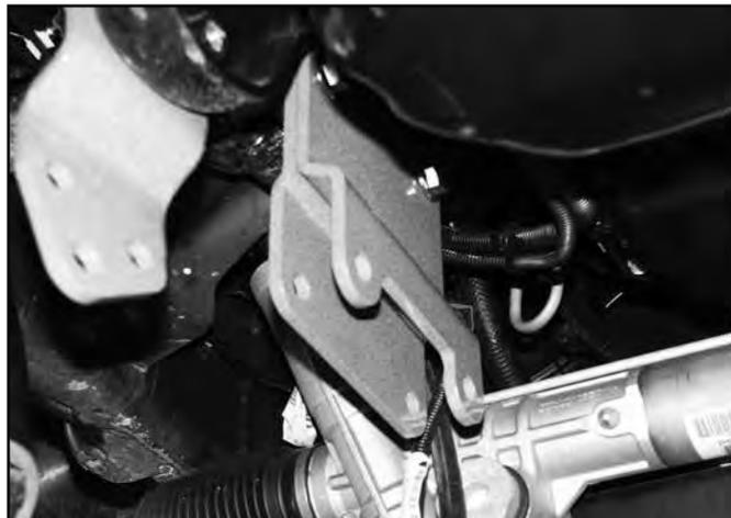
40. Install the driver's side rear differential drop bracket (01238) to the frame with three 12mm x 30mm bolts and 1/2" SAE washers (BP #617) into the existing welded nuts on the frame. (Fig. 12) The bracket will offset toward the outside of the vehicle with the gusset to the front. Leave hardware loose.
