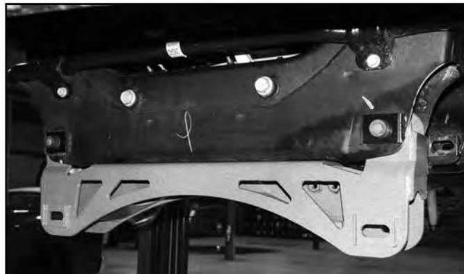
46. Install the new rear crossmember (01296) in the OE rear lower control arm pockets and loosely fasten with the provided 18mm x 150mm bolts, nuts in conjunction with the provided rectangle cam slot washers (01264). Run the bolts from front to rear and leave loose at this time. (Fig. 13b)
