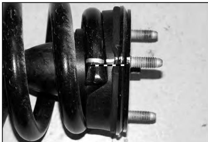
**! Caution** *Coil spring is under extreme pressure. Improper removal/installation of coil spring could result in serious injury or death. Use only a high-quality spring compressor and carefully read and follow the manufacturer's instructions.*
