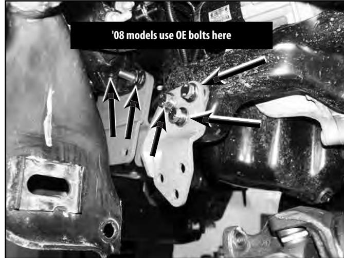
41. Using a jack (and an assistant to aid in balancing) raise the differential up to the new brackets.
