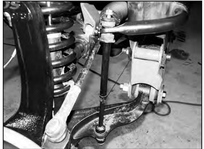
69. Reinstall front wheels. Torque to OE specifications, see owner's manual.
