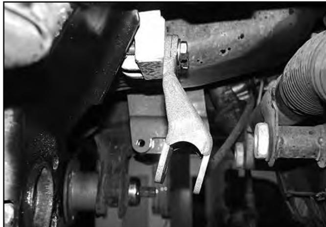
39. Install the two front driver's side differential drop brackets so that the bracket with the small offset (01236) is toward the outside of the vehicle (offsetting out) and the one with the bigger offset (01237) is on the inside (offsetting in). The brackets should taper down in height as they go toward the rear of the vehicle. Fasten the brackets to the frame with two  $\frac{1}{2}$ " x 2-1/2" bolts, nuts and  $\frac{1}{2}$ " SAE washers (BP #617). Leave hardware loose. (Fig. 11)
