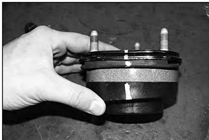
54. Reassemble the strut as it was taken apart by aligning the index marks made earlier. Fasten the assembly with the OE strut nut. Torque nut to 50 ft-lbs.
