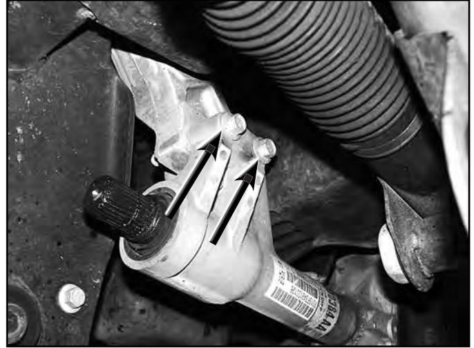
35. With the differential securely supported, remove the remaining bolts and lower the differential from the vehicle.
