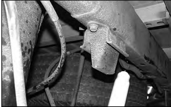
16. Attach the bump stop to the provided bump stop extension (01224) with 3/8" x 1-1/4" bolts, nuts and washers (BP #422). Torque hardware to 30 ft-lbs.
