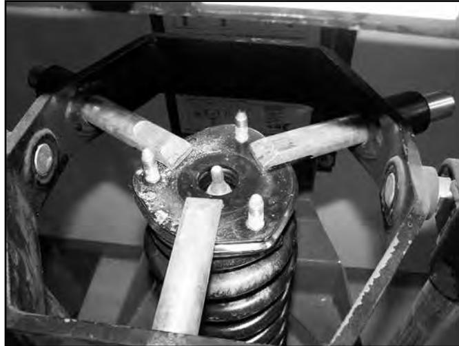
53. Place the provided preload spacer (01278) between the plastic coil seat and the rubber isolator (Fig 14d).
