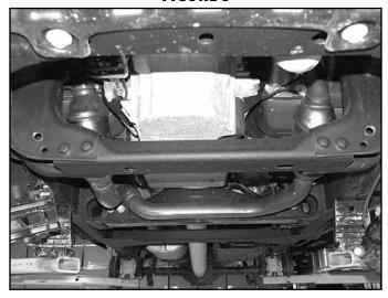
17. Install the new rear crossmember (02177) with the OE lower control arm bolts, nuts and washers. Also fasten the passenger's side of the crossmember to the two original crossmember mounting holes with the OE hardware (Fig 9). Leave hardware loose.
