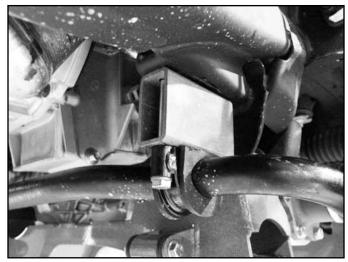
45. Attach the original sway bar links and hardware to the sway bar end and new hole in the lower control arm (Fig 22). Tighten the sway bar link until the bushings begin to swell.
