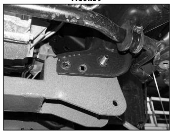
18. Install the front crossmember (02176) in the control arm pockets with the OE lower control arm bolts, nuts and washers (Fig 10). Also fasten the center of the crossmember to the frame using the two original front skid plate mounting holes and bolts. Leave hardware loose.
