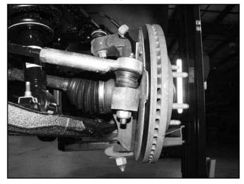
8. Remove the two brake caliper mount bolts and remove the caliper assembly from the knuckle (Fig 3). Hang the caliper securely out of the way. DO NOT hang the caliper by the brake hose.
