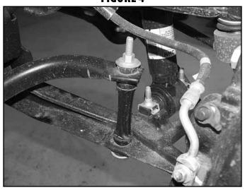
10. Remove the sway bar from the frame by removing the four bushing cap mounting bolts (Fig 5). Retain all sway bar components.
