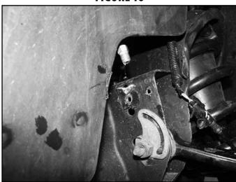
38. Attach the provided brake line bracket (02115-drv, 02116-pass) to the upper control arm mount using the original mounting hole/hardware and the newly drilled hole/provided 5/16" x 3/4" bolt, nut, flat washer and lock washer. (Fig 17) Leave hardware loose.
