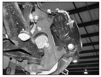
9. Remove the sway bar links from the sway bar and the lower control arm (Fig 4). Retain the links, bushings and hardware.
