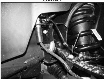
7. Disconnect the steering from the knuckle (Fig 2). Remove the tie rod end nut. Strike the knuckle near the tie rod end with a hammer to dislodge it. Retain the mounting nut.
