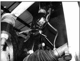
43. Locate the original sway bar link mounting hole on the lower control arm. Measure inward from the center on the hole 1-1/2" (toward the frame mount) and mark. Measure in from the back edge of the control near the first mark 3/4" and mark. Where the two marks cross drill a 5/8" hole (Fig 20).
