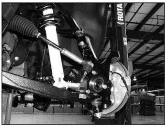
33. Working on one side at a time, remove the tie rod end from the steering link (Fig 15A). Trim 3/8" off of both the tie rod end and the steering link. (Fig 15B,C) This will allow for proper alignment adjustment once the kit is complete. Once the two pieces are trimmed, clean the ends of the threads and reinstall the tie rod end on the steering link. Repeat on other side of the vehicle.
