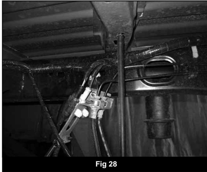
71. Attach the brake line to the relocation bracket with a ¼" nut and ¼" USS washer (BP #774). It may be necessary to rotate the OE brakeline clip bracket to have the lines face 'down' for adequate slack. Torque to 15 ft-lbs.
