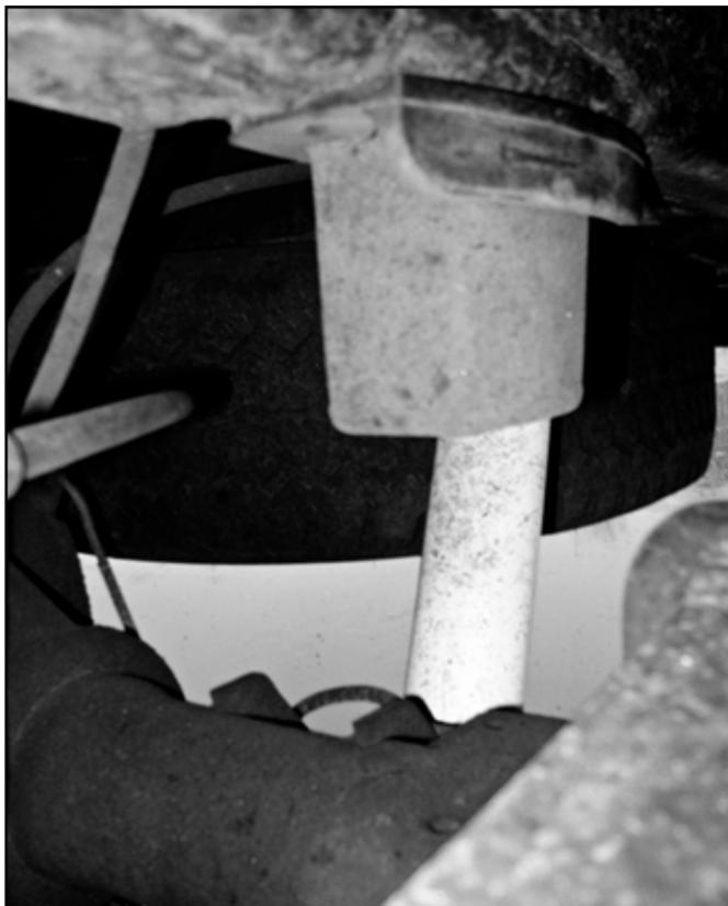
20. Install the factory bump stops on the new provided bump stop spacer (01196B) with the factory hardware. The bump stop will mount to the spacer on the face with 3 holes. Tighten hardware securely. (Fig 34)
