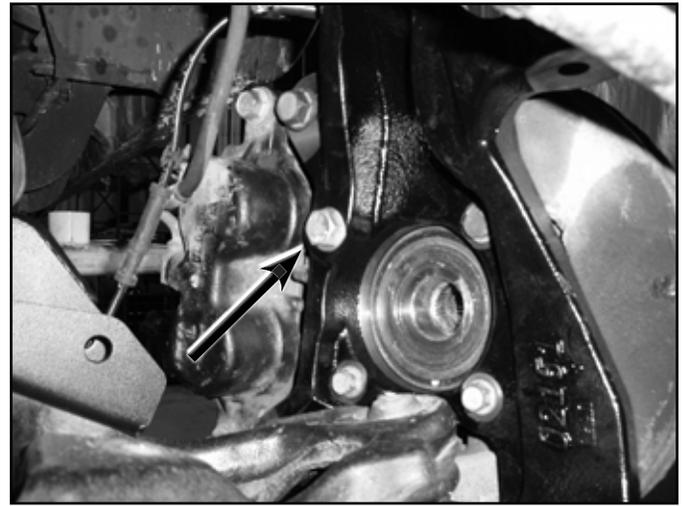
37. Install the brake rotor on the hub. Install the brake calipers on the knuckles with the original bolts. Apply Loctite to the bolt threads and torque the bolts to 125 ft-lbs. Be sure the brake hose is running under the upper control arm and behind the steering knuckle.
