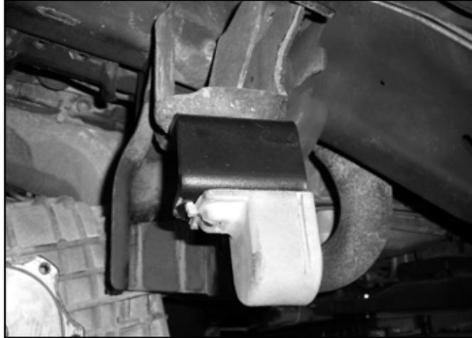
29. Install the factory lower control arms into the new crossmembers. Fasten the control arms with  $5/8"$  x  $5"$  bolts (front),  $5/8"$  x  $6"$  bolts (rear), nuts and  $5/8"$  SAE washers (BP 544). Run the front bolts front to rear, rear bolts rear to front (Fig 16), install spacer tubes. Leave hardware loose.
