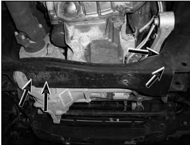
22. Inspect the inside factory control arm mounting holes. There will be a sharp lip left from the original control arm/hardware. Use a file or rotary grinder to remove the sharp lip left from the control arms (Fig 10). This will allow the new cross members to be installed easily.
