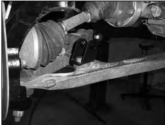
43. Locate the new front sway bar links (911109), small hourglass bushings (SB35BK) and 0.750" OD x 1.575" long sleeves (54587). Install the bushings and sleeves into the eyes of the links. Install the links into the new brackets on the lower control arms with 9/16" x 2-3/4" bolts, nuts and washers (BP 569). Run the bolts from front to rear and leave hardware loose (Fig 27). (4wd model shown - 2wd similar)
