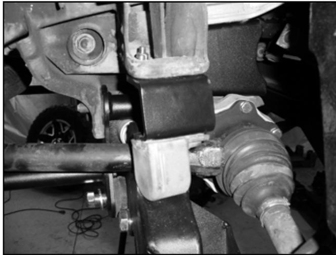
48. If installing optional front skid plate. Attach with factory splash guard hardware at the front frame crossmember. Use new 1/2" button head bolts (#571) to attach skid plate to the crossmember. Tighten to 35 ft-lbs.
