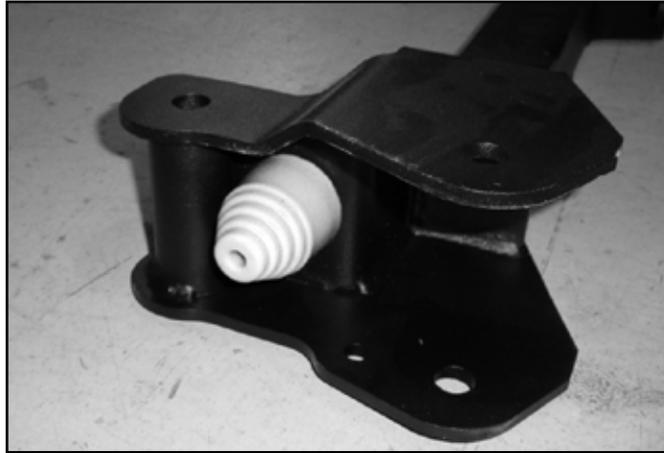
25. Install the rear crossmember in the rear lower control arm pockets, fasten the crossmember with the original lower control arm hardware. Run the bolts from front to rear. Leave hardware loose.
