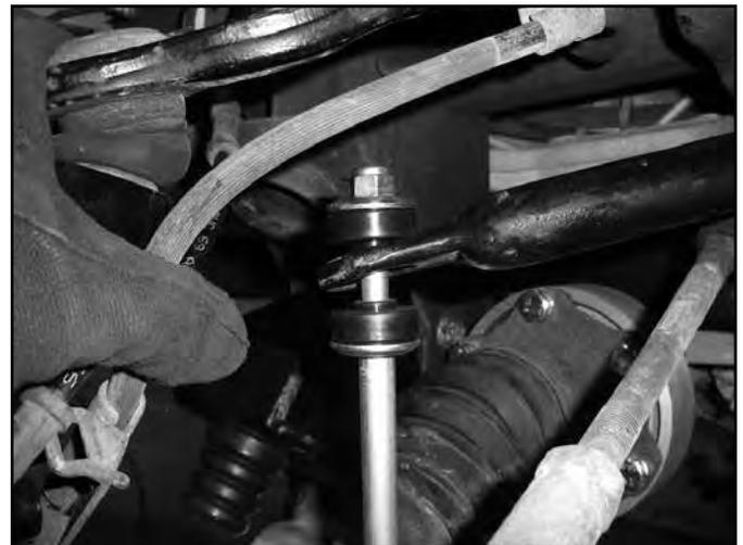
40. **Narrow Track Knuckle Kits Only:** Reconnect the original brake hose bracket to the upper control arm with the original bolt. Torque to 10 ft-lbs. Attach the second original brake hose bracket to the new "L" bracket install on the knuckle at the upper ball joint with a provided 1/4" x 3/4" bolt, nut and washers (BP 578). Torque to 10 ft-lbs.
