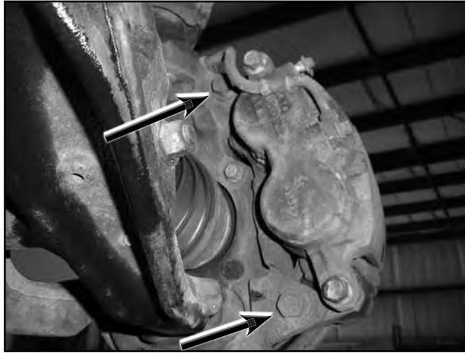
15. If equipped, remove the rotor retaining clips from the wheels studs. These will not be reused. Remove the brake rotor and set aside.
