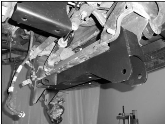
24. Install the new provided bump stops (M02096RB) on the new rear crossmember (02191) with 3/8" hex nuts, flat and lock washers (BP 544). Tighten hardware securely (Fig 12).
