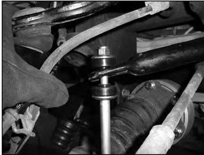
45. Attach the tie rod ends to the knuckles. Fasten with the original nuts and torque to 37 ft-lbs.
