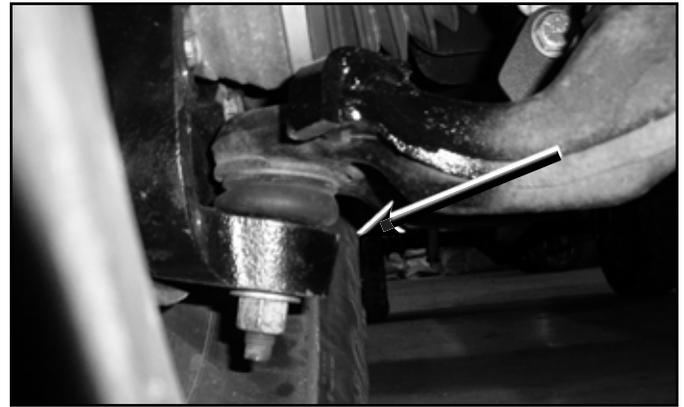
6. To determine the Z-height use the following equation:  $Y-X=Z$ . For the intended 7" of lift the value for Z should be approximately 4". If your value for 'Z' is less than 4" the torsion bars need to be adjusted up (tightened). If your value for 'Z' is more than 4" the torsion bars need to be adjusted down (loosened). These values are for reference but should not vary more than 1" in either direction.
