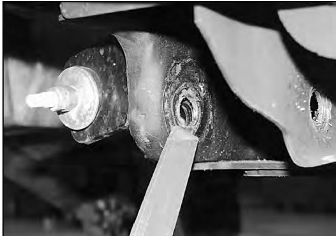
23. Locate the new front crossmember (02190). Install the crossmember in the front lower control arm pockets so that the two longer differential mounting tabs are on the driver's side pointing rearward (Fig 11). Fasten the crossmember with the original lower control arm hardware. Run the bolts from front to rear. Leave hardware loose.
