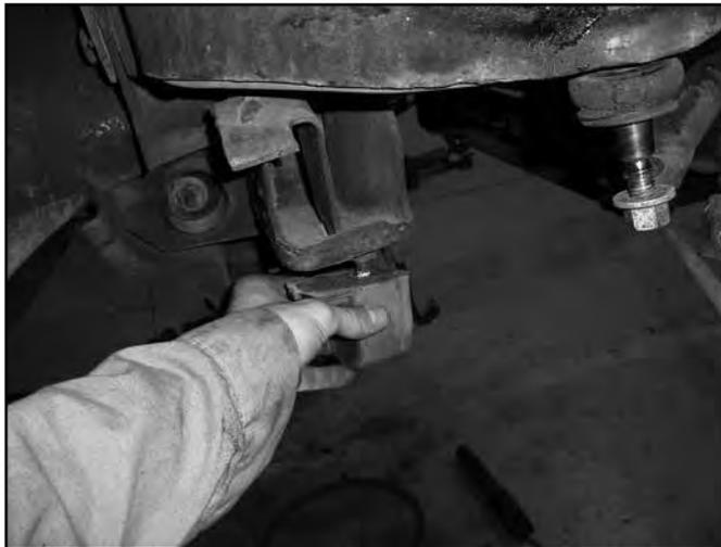
21. Remove the four bolts mounting the rear crossmember to the rear lower control arm pockets (Fig 9). Remove the crossmember from the vehicle. The crossmember and hardware will not be reused, 4WD model shown, 2WD similar.
