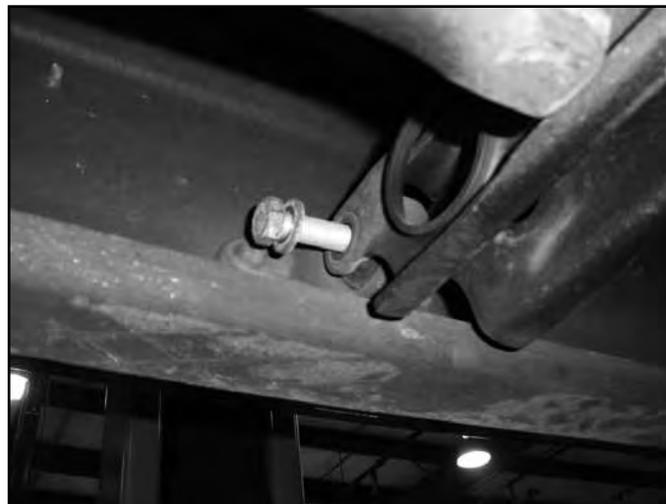
8. Remove the torsion bars by pulling them rearward out of the lower control arms. Set the torsion bars aside.
