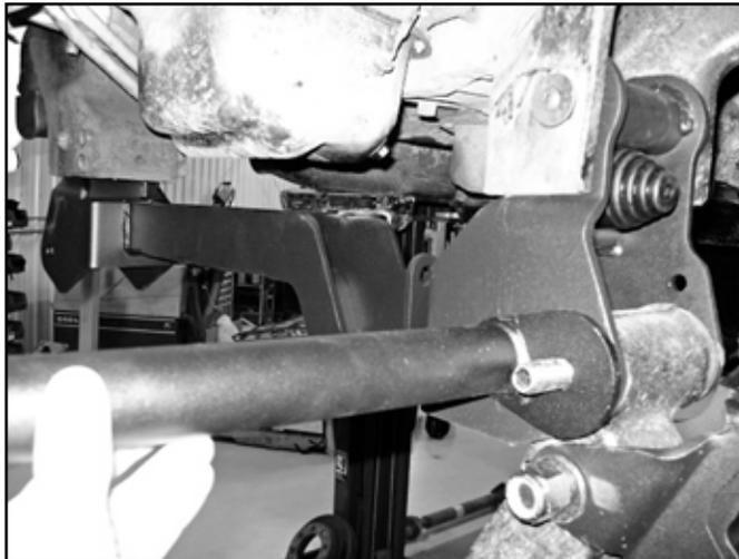
30. Located the factory shock mount bolted to the lower control arm. Remove the shock mount by removing the two mounting bolts. These bolts are held in place with thread locker so take care not to break the bolts with excessive force when removing. Save the bolts and discard the bracket.
