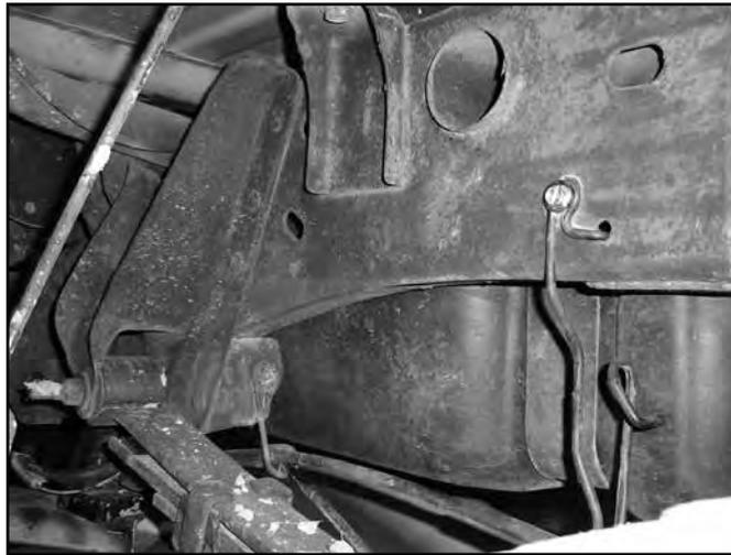
4. Disconnect the factory brake line bracket attached driver's side frame rail. The nut is accessed on the outside of the frame (Fig 31).
