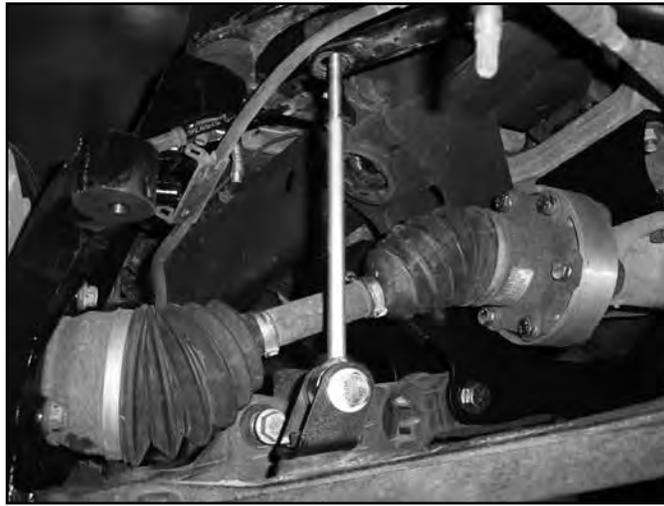
44. Install a provided stem washer (S100776) followed by a stem bushing (SB26BK) on each sway bar link. Install both links into the sway bar and install a second stem bushing followed by a second washer. Fasten the sway bar link upper assemblies with 3/8" nylock nuts (BP 569). Leave nuts loose (Fig 28).
