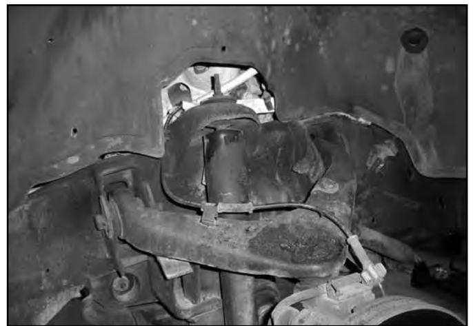
14. Remove the two bolts mounting the brake caliper assembly to the steering knuckle and hang the caliper out of the way (Fig 7). Do not hang the caliper by the brake hose. Save mounting bolts.
