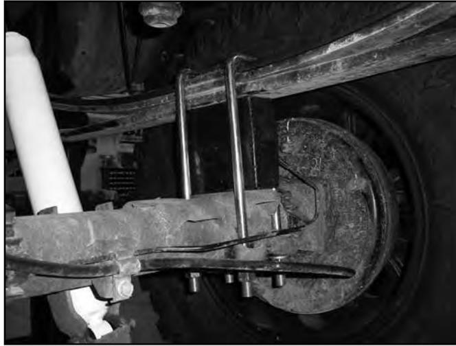
9. Repeat the installation on the driver's side of the vehicle. Pay special attention to all of the brake lines and wires. Do not allow them to get over-extended.
