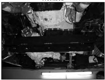
40. With the rear crossmember installed, fasten the factory rear differential mount to the outer crossmember mount with a 9/16" x 2-1/2" bolt, nut and washers (BP 647). Also, install the factory flanged high nut on the captive stud, which is accessed through the bottom of the rear crossmember (Fig 33). Leave hardware loose.
