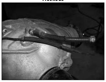
36. With the help of an assistant and an appropriate jack, raise the differential up to the new front crossmember. Align the holes in the factory differential mount brackets with the corresponding holes in the crossmember. Loosely fasten the differential (Fig 29) to the front crossmember with 9/16" x 3-1/2" bolts, nuts and washers along with the large lower factory washer. (BP 647).
