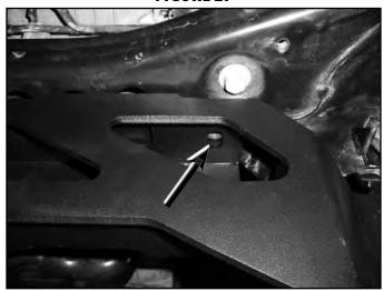
35. Locate and replace the factory vacuum and breather lines on the top of the differential (Fig 28). Transfer the hose clamps from the factory breather hose to the new provided one. The vacuum line does not have clamps and just slides onto the hard line.
