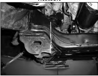
28. On the passenger side, measure in and mark 3" from the inside edge of the control arm pocket (Fig 22). Extend the line along the bottom of the crossmember (parallel to the inside edge of the control arm pocket) and up the front and back faces of the crossmember.
