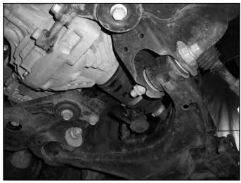
20. Disconnect the lower strut mounting bolt and remove from the lower control arm (Fig 16). Allow the lower control arm to swing down. Save the strut mount hardware.
