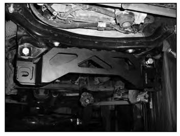
34. 4wd models only, 2wd skip to # 39. Locate the top holes inside the front crossmember that line up with the original differential mount holes in the frame (Fig 27). There will be a gap between the top of the crossmember and the bottom of the frame. Insert a provided 5/8" USS washer (BP 647) between the frame and crossmember at each (2) mount hole. Install provided 9/16" x 3-1/2" bolts, nuts and washers (BP 647) up through the crossmember, spacer washer and frame. Leave hardware loose.
