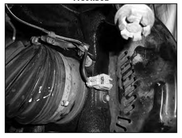
75. Attach the ABS wire bracket to the backside of the knuckle in the provided tapped hole with the original bolt (Fig 53). On the driver's side it will be necessary to remove the extra tab on the bracket to mount it properly (Fig 54). The ABS line can be slid in the plastic retainer clips that attach to the metal brackets to adjust the line for proper slack. Lubricate the line with spray lubricant and pull through the plastic clips as necessary. Torque bracket bolt to 8 ft-lbs.
