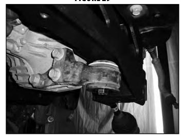
37. Locate the factory rear differential mount that was removed earlier. Locate the bottom outer mount surface and the cast ribs that extend close to the mounting hole. These ribs need to be ground down flush to the mounting surface back into the mount body about 1/4" to provided clearance with the new differential mount (Fig 30). This can easily be done with a standard angle grinder.
