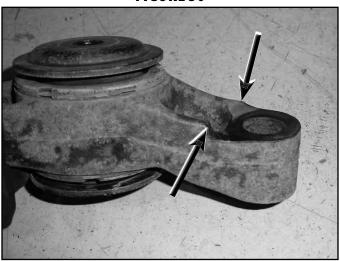
38. Loosely install the modified factory rear differential mount to the differential with the original bolt (Fig 31). The mount should be positioned as it was when removed with the captive stud to the inside and pointing down. Leave the bolt loose so the bracket can move freely.
