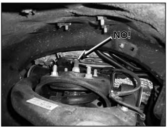
23. Steps 23-31 are for 4wd vehicles only, 2wd models skip to step# 32. Locate the front differential actuator wire connector on the front passenger's side of the differential. Push in on the retaining clip and pull the connector free from the actuator (Fig 18).
