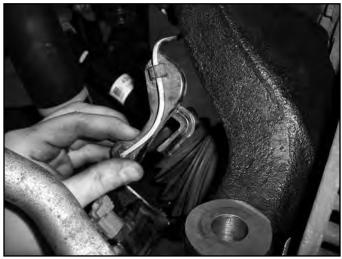
76. Locate the new brake line relocation brackets (01655). Attach the brackets to the original frame mount with the original bolt. The stud on the bracket will point out and the bracket will angle in toward the strut about 20-30 degrees from vertical (Fig 55). Torque bolt to 10 ft-lbs.
