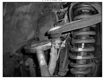
18. Disconnect the steering knuckle from the lower ball joint mount. Remove the two bolts (Fig 14) and remove the knuckle from the vehicle. Save bolts and knuckle.
