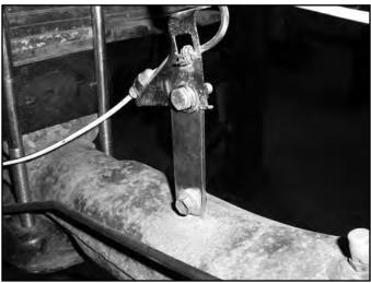
13. Locate the provided brake line relocation bracket (01661 - 1" hole-to-hole), provided 1/4" hardware and wire clip (BP 651). Install the wire clip on the ABS wire where the factory plastic clip was removed (Fig 65A, B). Remove the 1/4" x 1" bolt w/washer through the clip, into the new relocation bracket and into the front of the original ABS mount tab on the top of the differential. Fasten with a 1/4" nut and washer. Position the relocation bracket vertical and torque bolt to 8-10 ft-lbs.
