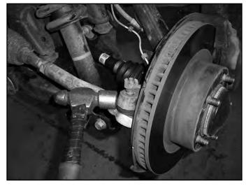
7. Disconnect the sway bar links from the lower control arms and sway bar (Fig 4). Remove the links from the vehicle. Save the lower mount bolts and discard the rest.
