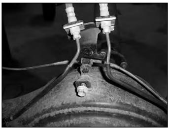
6. Disconnect the ABS line bracket from the driver's side of the axle (Fig 62A). Save hardware. For 7" lifts, carefully bend the factory ABS line bracket down at the charcoal canister located on the frame (Fig 62B, C).
