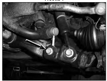
8. Disconnect the brake line brackets (Fig 5A, B) from the steering knuckles (2 per knuckle). Save hardware.
