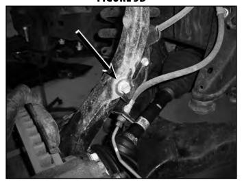
9. Disconnect the brake line bracket from the frame (Fig 6). Save bolt. Remove the ABS line from the retaining bracket on the upper control arm. Remove the retaining bracket on the upper control arm and discard the bracket it will not be reused.
