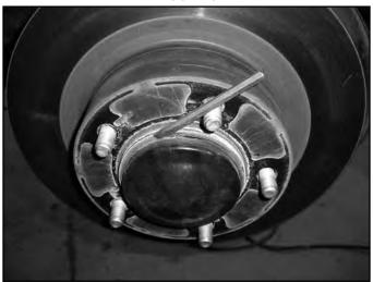
14. Remove the cotter pin and castellated nut cap from the end of the axle shaft. Remove the axle nut from the axle. Save the axle nut and cap (Fig 10). Discard the cotter pin (new one provided).
