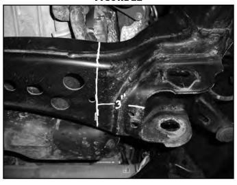
29. Using a reciprocating saw (highly recommended), hack saw or cut-off wheel, cut the rear crossmember out of the vehicle along the driver's and passenger's side cut lines (Fig 23).
