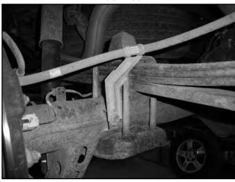
5. Disconnect the rear brake lines from the (3) mounting points at the center of the axle (Fig 60). Save hardware and leave the factory clamps on the hard lines. Disconnect the plastic ABS line clip from the top of the differential (Fig 61). Remove the plastic clip from the ABS line, it will not be reused.
