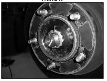
15. Unseat the axle shaft from the knuckle. Use an air hammer with blunt nose punch (recommended) or a hammer and punch, unseat the axle from the hub (Fig 11). A large rubber mallet can be used also, but make sure to thread the axle nut on flush with the end of the axle to protect the threads.
