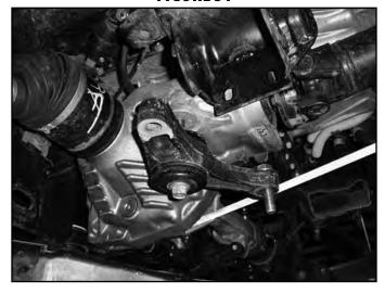
39. Install the new rear crossmember (02203) in the rear lower control arm pockets (Fig 32). When installing the crossmember, align the captive stud on the rear differential bracket with the mounting hole in the crossmember. Fasten the crossmember to the frame with 18mm x 170mm bolts (BP 650) and (2) rectangle cam washers (02212). Run the bolts from rear to front. Install the remaining (2) cam washers on the bolt but do not install the nut.
