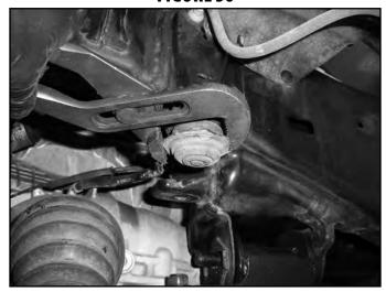
49. Locate the provided bump stop mounts (02216 - drv, 02217 - pass) and new bump stops (M03138BK). The new mounts are side specific. The large tab will mount to the rear crossmember bolt and the small slotted hole mounts to the frame. Install the provided bump stops (Fig 37A) to the new mounts with a 3/8" flanged nut (BP 649). Tighten nut securely (do not overtighten, causing the bump stop to deform).
