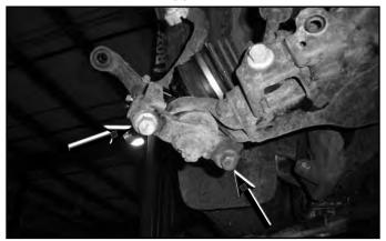
19. Loosen but do not remove the lower control arm cam bolts. On the front, loosen the bolt from the front. On the rear, loosen the nut from the front (Fig 15).
