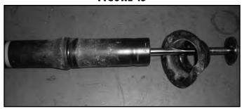
59. Install the proper preload ring on the strut. For Bilstein Struts, the preload ring will seat over the strut snap ring and the preload ring OD will step down to fit inside the coil seat (Fig 44A). For Standard Struts, the top edge of the preload ring tapers in to fit inside the coil seat (Fig 44B).
