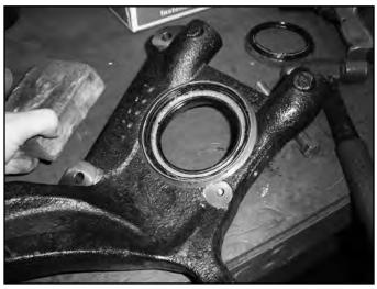
68. Install the new steering knuckles on the appropriate side of the vehicle. Run the CV shaft through the knuckle hub bore and fasten the knuckles to the lower ball joint mount with the original mounting bolts (Fig 50). Use Loctite on the bolts and torque to 175 ft-lbs.
