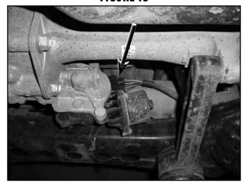
24. Locate the differential vacuum and breather lines on the upper driver's side of the differential (Fig 19). Disconnect the lines from the hard lines at the frame.
