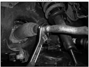
6. Remove the tie rod end cotter pin. Remove the nut from the tie rod end and thread back on a couple of turns. Strike the steering knuckle near the tie rod end to dislodge the taper (Fig 3). Remove the nut and the tie rod end from the knuckle. Save the nut and discard the cotter pin.
