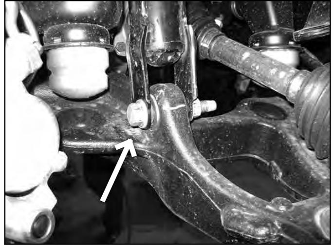
23. Remove the front and rear lower control arm bolts and remove the control arms from the vehicle (Fig 14) Save the control arms and mounting hardware.
