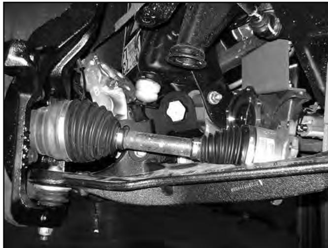
59. Install the original CV axle nut and washer and torque to 155 ft-lbs. Reinstall the hub dust cap.
