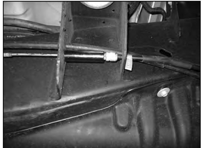
23. Thread on a M6 jam nut and the coupler nut to the e-brake cable (BP 588). Adjust the coupler nut depth to have half of the threads engaged. (Fig R11)
