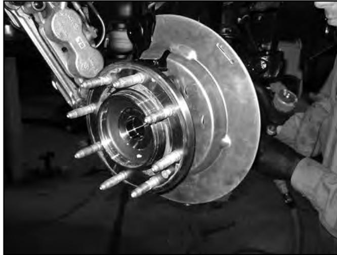
55. Run the ABS line around the front of the steering knuckle and up to the wire connector on the frame. Reconnect the wire and reattach it to the original place on the frame.
