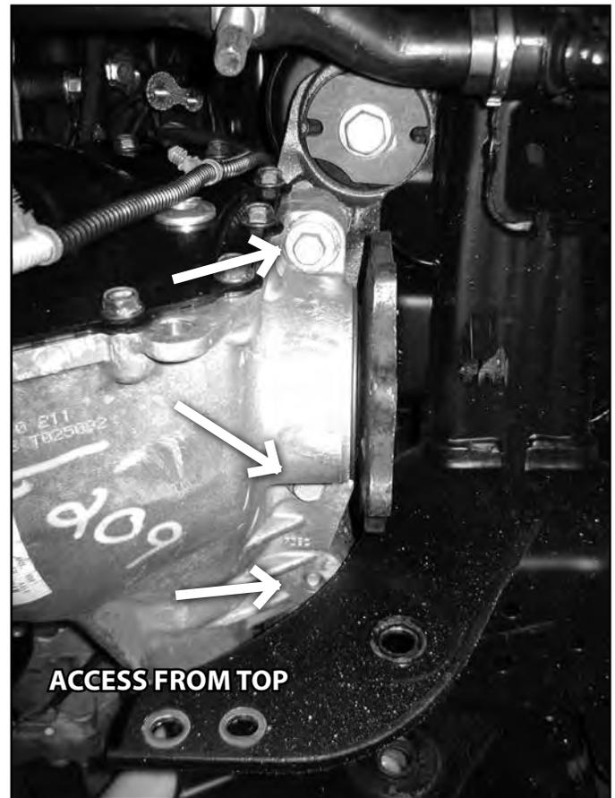
30. Support the front differential with an appropriate jack. Remove the differential mounting hardware and lower the differential from the vehicle and set aside. Save hardware.
