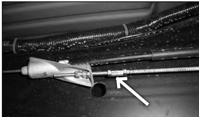
26. Reinstall the E-brake cable bracket near the jounce bumper with factory hardware.
