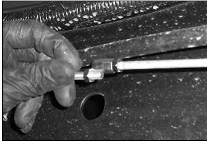
24. Attach the M6 threaded extension (SBTE) with jam nut and tighten securely.
