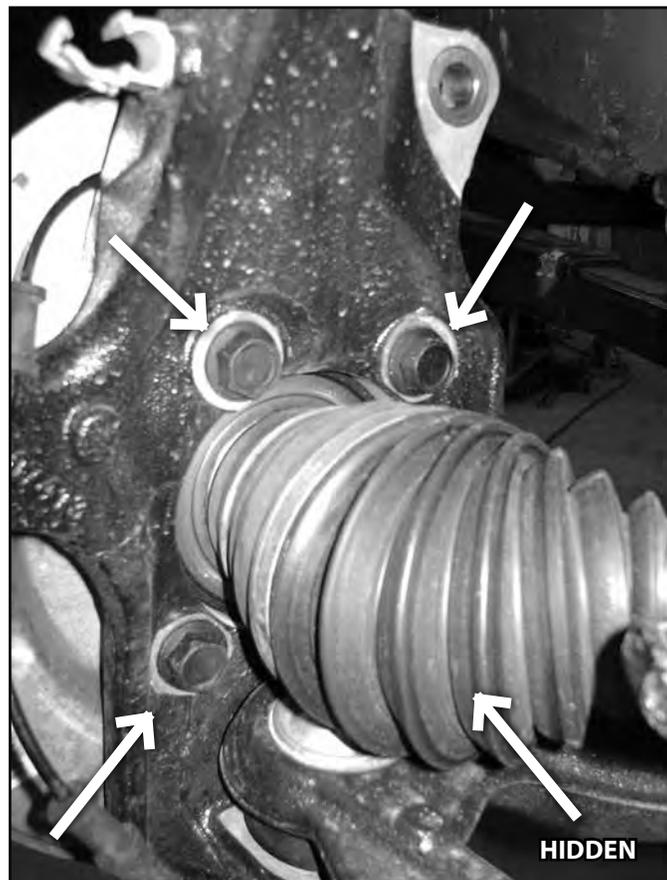
20. Remove the upper and lower ball joint nuts (Fig 11). Reinstall the nuts a couple of turns by hand. Strike the knuckle near the ball joints to release the taper. Remove the nuts and remove the steering knuckle from the vehicle. Save nuts. Take care not to strike the ball joint.
