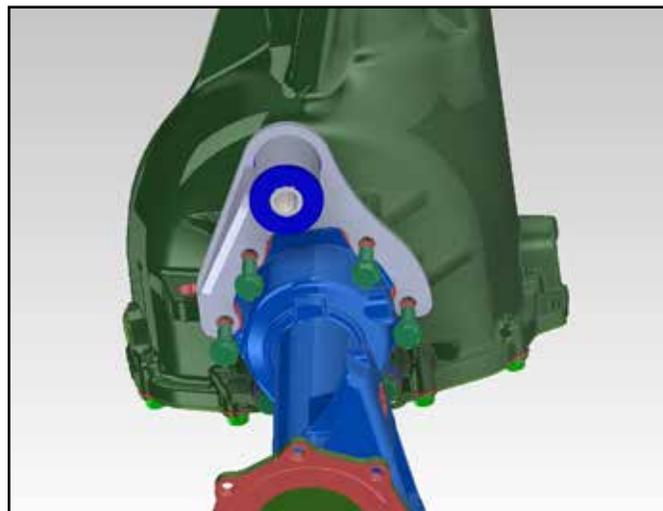
35. Locate the new passenger's side differential bracket (02371). Bracket has a single center gusset. Install the bracket on the existing studs on the passenger's side factory bracket. Fasten with the original nuts and washers. When installed the open side of the bracket will face inward and the bracket will taper down as it goes to the rear (Fig 22). Torque nuts to 65 ft-lbs.
