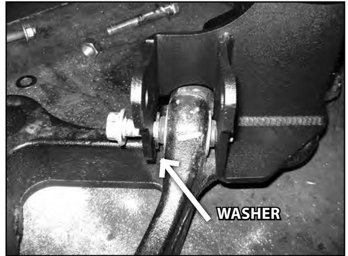
45. With both new torsion bar bracket installed on the factory control arms, install the control arms in the crossmembers. Fasten the control arms with the provided 18mm x 120mm (front) and 18mm x 140mm bolts, nuts and 3/4" SAE flat washers (BP 585). Run the front bolts front-to-rear and the rear bolts rear-to-front. (Fig 27) Leave hardware loose. These bolts will be torque with the weight of the vehicle on the suspension.
