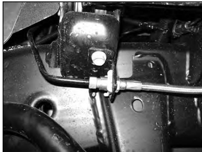
66. There are two threaded holes near the top of the steering knuckle neck on the back side. Using a provided wire clamp, 1/4" x 3/4" bolt and 1/4" lock washer (BP 590) loosely fasten the brake line to the lower threaded hole on the steering knuckle. Using the same fastener combination, attach the ABS line to the upper threaded hole. The hardware will be tightened once the line slack is set. (Fig 36A).
