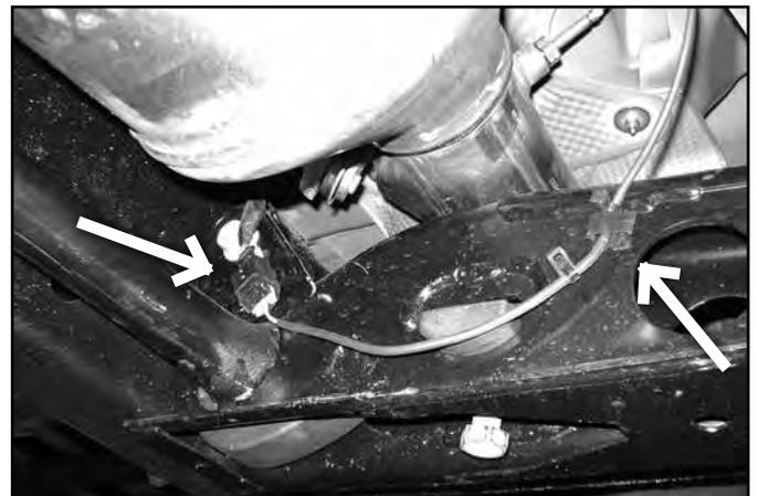
9. Remove the torsion bars by pulling them rearward out of the lower control arms. Set the torsion bars aside.
