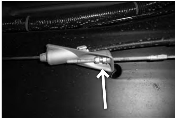
7. Disconnect the E-brake cable bracket from the frame near the rear jounce bumper. Save hardware, it will be reinstalled later. (Fig R3)
