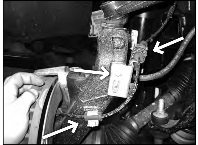
15. Remove the two bolts mounting the brake caliper assembly to the steering knuckle and hang the caliper out of the way (Fig 7). Do not hang the caliper by the brake hose. Save mounting bolts.
