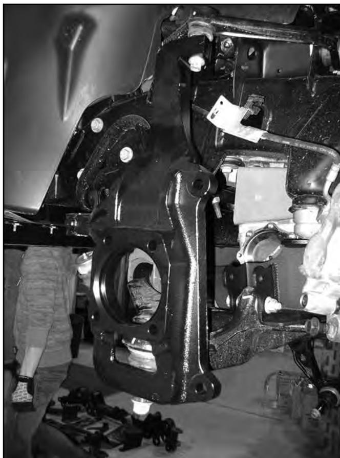
52. Locate the hub o-ring in the factory steering knuckle hub bores. Carefully remove the o-rings (Fig 30) and install into the new steering knuckles.
