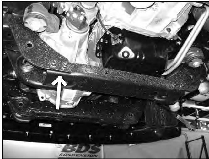
27. Disconnect the electrical connector from the front differential actuator (Fig 17A) Remove the wire from the three plastic wire retainers along the top of the differential.
