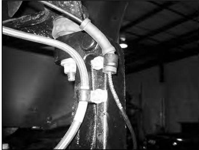
67. On the front side of the steering knuckle there is a small threaded hole. Using a third wire clamp, fasten the ABS wire to the front face of the knuckle with a 1/4" x 1/2" self-tapping bolt (BP 590). Tighten securely. (Fig 36B) Adjust the slack in the two other lines, rotating the steering knuckle back and forth as a check, and tighten the upper two clamps to 10 ft-lbs.
