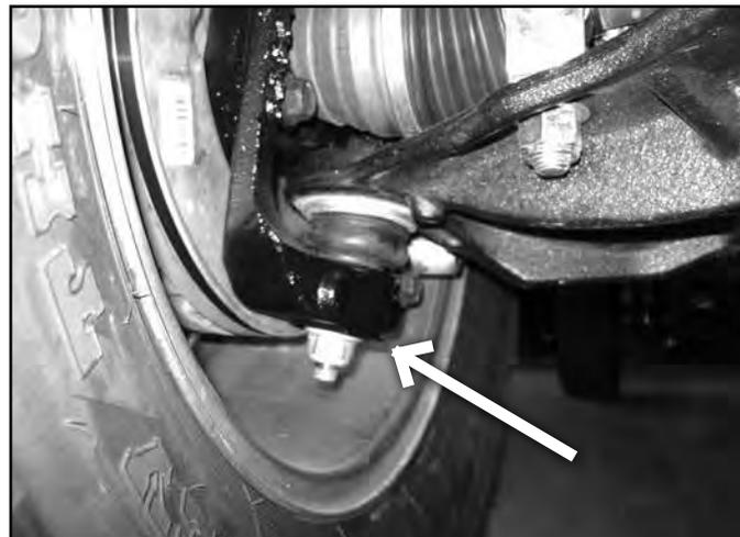
4. Roll the vehicle forward and back to settle the front suspension. With the vehicle on flat, level ground measure the distance from the floor to the center of the front lower control arm bolt. This is distance 'Y'.
