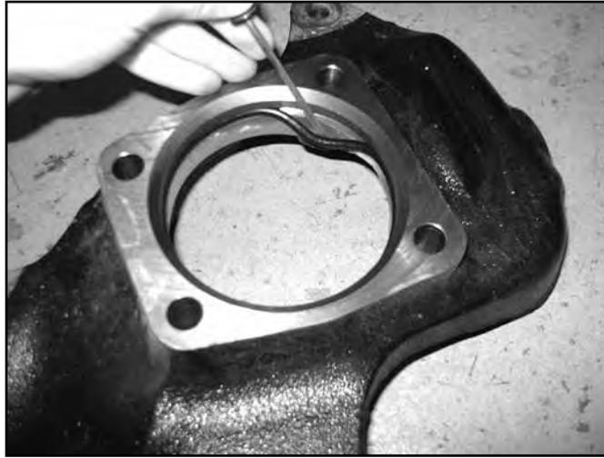
53. Locate the factory driver's and passenger's brake dust shields. They need to be modified to provide adequate brake caliper clearance. Make a cut line by following the straight edge on the caliper side of the shield all the way to the bottom edge of the shield. (Fig 31) Cut the shield along the line.
