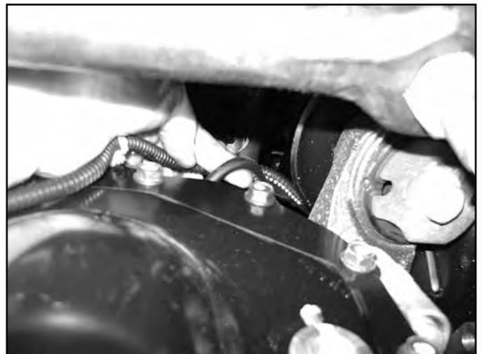
29. Loosen but do not remove all of the front differential mounting bolts/nuts. There are two nuts on the passenger's side (Fig 18A) and three bolts on the driver's side (Fig 18B - two mount from the bottom up and one from the top down). Remove the rear-most bolt mounting from the top.
