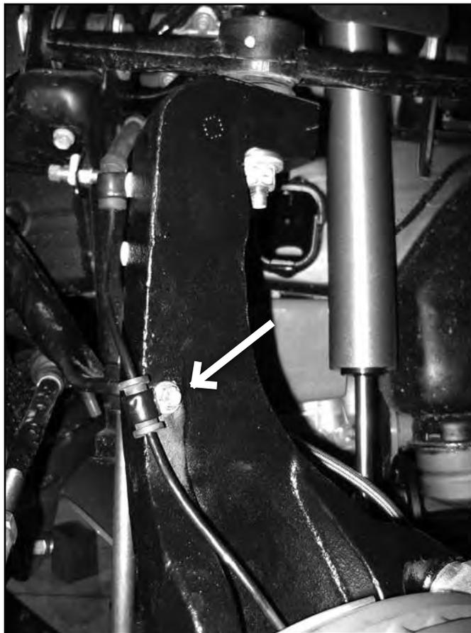
68. Locate the new front sway bar links (911109), hourglass bushings (SB58RB) and 0.625" x 1.375" steel sleeves (45313). Lightly grease and install the bushings and sleeves into the sway bar link ends.
