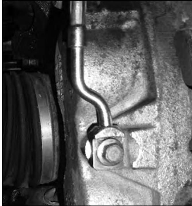
64. Remove the factory brake line from the caliper. Be sure to remove the factory crush washers as well. Place a new provided crush washer on each face of the new brake line and install on the caliper with the factory banjo bolt. Torque the bolt to 20 ft-lbs.
