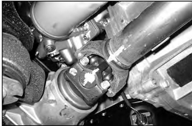
26. Remove the four bolts mounting the rear crossmember to the rear lower control arm pockets (Fig 16). Remove the crossmember from the vehicle. The crossmember and hardware will not be reused.
