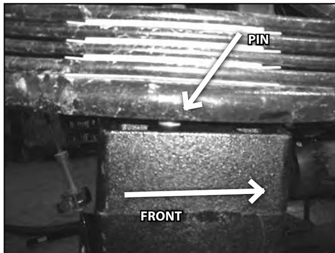
15. Attach axle to springs with new u-bolts (5/8" x 4" x 16"). Run the u-bolts from bottom up and through the new u-bolt plate. Snug the hardware at this time, but do not torque to specification.
