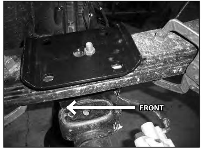
13. 3" & 5" Overload options: The Models equipped with overload leaves will need the separation block modified. Trim the anti-rotation tabs from the front side of block on both the inside and outside of the block. Use extreme care near the fuel tank, do not use any method that will create sparks if the block is not removed when modified. A sawzall is highly recommended. (Fig R6)
