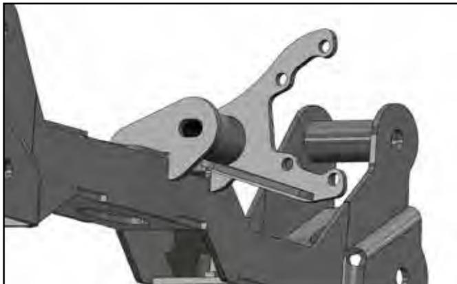
39. With the differential and rear crossmember installed, tighten all the differential mount hardware. Torque the (4) 1/2" bolts to 65 ft-lbs and (1) 9/16" bolt to 95 ft-lbs.
