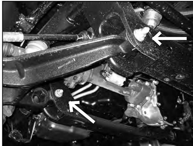
24. There are two factory bump stops per side. Remove the front rubber bumpstop from the frame mounts on each side. They can be removed with a pair of channel-lock pliers.
