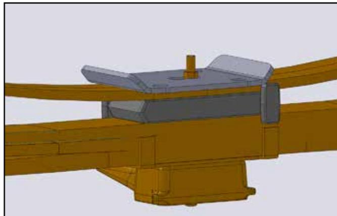
14. Lower the axle to allow the lift block (5FB18) to be installed. The leaf spring pin will go in the REAR hole of the block. (Fig R7)
