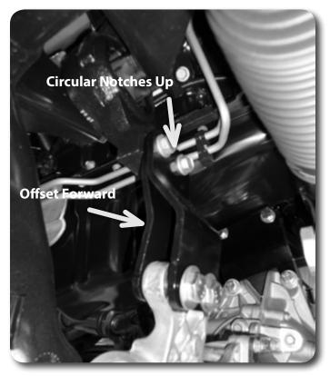
34. Install the two front driver's side differential drop brackets so that the bracket with the small offset towards the driver's side and the one with the bigger offset is towards the passenger's side. The brackets should drop more at the front of the vehicle. Fasten the brackets to the frame with two 12mm x 40mm bolts, nuts and washers. Leave hardware loose. Figure 13
