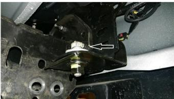
2. Remove the tow hook along with foam shield.
