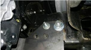
6. Reinstall the tow hooks. Use the factory tow hooks. If there are no tow hooks present, use  $\frac{1}{2}$ " bolts. Also, at this time tighten the 18mm bolt that was loosened in step 1.
