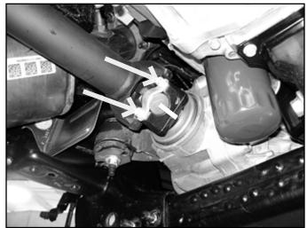
22. The driver's side rear lower control arm pocket must be cut to provide clearance for the front differential in the relocated position. This also aids in the removal of the differential. This area needs to be cleaned of any oil, grease and/or undercoating. These coatings are flammable.
