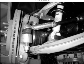
7. Remove the two brake caliper mounting bolts and remove the caliper from the knuckle (Fig. 4). Hang the caliper securely out of the way DO NOT hang the caliper by the brake hose. Save caliper bolts.
