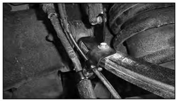
69. Reconnect ABS line at the frame. Attach the ABS line to the steering knuckle with the provided wire clamps and ¼" x ¾" self tapping bolt and flat washer. Torque bolt to 15 ft-lbs. Use zip ties to retain the remaining section of the ABS line as needed to keep it away from rotating objects. (Fig. 36)
