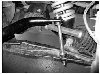
72. Connect the steering tie rod ends to the knuckles with the short provided nylock nuts. Ensure the nut has full thread engagement. Torque to 60 ft-lbs. Tighten the tie rod end jam nuts securely. They will be adjusted during alignment. Install the zerk fittings into the tie rod ends.
