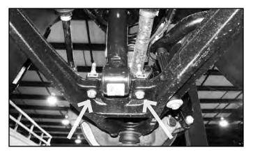
14. Remove the CV shaft mounting flange bolts (6 per side) (Fig. 9). Mark the shaft to indicate driver's or passenger's side. Bolts will not be reused.
