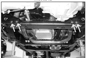
21. Make an alignment mark to show the relationship between the front driveshaft and the differential yoke. Remove the four driveshaft bolts and disconnect the driveshaft from the differential. Save bolts. (Fig. 13)
