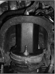
52. Install the strut assembly to the appropriate frame mount with the original nuts. Leave hardware loose. Make sure there is enough slack on the MagneRide wire harness.
