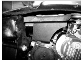
39. Install the differential to the new driver's and passenger's differential brackets. Fasten the differential to the driver side bracket with  $\frac{1}{2}$ " x 1-3/4" bolts, nuts and washers. Use the 5/8" bolt, 5/8" SAE washer and one extra thick 5/8" washer on the passenger's side. The extra large washer will go against the differential housing flange with the large slots. Leave hardware loose.
