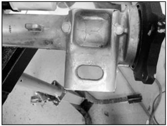
32. The lower tab of the differential will need to be trimmed to clear the high clearance skid plates as shown in Figures 22A, B.
