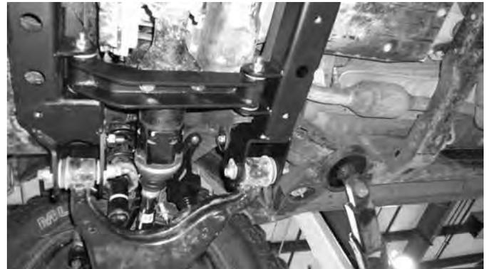
35. Reinstall the factory differential mount (Driver's side rear) with the factory bolts. Leave slightly loose.
