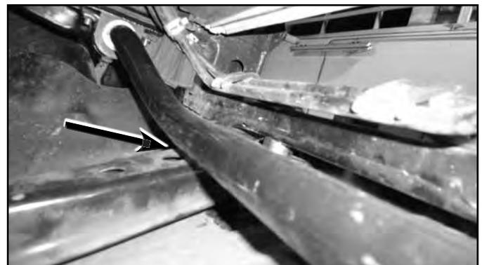
31. Install the factory skid plate back on with factory hardware.
