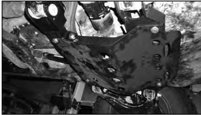
67. Center the front cross member cam. Adjust the rear cam to be 'out' slightly (approx 45 degrees). Snug but do not torque the hardware at this time.
