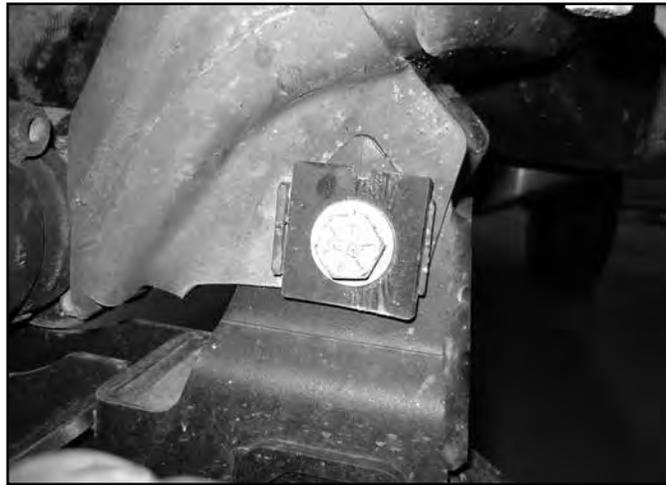
25. Mark the factory crossmember at the center of the slots on the back side of the BDS rear crossmember. Temporarily remove the BDS rear crossmember to drill 11/16" holes at the marks in the factory crossmember. A step drill is highly recommended. (Fig 15b & c)
