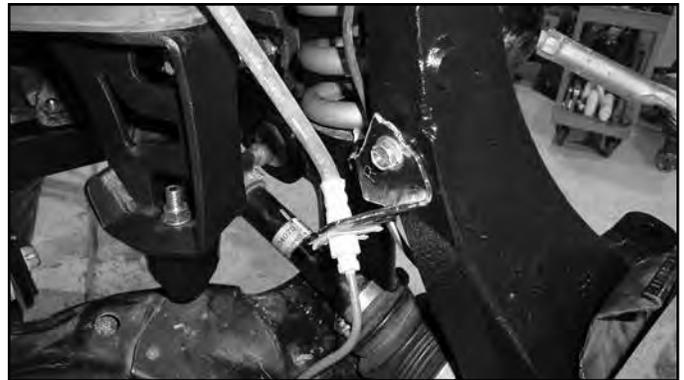
59. Attach the brake line bracket to side of the steering knuckle with factory bolt.
