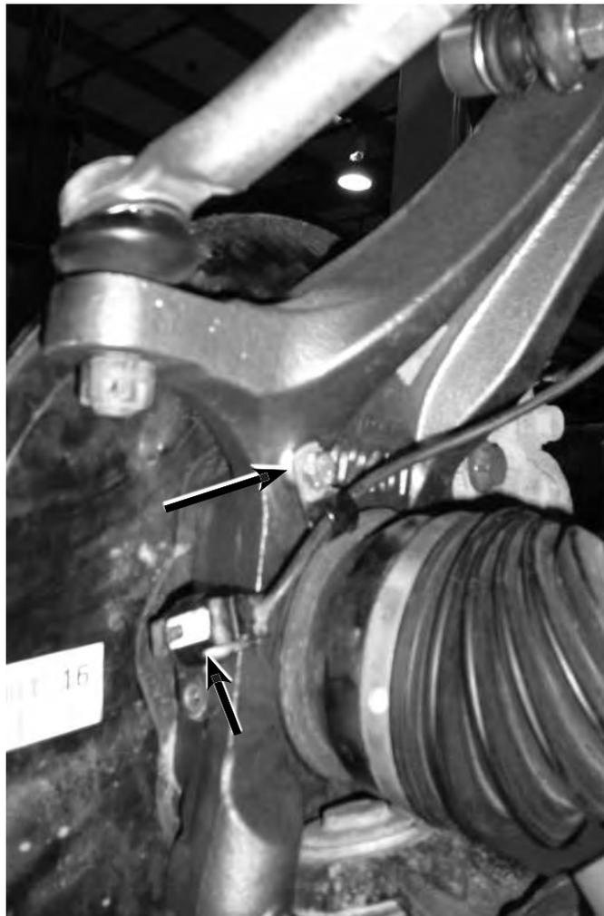
62. Attach the ABS sensor to the steering knuckle with the factory bolt. Make sure there is no debris on the sensor before it is installed. Tighten to 73 in-lbs.
