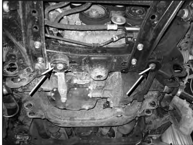
21. Measure  $\frac{1}{4}$ " inside of the factory weld seam (or about 3-1/4" from the inside edge of the cam slot) and make a cut line all around the factory crossmember. Make a vertical cut. (Fig 14a, 14b, 14c)
