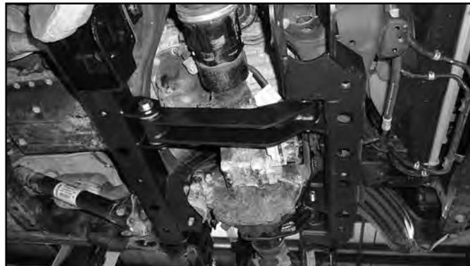
39. Remove the differential breather tube assembly from the vehicle and bend upward to clear the steering shaft. Reinstall with factory hardware. Tighten to 15 ft-lbs. (Fig 21a & 21b)
