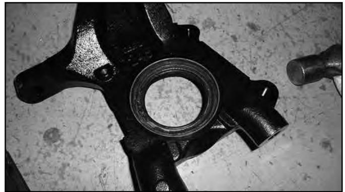
50. Remove the factory unit bearing and dust shield from the OE steering knuckle. The bolts will not be able to be completely removed from the hub, thread them out enough to disengage them from the steering knuckle.
