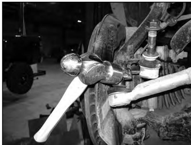
11. Remove the lower ball joint to steering knuckle mounting hardware. It will not be reused. Remove the steering knuckle assembly from the vehicle. It may be necessary to use a punch and hammer to dislodge the CV from the hub.
