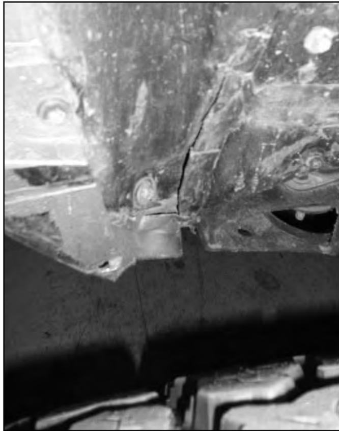
90. Trim the body mount as shown: Measure in 5" from the outside edge, measure over 1" from the center of the circle, trim and remove section from the body mount. (Fig 40a 40b)
