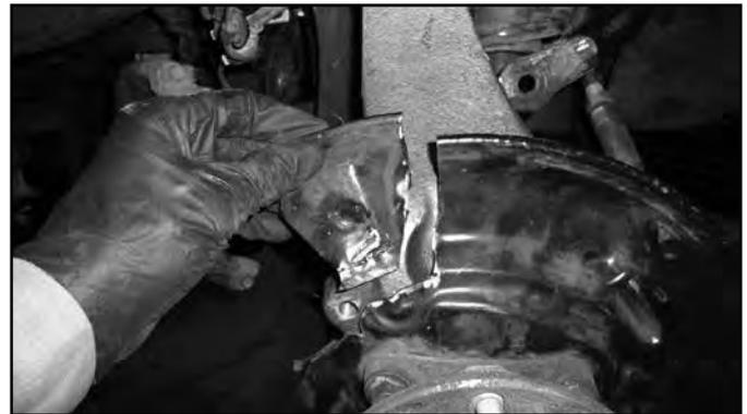
52. Install the hub and dust shield into the new steering knuckles. The dust shield must be installed. Failure to do so will damage the ABS sensor. Use loc-tite on the hub bolt threads. Tighten to 60 ft-lbs
