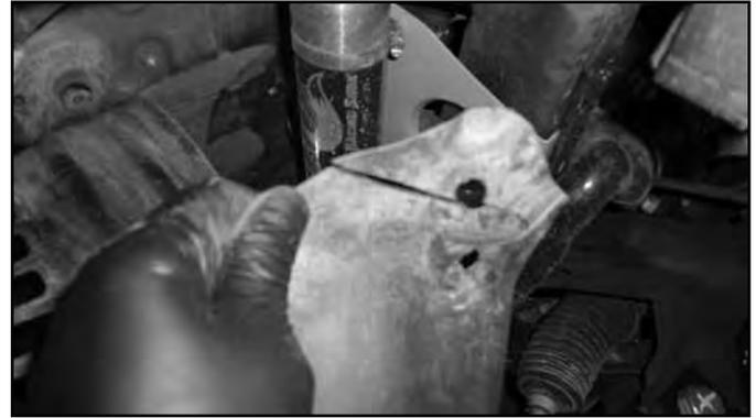
92. Reattach the inner fender to the front fascia with factory bolt through the new hole. This will pull the front inner fender away from the tire.
