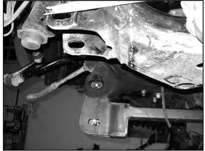
22. Measure over 7-1/4" from the first cut line and make another mark around the entire cross member. This should be on the center of the large circles. Make a vertical cut and remove the section from the vehicle. (Fig 14d, 14e)
