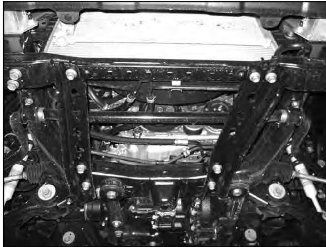
5. Disconnect the brake line bracket from the steering knuckle and disconnect ABS wire from the bracket. Disconnect the brake calipers from the knuckle. Hang the caliper out of the way. Do not allow the caliper to hang from the brake line. Keep all hardware. (Fig 3)
