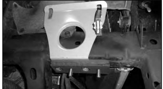
28. Disconnect the sway bar link from the sway bar. Cut out the template at the end of the instruction sheet. Place over the end of the sway bar. Trim / grind away approximately 1/4" of material to give enough clearance between the sway bar and new steering knuckle. (Fig 17a, 17b)
