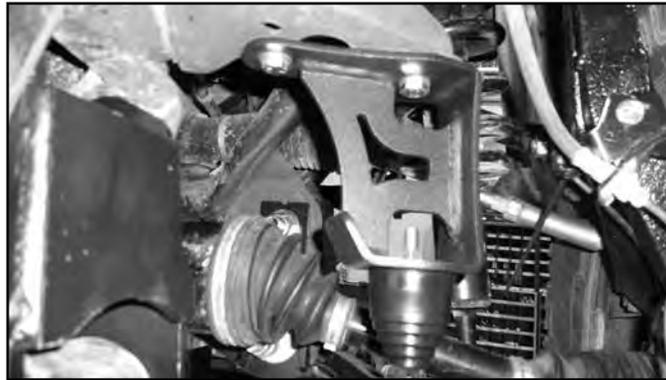
42. Attach the driveshaft to the front differential with factory hardware. Tighten to 65 ft-lbs.
