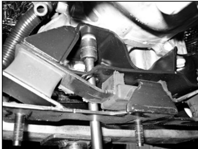
10. Manual shift transfer cases: Disconnect the shift linkage from the transfer case, retain all hardware.
