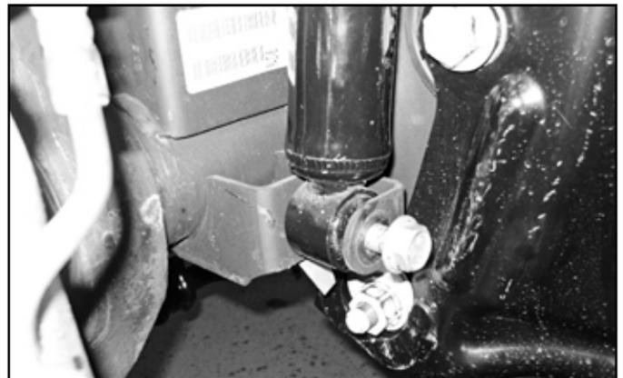
13. Raise the front axle and reattach factory shocks with factory bolt. It is not necessary to put the nut tab back on. The shocks will be there to keep the axle secure. Keep a jack under the axle for extra support.
