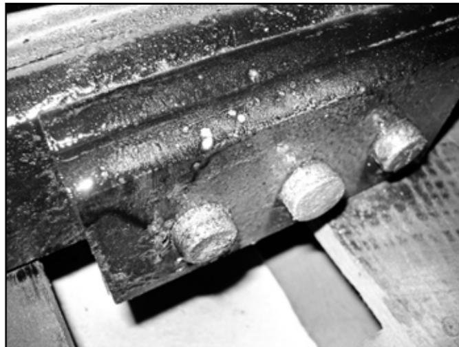
55. Repeat block and u-bolt installation on opposite side of the vehicle.
