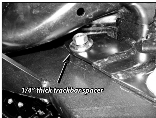
28. Fish the bolt tab through the frame rail with the included bolt wire and attach to the trackbar bracket with 1/2" USS washer and regular nut. Apply loctite to the bolt threads. Attach the upper hole with 1/2" x 1-3/4 (#792) bolt with spacer washer as shown. (Fig 15a, 15b)
