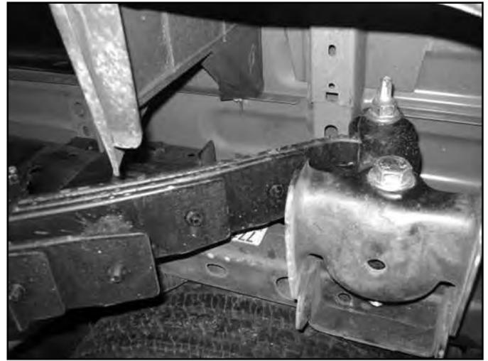
51. Install new u-bolts and install the nuts, snug but do not tighten at this time.
