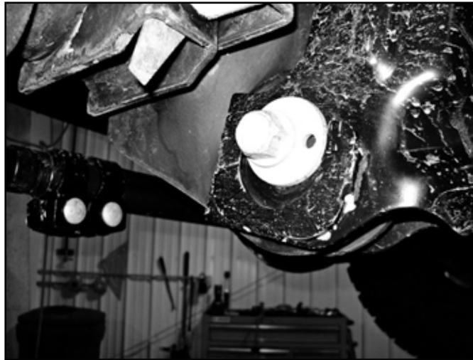
44. Turn the steering wheel to get the trackbar to align with the bracket. Install new 18mm bolt and tighten to 150 ft-lbs (#792).
