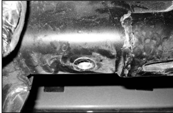
19. Place the machined sleeve into the existing frame rail hole. Reinstall the bracket with hardware (#793) and sleeve as shown (Fig 11a, 11b, 11c)
