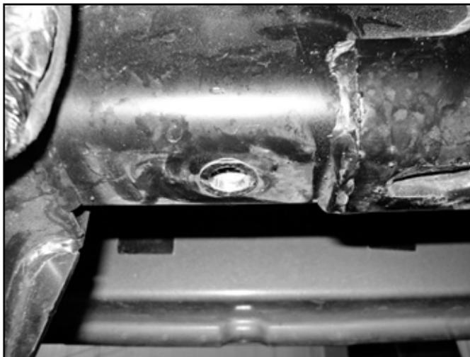
23. Place the machined sleeve into the existing frame rail hole. Reinstall the bracket with hardware (#788) and sleeve as shown. Due to variations in the factory brackets, shims are included to go between the bracket and transmission crossmember to take up the slack. Drop the shims in from the top. There are (2) 1/8" shims and (2) 1/16" shims included. Shims may need to be stacked. (Fig. 11a-g)
