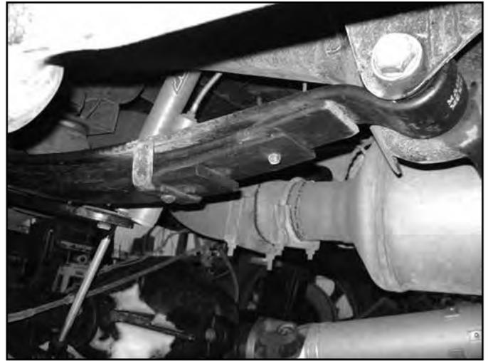
66. Lower axle enough to install new block with the bump stop wing facing in. If installing air bags, the wing will need to face towards the caliper side of the wheel to allow for clearance.
