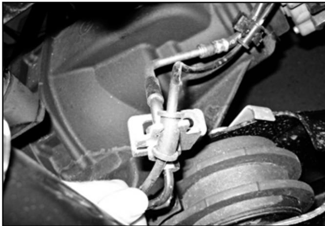
13. Disconnect the brake line from the ABS wires.
