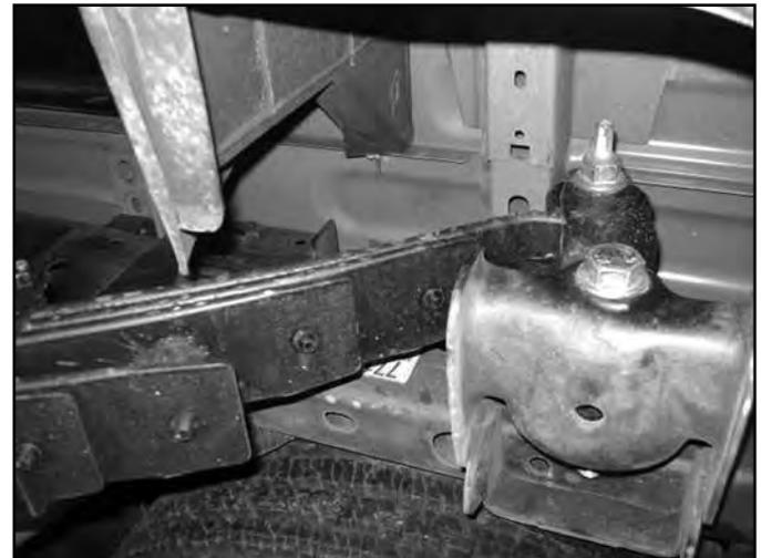
57. Install new 2" lift block BACKWARDS (large end in front - small towards rear) with new u-bolts and install the nuts, snug but do not tighten at this time. Note: the new u-bolts are 5/8", which means they are larger and stronger than factory 14mm. The factory leaf spring plate will need to be modified to clear the u-bolts. Grind or drill out the mounting plates slightly for adequate clearance.
