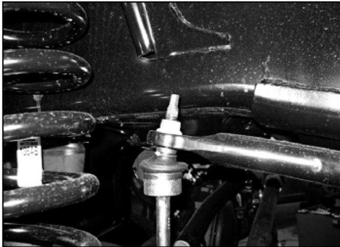
12. Disconnect the brake line bracket from the top of the radius arm mount on the axle, retain bolt, discard bracket. (Fig. 5a)
