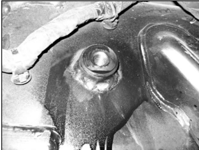
22. Insert the rivet nut into the bottom of the frame rail. Use the hardware (#799) to set the rivet nut into place as shown (Fig. 10). See the end of the instruction sheet for detailed rivet nut installation instructions.
