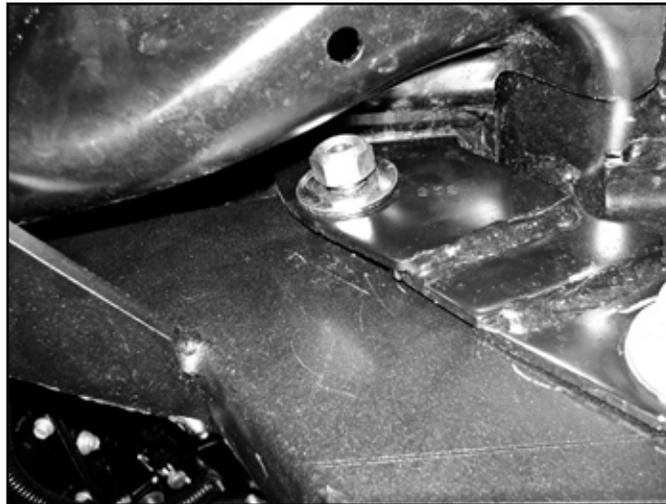
34. Fish the bolt tab through the frame rail with the included bolt wire and attach to the trackbar bracket with 1/2" USS washer and regular nut. Apply loctite to the bolt threads. Attach the upper hole with 1/2" x 1-3/4 (#789) bolt with spacer washer as shown. (Fig. 15a, 15b)
