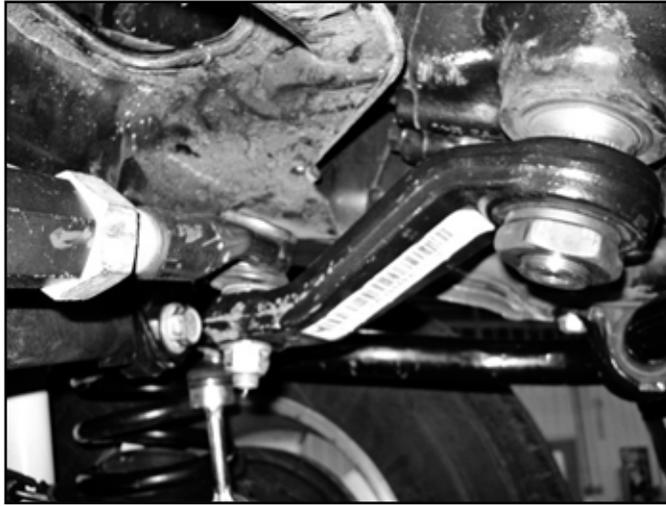
11. Disconnect the sway bar links from the sway bar they will not be reinstalled. (Fig. 4)
