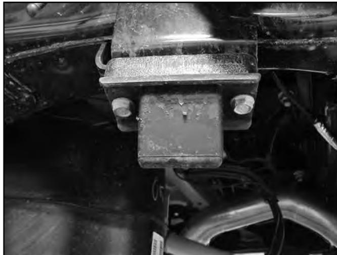
20. **2.5-3.5" Bump Stop Installation:** Install the bump stop drop brackets with new 10mm hardware to the frame (BP 458). Install so the gusseted side faces in and offsets the bumpstop towards the center of the vehicle. Using the provided 10mm bolts, nuts, and washers, attached the bump stop directly to the bottom of the drop bracket. The factory spacer will not be used. Tighten to 35 ft-lbs. (Fig 13)
