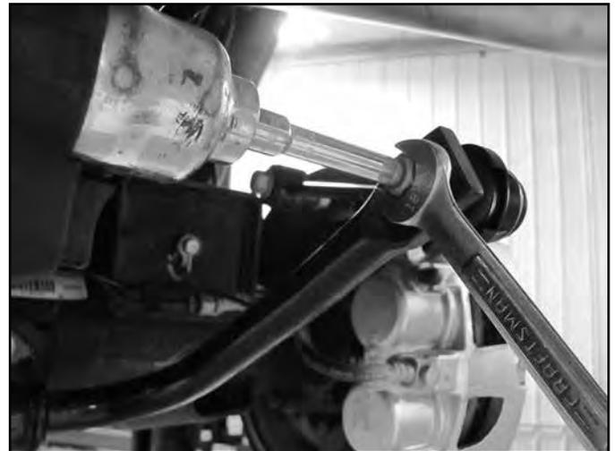
8. Loosen the air fittings at the valve block on the passenger side frame rail to allow the air to bleed from the rear bags (Fig 3).
