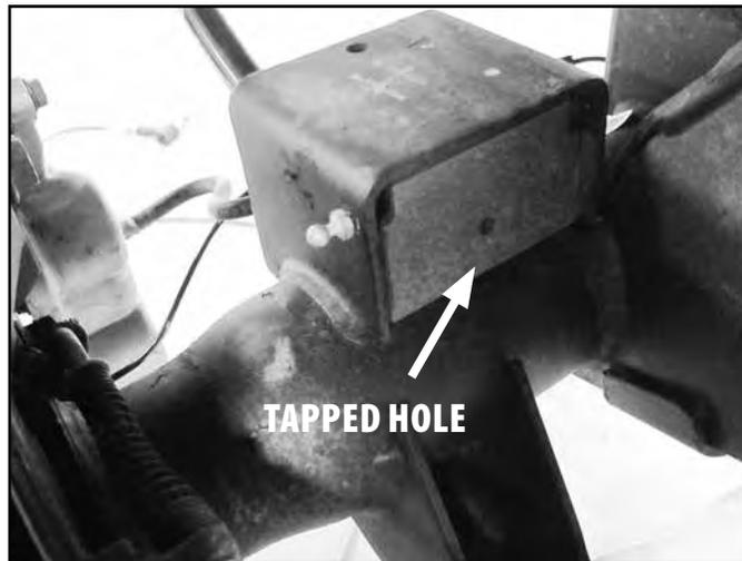
24. Fasten the sensor relocation brackets to the axle with the 3/8" self tapping bolt and provided 6mm bolt and washer (BP 460)
