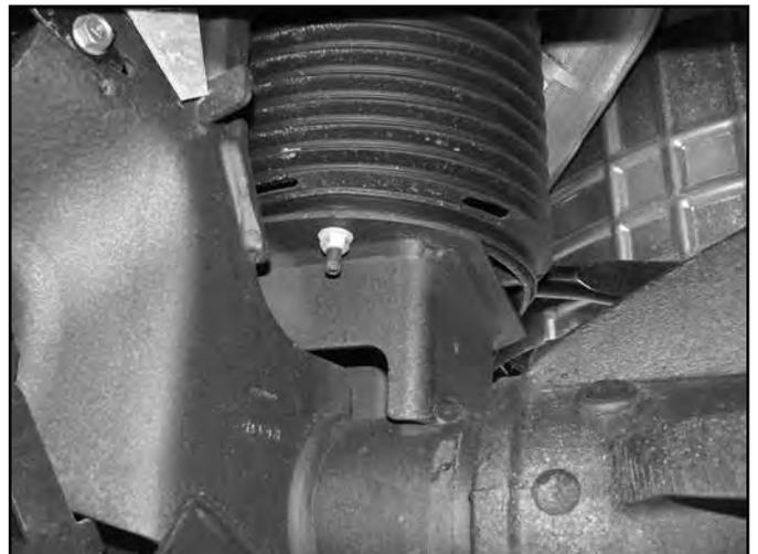
12. Locate the holes in the rear lower air bag mount. Clearance the rear most hole on the driver's side to 1/2" to accept larger track bar hardware, the remaining 3 holes will accept 3/8" hardware. (Fig. 7)
