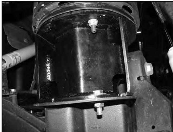
17. **3.5" - 5" Kit BDS NX2 Shock Installation:** BDS (Silver body) shocks will require a stem eliminator bracket to be installed and tightened on the shock before installation. The hardware is in bolt pack 946 included in the shock box. (Fig. 10 on Left)
