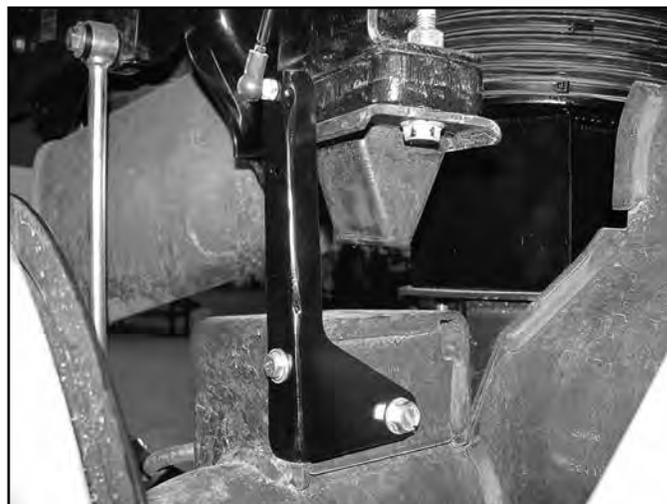
25. Attach the factory linkage stud to the linkage bracket with the provided nylock nut (BP460). Use the following image as a guide for your desired ride height. Pop the linkage rod back onto the stud.
