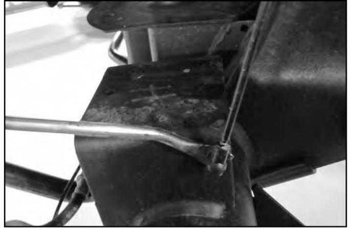
10. Disconnect the rear shocks and lower the axle, retain hardware. On the driver's side it is easiest to access the top hardware by cutting the inner fender well as shown. This trim procedure is not required but greatly aids in removal and installation of the shock (Fig 5a, 5b).
