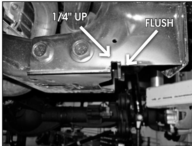
16. Place the radius arm drop bracket up to the frame rail. Insert  $\frac{3}{4}$ " bolt to locate the bracket. Mark the center of the slot on the bottom of the frame rail, mark the center of the top, rear hole on the side of the frame rail. (Fig. 8)
