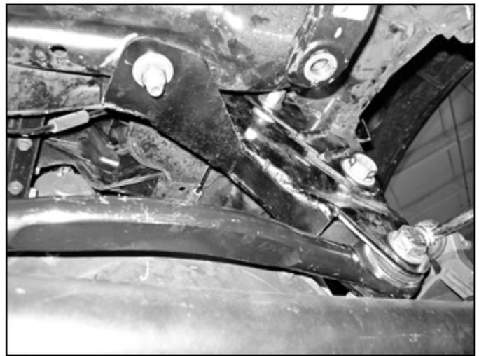
29. Tighten 1/2" trackbar hardware to 65 ft-lbs. Tighten 18mm factory bolt to 150 ft-lbs.
