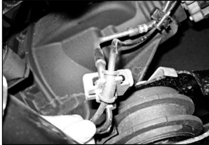
12. Disconnect the factory shock from the lower shock mount. (Fig. 6) Lower the front axle and remove the factory coil springs.
