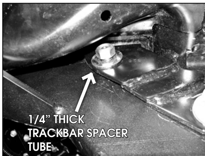
28. Fish the bolt tab through the frame rail with the included bolt wire and attach to the trackbar bracket with 1/2" USS washer and regular nut. Apply loctite to the bolt threads. Attach the upper hole with 1/2" x 1-3/4 (#792) bolt with spacer washer as shown. (Fig. 15A, 15B)
