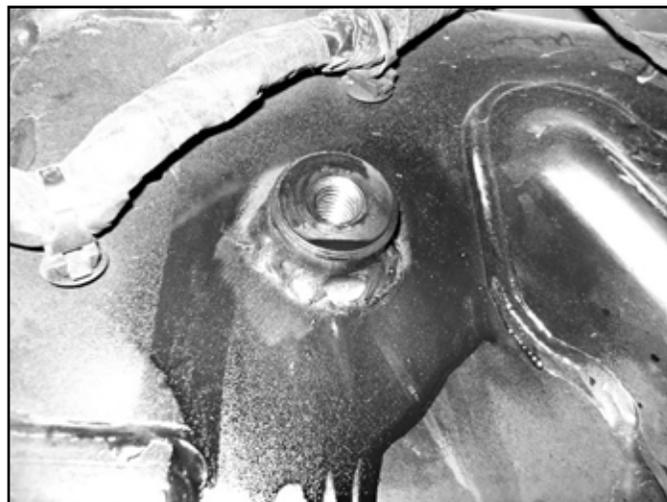
18. Insert the rivet nut into the bottom of the frame rail. Use the hardware (#799) to set the rivet nut into place as shown (Fig. 10) See the end of the instruction sheet for detailed rivet nut installation instructions.
