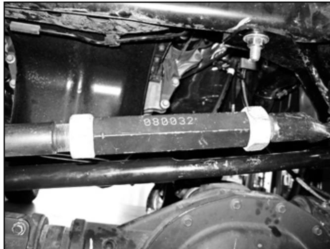
37. Install new pitman arm, use alignment mark made earlier. Loctite factory nut and install with lock washer tighten nut to 225 ft-lbs.
