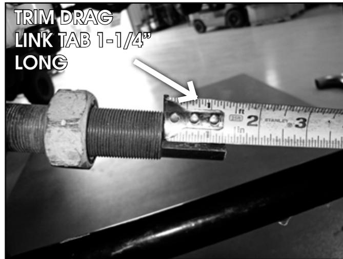
36. Reassemble the drag link, adjust so that there is approximately  $\frac{3}{4}$ "~ $\frac{7}{8}$ " of thread exposed past the jam nuts and that the tie rod end faces up. (Fig. 18)
