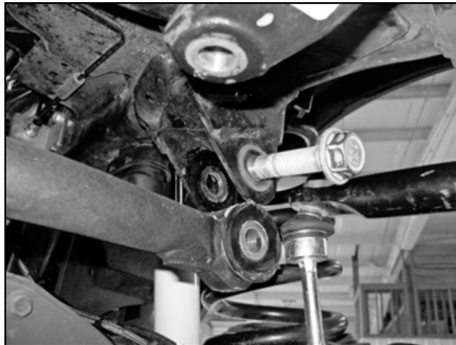
4. Raise the front of the vehicle and support the frame rails with jackstands. Do not support on the radius arms, they will be removed during the installation.
