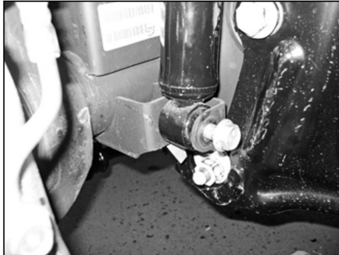
13. Raise the front axle and reattach factory shocks with factory bolt. It is not necessary to put the nut tab back on. The shocks will be there to keep the axle secure. Keep a jack under the axle for extra support.
