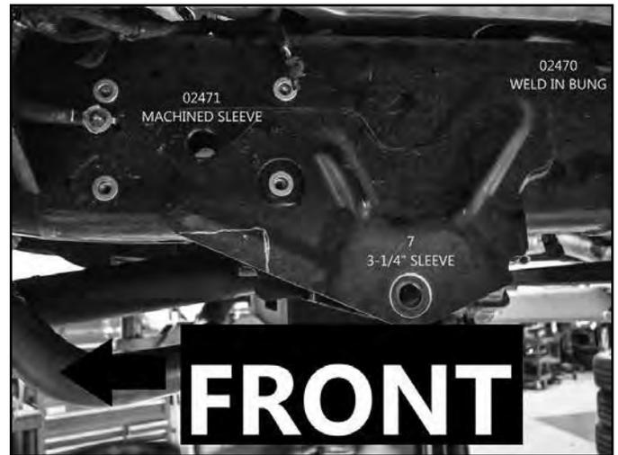
20. With a jack still under the axle, disconnect the radius arm from the driver's side frame bracket. Reinstall the passenger's side radius arm with factory hardware. Rotate the cam to the marked position. Leave hardware slightly loose.
