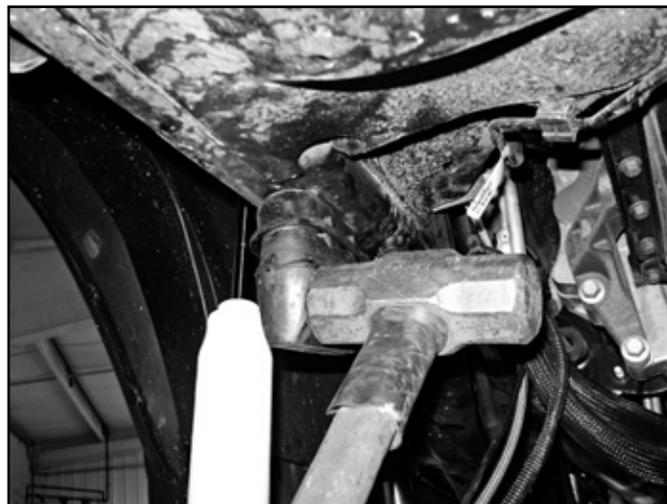
24. Grease new replacement bump stops and raise axle to press the bump stops into position. These will be a tight fit. It is easiest to lift the axle with a jack to compress the bump stops into position. (Fig. 13)
