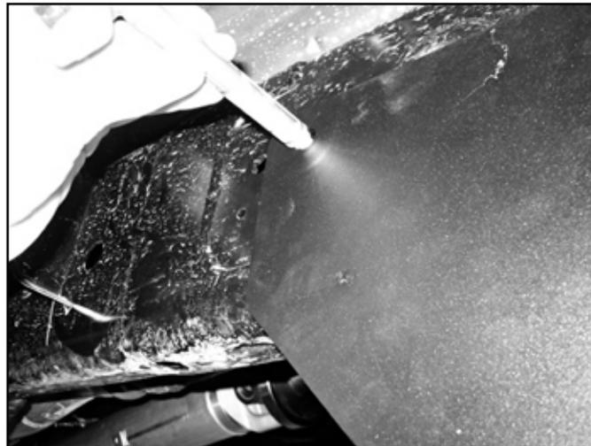
17. Remove the bracket and drill the 2 centers to  $\frac{11}{16}$ ". Prep the area on the side of the frame rail for welding. Place the weld in bung into the hole and weld the bung into place. (Fig. 9)
