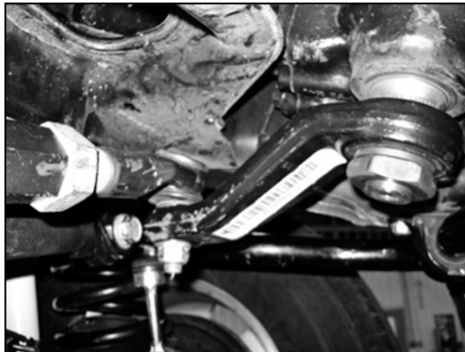
12. Disconnect the sway bar links from the sway bar. Retain all hardware. (Fig. 4)
