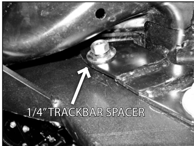
33. Fish the bolt tab through the frame rail with the included bolt wire and attach to the trackbar bracket with 1/2" USS washer and regular nut. Apply loctite to the bolt threads. Attach the upper hole with 1/2" x 1-3/4 (#789) bolt with 1/4" spacer (01499) washer as shown. (Fig. 15a, 15b)
