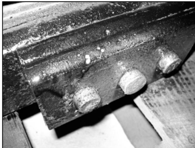
63. Install new lift block with new u-bolts and install the nuts, but do not tighten at this time.
