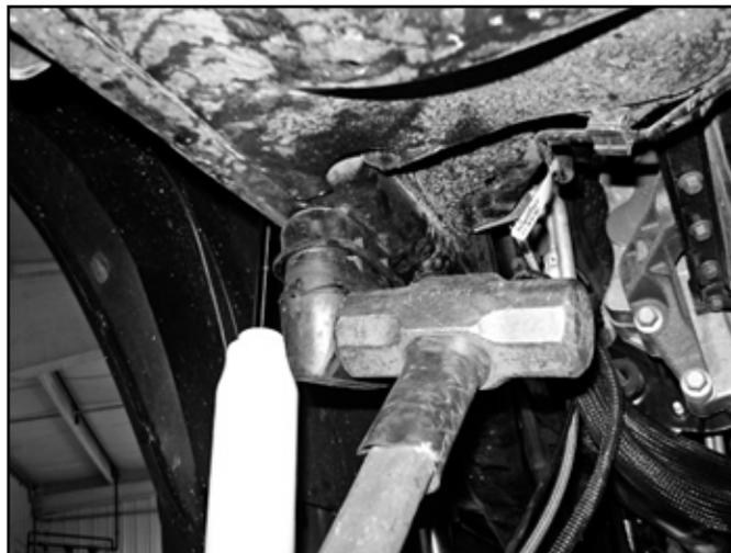
29. Grease new replacement bump stops and raise axle to press the bump stops into position. These will be a tight fit. It is easiest to lift the axle with a jack to compress the bump stops into position. (Fig. 13b)
