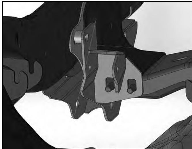
23. Grease and install bushing and sleeves into the lower control arm. Thread the grease fitting into the arm.
