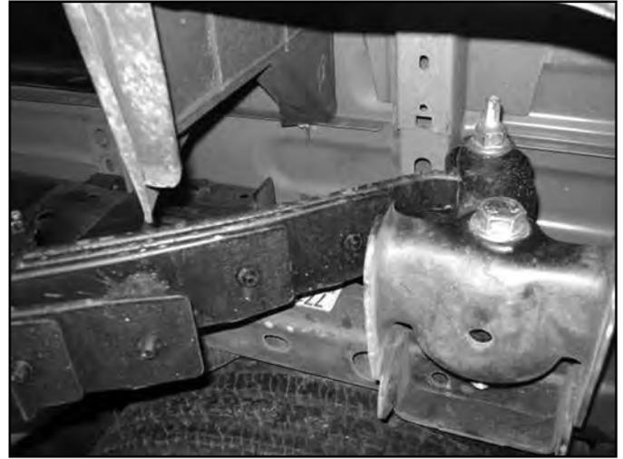
59. Install new u-bolts and install the nuts, snug but do not tighten at this time.
