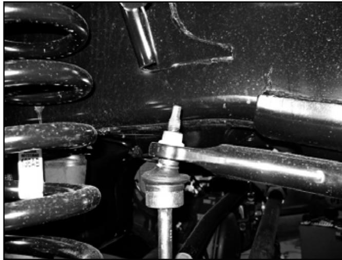
13. Disconnect the brake line bracket from the top of the radius arm mount on the axle, retain bolt, discard bracket. (Fig. 5)
