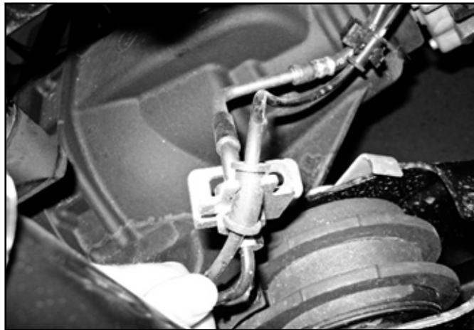
14. Disconnect the front driveshaft from the axle, retain the 4 bolts.
