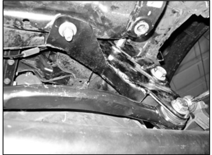
34. Tighten 1/2" trackbar hardware to 65 ft-lbs. Tighten 18mm factory bolt to 250 ft-lbs.
