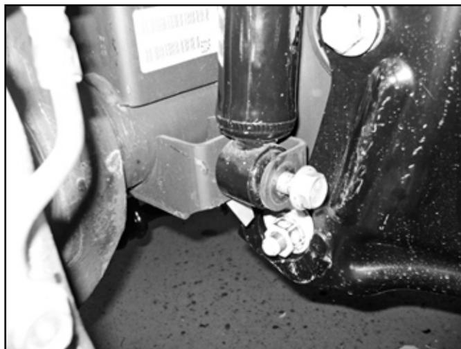
16. Raise the front axle and reattach factory shocks with factory bolt. It is not necessary to put the nut tab back on. The shocks will be there to keep the axle secure. Keep a jack under the axle for extra support.
