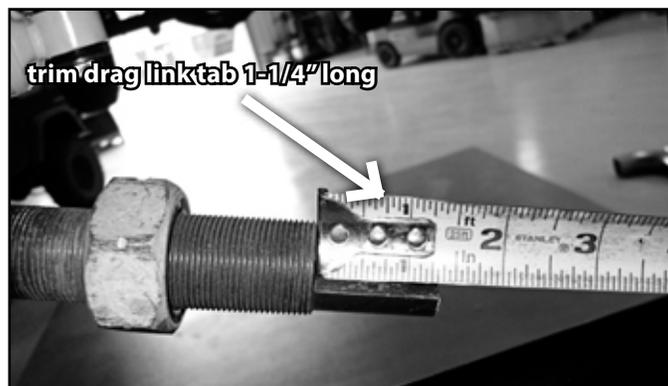
41. Reassemble the drag link, adjust so that there is approximately  $\frac{3}{4}$ "~ $\frac{7}{8}$ " of thread exposed past the jam nuts and that the tie rod end faces up. (Fig. 18)
