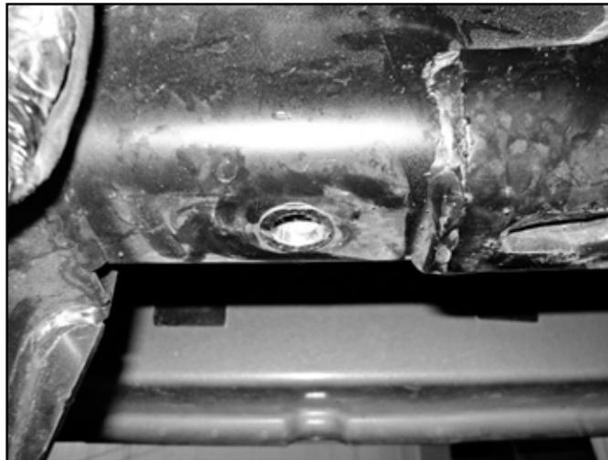
22. Place the machined sleeve into the existing frame rail hole. Reinstall the bracket with hardware (#788) and sleeve as shown. There will be a spacer sleeve that goes between the bracket and frame. Due to variations in the factory brackets, shims are included to go between the bracket and transmission crossmember to take up the slack. Drop the shims in from the top. There are (2) 1/8" shims and (2) 1/16" shims included. Shims may need to be stacked. (Fig. 11a-h)
