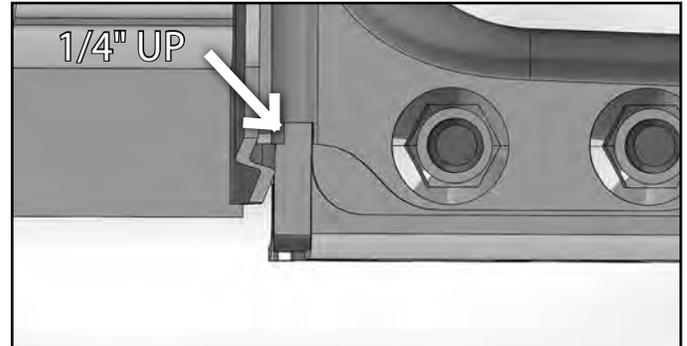
19. Remove the nuts from the transmission crossmember, if not already done in the transfer case index installation. Place the 4-link bracket up to the frame rail. Insert  $3/4$ " bolt to locate the bracket. Mark the center of the slot on the bottom of the frame rail, mark the center of the top, rear hole on the side of the frame rail. (Fig. 8)
