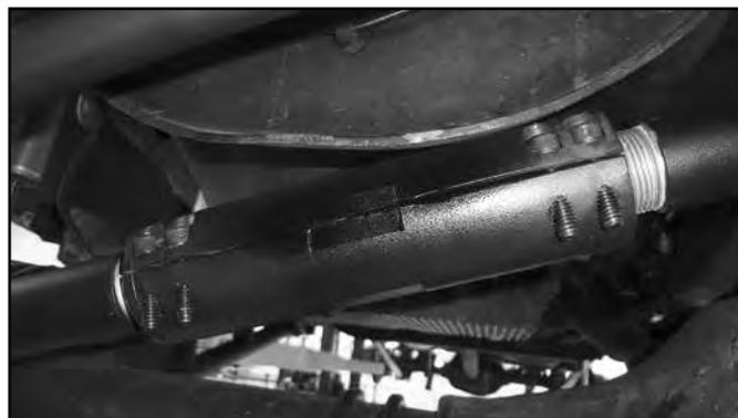
24. Attach the axle mount to the track bar. It may be necessary to have an assistant turn the wheel to get the mount to line up. Square the mount up to the factory joint. Attach with factory nut. Tighten to 184 ft-lbs
