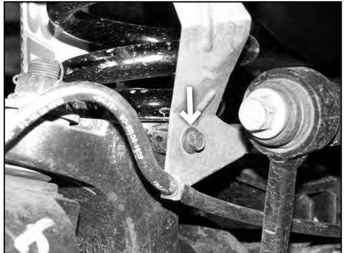
12. Disconnect the brake line bracket from the front of the coil perch (Fig 6). Retain hardware.
