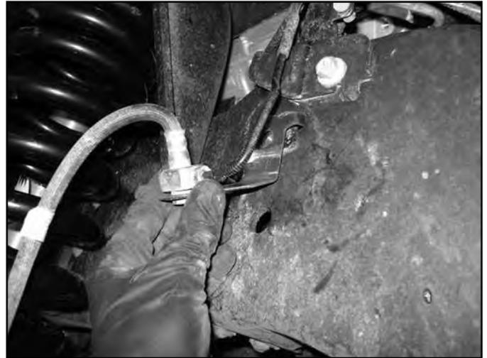
29. Check all hardware for proper torque.
