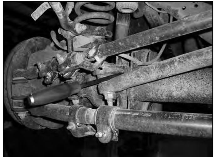
4. Disconnect the front track bar from the frame mount.
