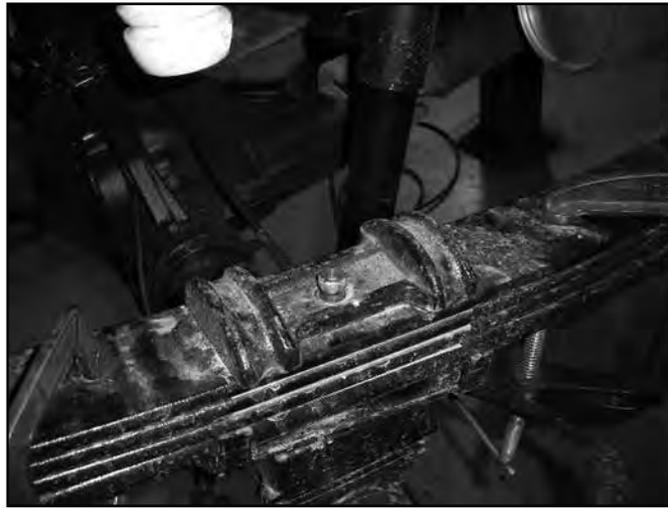
38. Remove the factory lift block. It will not be reused.
