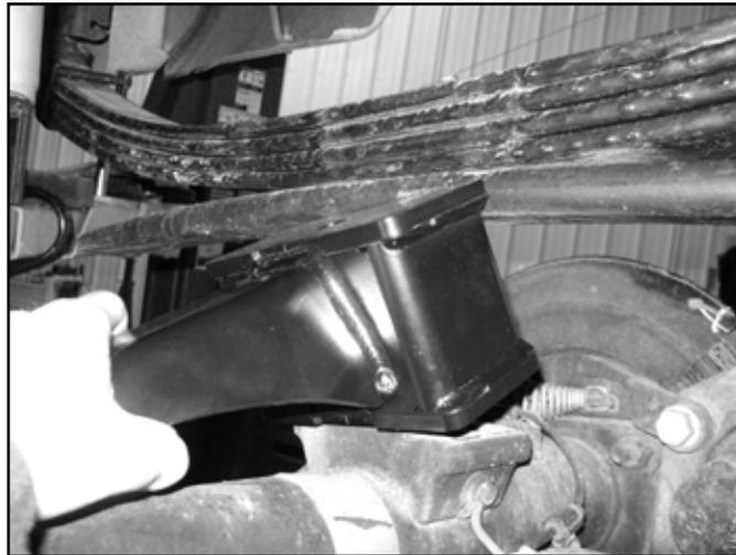
41. Repeat block installation of the driver's side. Take care not to over extend the brake lines.
