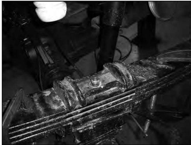
44. Remove the factory lift block. It will not be reused.
