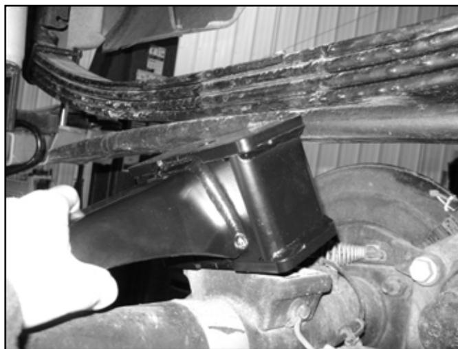
47. Repeat block installation of the driver's side. Take care not to over extend the brake lines.
