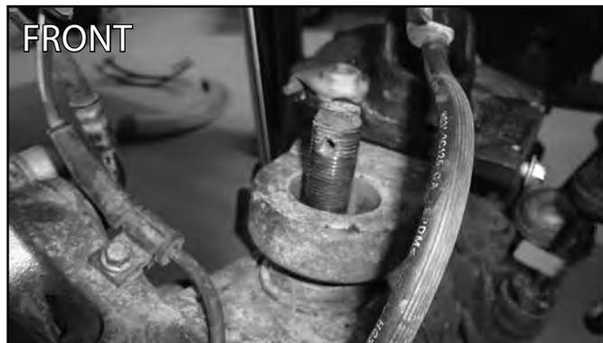
19. Install the new sleeve with the arrow on the top of the sleeve pointing toward the front of the vehicle. Using the old sleeve, pound down on the new sleeve to seat it on the ball joint taper. Make sure that the flat of the sleeve is flush with the flat of the axle (Fig C).
