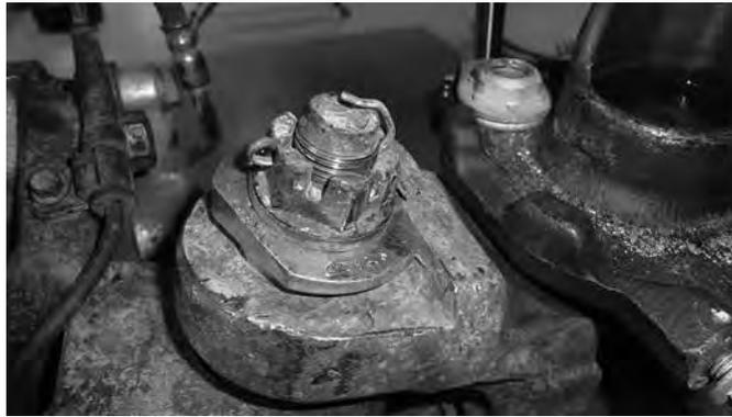
21. Install the shim under the factory coil spring mount with the thick end of the shim at the FRONT of the vehicle. Place the machined washer on the inside of the coil spring mount, thick area of machined washer will be at the REAR of vehicle. Attach with new 14mm bolt with lock washer (#824), tighten to 65 ft-lbs. (Fig 9a, 9b).
