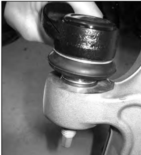
8. Remove the upper and lower ball joint nuts and re-install a few turns, refrain from hitting the aluminum steering knuckle, use appropriate tool to separate ball joints, avoid damaging the threads.
