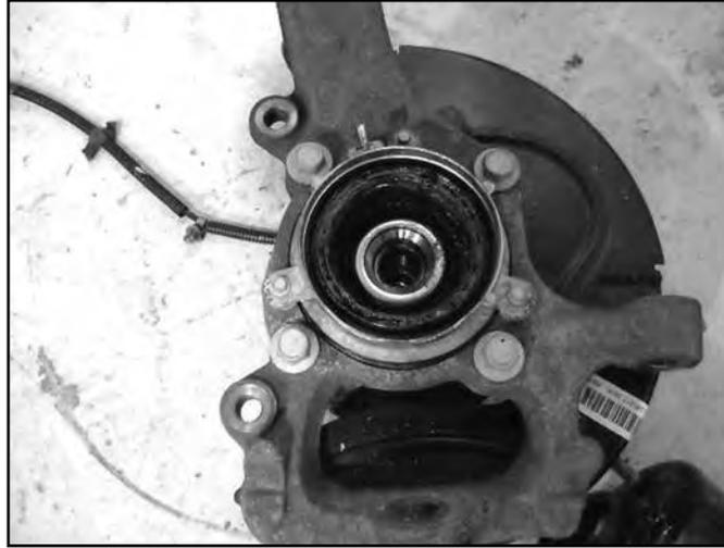
29. Install the hub into the corresponding new BDS knuckle and fasten with the OE bolts. The ABS wire will be located at the 'top' of the hub. Use Loctite on the bolt threads and torque to 148 ft-lbs.
