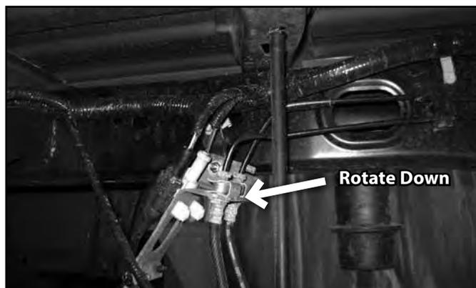
58. Attach the brake line to the relocation bracket with a ¼" nut and ¼" USS washer (BP #774). It may be necessary to rotate the OE brake line clip bracket to have the lines face 'down' for adequate slack. Torque to 15 ft-lbs.
