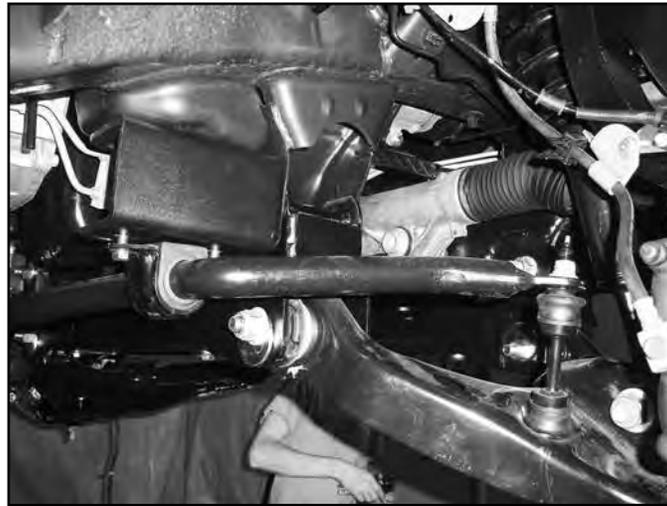
38. Install tie rod ends to the knuckles from top-down. Torque to 111 ft-lbs.
