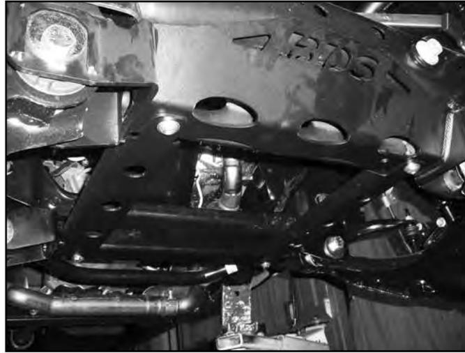
20. Install the lower control arms in the new crossmembers and fasten with the provided 18mm cam bolts, cam washers and 18mm nuts. Run the front bolts from front to rear and leave loose. Run the rear bolts from rear to front. The main body of the cam will be 'up' in the cam slot.
