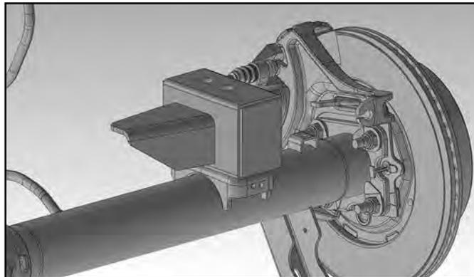
56. Attach u-bolts with the factory lower u-bolt plate. Snug u-bolts, they will be torqued to specification when the vehicle is on the ground.
