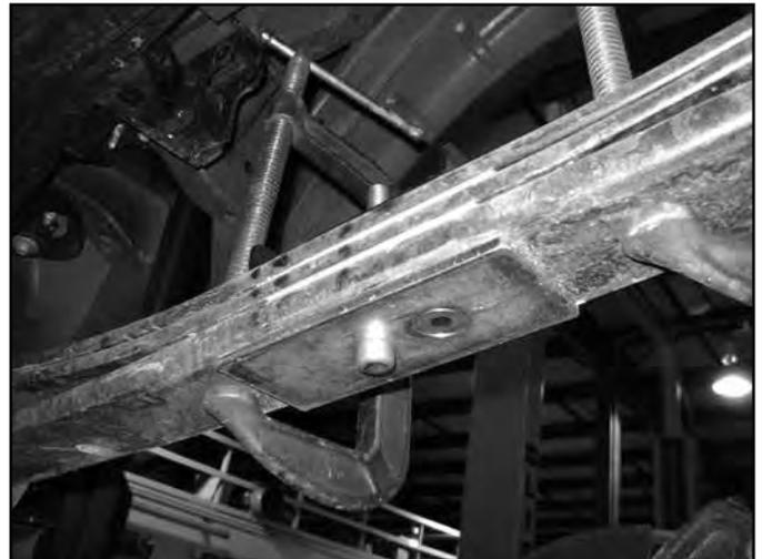
52. Install the new provided lift block so that the bump stop wing goes toward the inside of the vehicle. The block will use the both of the lower center pin holes. The upper only uses 1 hole which will shift the axle slightly forward.
