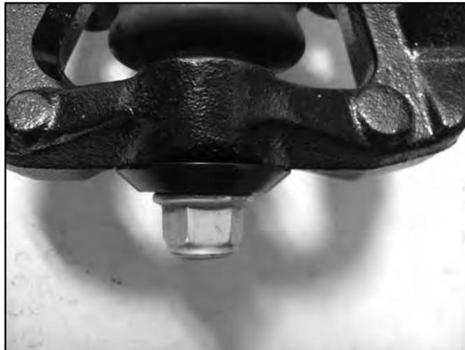
32. Attach the upper control arm to the knuckle with the original nut. Torque the upper ball joint to 85 ft-lbs and the lower ball joint to 111 ft-lbs. Make sure the larger lower balljoint washer is centered before tightening.
