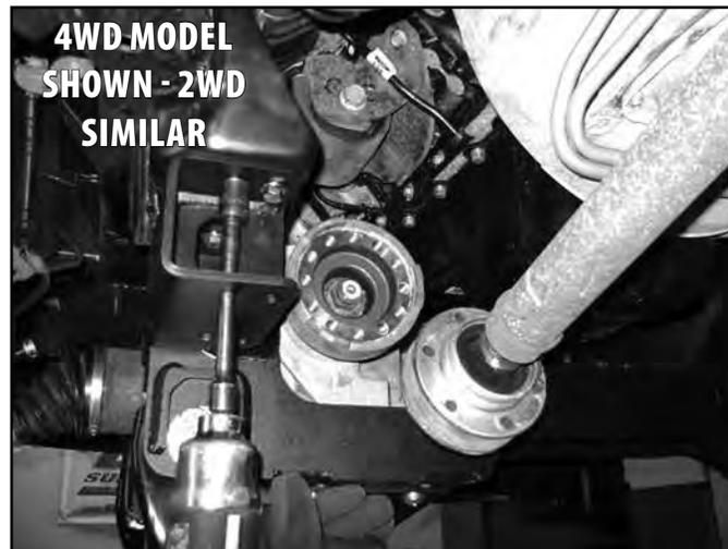
23. With the lower control arms installed, go back and torque the four crossmember mounting bolts to 222 ft-lbs. Ensure that the front crossmember is centered in the vehicle. Apply Loctite to the threads and torque the crossmember support bolts to 50 ft-lbs. Tighten sway bar drop hardware to 35 ft-lbs.
