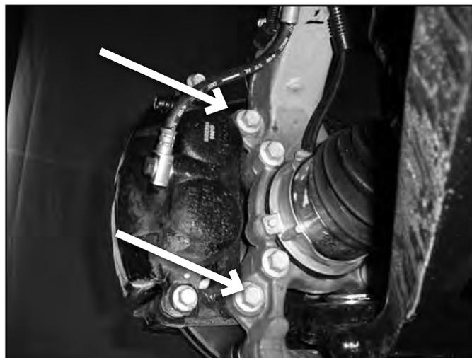
6. Disconnect the ABS lines from the retaining clips. Disconnect the brake line bracket from the frame rail. Disconnect the ABS line from the hub assembly. (Fig 2).
