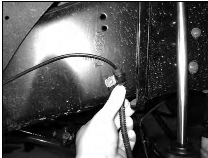
40. 4" Lift Only: Remove the factory front brake line brackets from the frame. The brackets have a squared edge in the brake line mounting hole. (Fig 14A) Using a file or rotary grinder, remove the square edge to form a complete round hole. (Fig 14B) Reattach the brackets to the frame tighten securely with the factory hardware. Install the brake line junction in the bracket from the bottom and fasten with the factory retaining clip. (Fig 14C)
