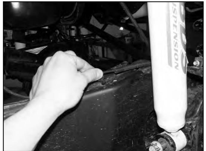
11. Disconnect the OE steering stabilizer from the frame mount.
