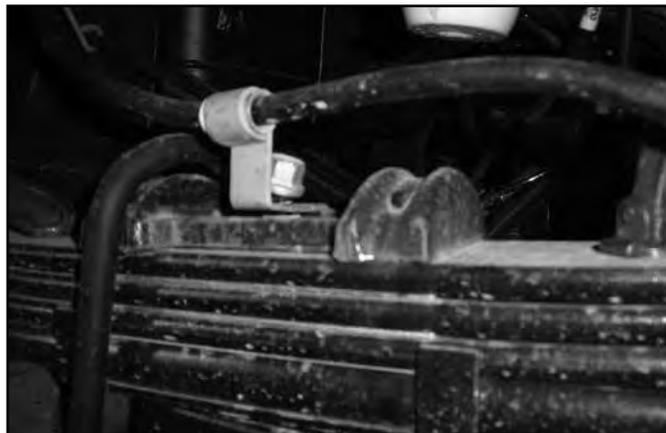
68. If more parking brake cable slack is needed, remove the cable from the rear-most retaining bracket on the frame. (Fig 21)
