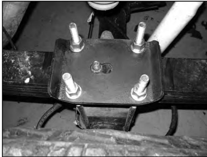
61. Repeat block installation of the driver's side. Take care not to over extend the brake lines.
