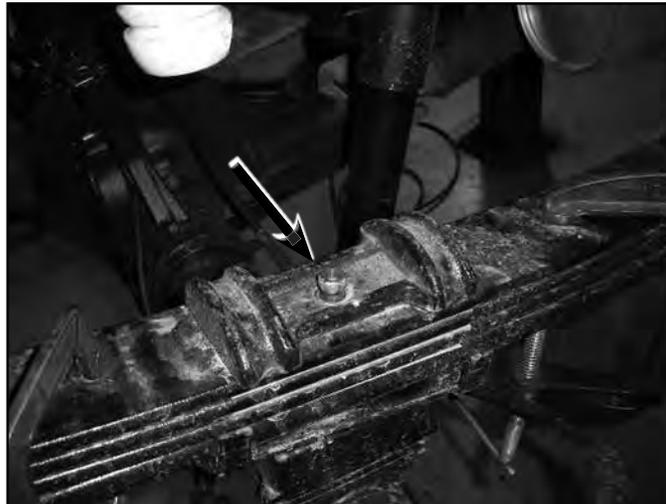
58. Remove the factory lift block. It will not be reused.
