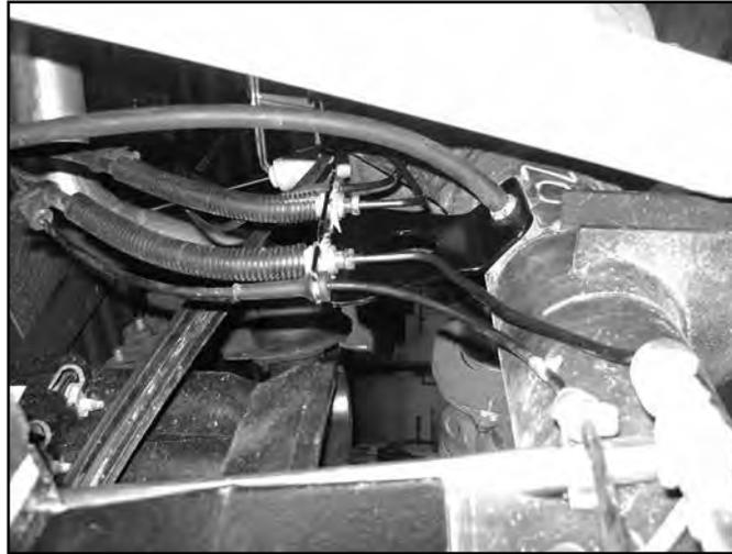
55. Disconnect the brakeline bracket from the rear axle by removing the breather tube stud. Discard the bracket, retain the breather tube stud.
