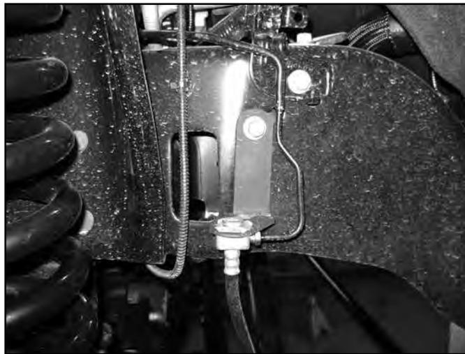
42. Properly bleed the brake system of air and top off the brake fluid reservoir with the proper type of fluid (see owners manual).
