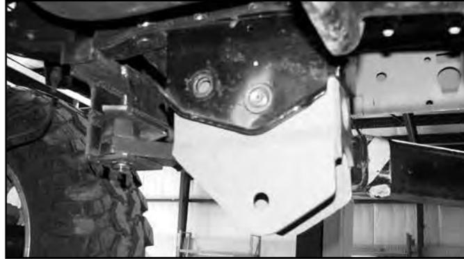
29. Swing the radius arm up into the new bracket and fasten with the original mounting hardware. Leave loose.
