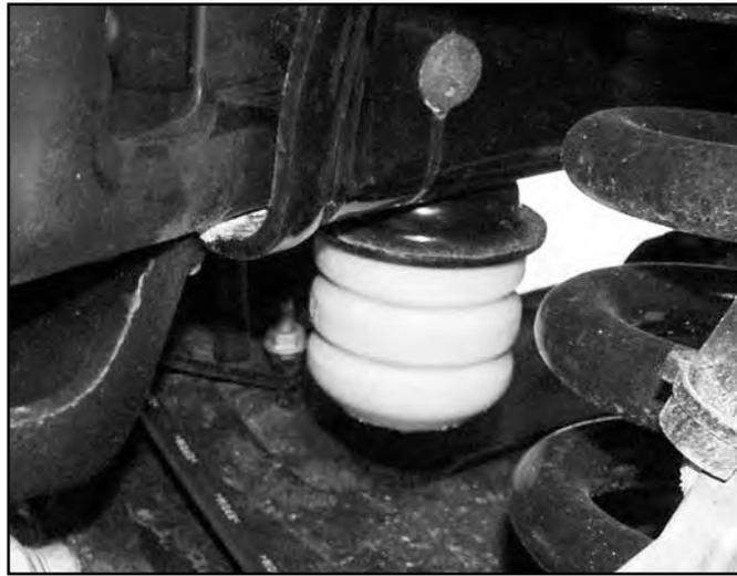
24. Position the cup on the provided bump stop extension. (01001) The alignment tab on the bump stop cup will fit in the second hole in the extension.
