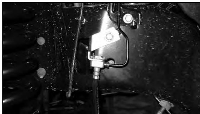
53. 6" Lift Only: Remove the factory brake line brackets from the frame. Install the new provided brake line brackets and secure with the factory hardware. Carefully reform the brake hard line and install the junction block through the bottom of the new bracket. (Fig 22) Fasten with the original brake line clip.
