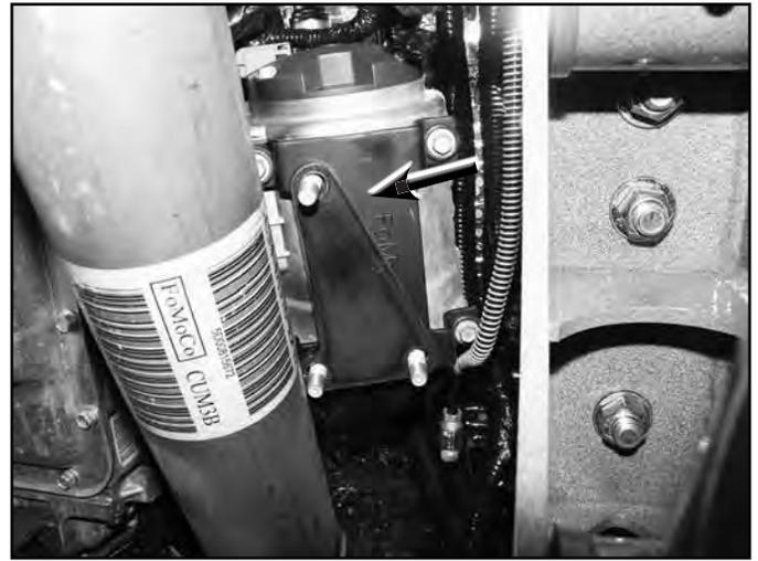
42. With all of the control arms attached, reinstall the fuel junction block (if removed) on the driver's side frame rail. Torque hardware to 20 ft-lbs.
