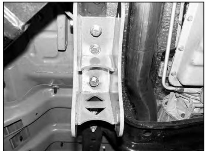
34. Install the assembled upper control arm in the new frame bracket and fasten with a  $\frac{3}{4}$ " x 5-1/2" bolt, nut and  $\frac{3}{4}$ " SAE flat washers from bolt pack #432. The two tabs on the control arm go up. Leave hardware loose. (Fig. 14)
