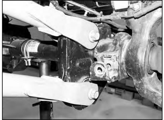
36. Install the new lower control arm in the new frame bracket with a  $\frac{3}{4}$ " x 5-1/2" bolt, nut and  $\frac{3}{4}$ " SAE flat washers. Install arm so that the grease fitting is up. Leave hardware loose.
