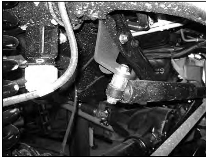
14. Disconnect the (5) bolts mounting the OE track bar bracket to the frame. Remove bracket and retain hardware.
