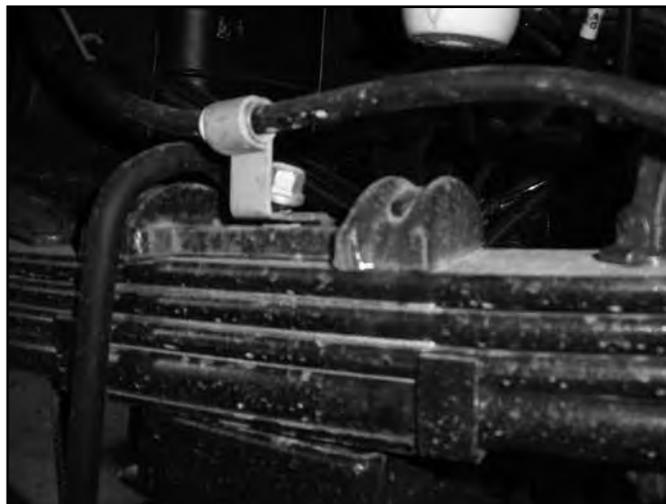
74. If more parking brake cable slack is needed, remove the cable from the rear-most retaining bracket on the frame. (Fig 28)
