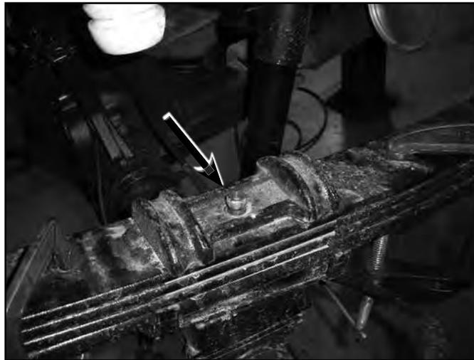
64. Remove the factory lift block. It will not be reused.
