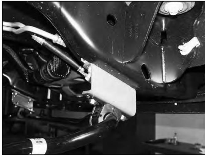
49. Install the sway bar link ends to the sway bar and secure with the OE hardware. Torque to 90 ft-lbs.
