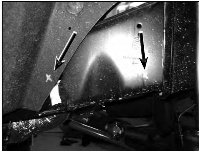
51. Locate the provided wire clamps, 1/4" self tapping bolts (BP 656) and mountable zip ties (tree on the end). With the suspension at full extension (hanging from shocks) ensure that the ABS line still has some slack from the new mounting point on the frame to the axle. Fasten the line to the frame with the wire clamp and 1/4" self-tapping bolt. (Fig 20B) Attach the loose end inside the inner fender with the mountable zip tie.
