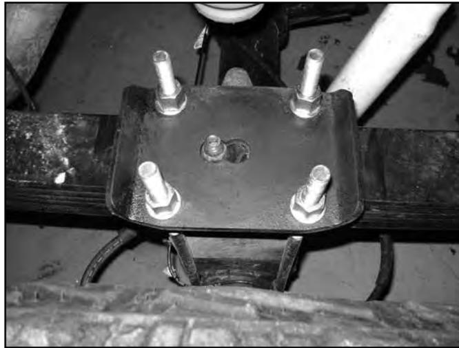
67. Repeat block installation of the driver's side. Take care not to over extend the brake lines.
