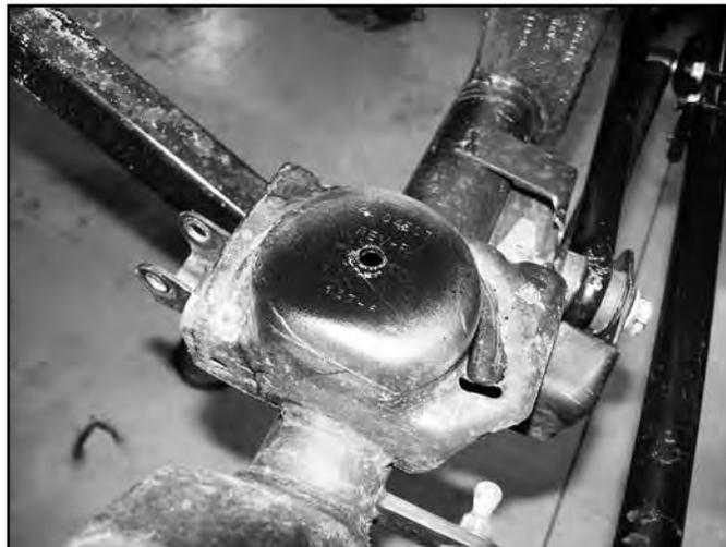
10. Place a provided bump stop extension inside one of the new front coil springs and install the spring in the vehicle. Make sure the spring is seated properly in the axle mount.
