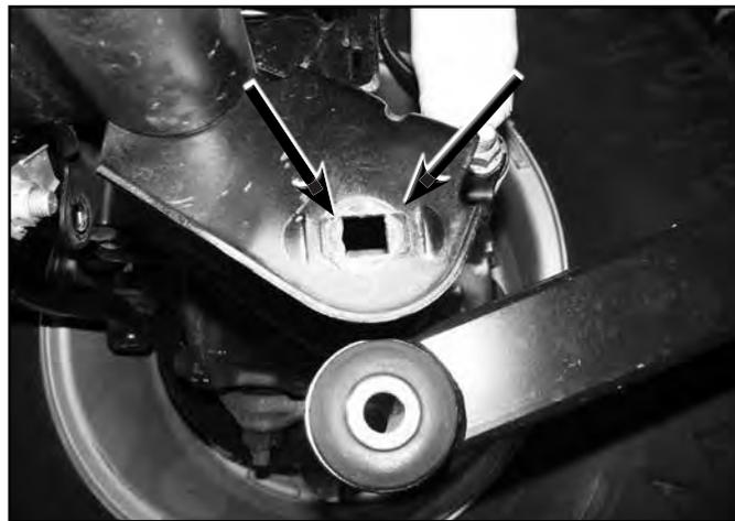
17. When the perforated sections are removed from the lower control arm mount, reinstall the control arm to the axle with octagon cams on factory bolt. Rotate the cams so that the bolt is as far towards the 'rear' of the slot as possible. Just snug the cam hardware so that the cam washers are retained within the stops. Final cam bolt torque will be completed with the weight of the vehicle on the suspension. (Fig 4)
