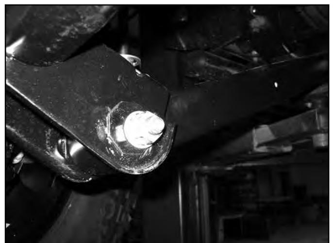
24. Repeat cam bolt installation on the driver's side.
