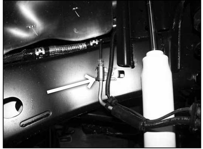
8. Remove the OE steering stabilizer. Save hardware. Leave the stabilizer bracket on tie rod. (Fig 4)
