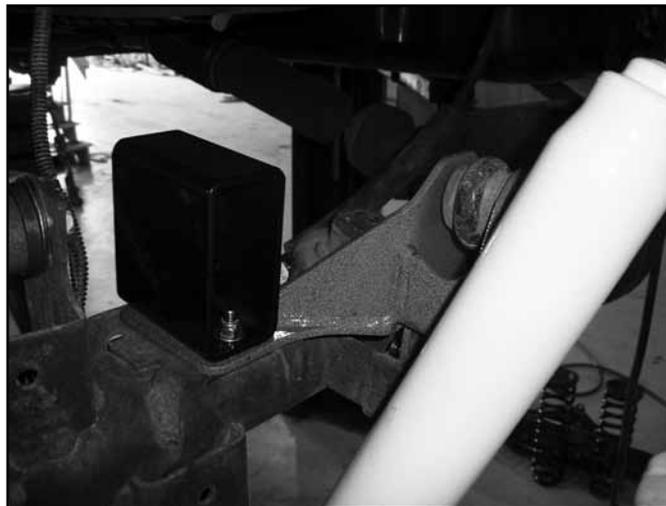
60. With the support wing/bump stop hardware tight, torque the 3/8" (35 ft-lbs) and 9/16" (100 ft-lbs) track bar bracket hardware.
