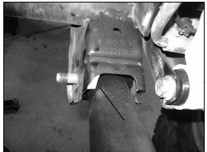
19. Using the OE hardware, install the arms so the bend is up and towards the center (Figure 8). The bend is centered. It may be necessary to raise or lower the axle to align the control arm bolts. Leave hardware loose, it will be tightened with the vehicle at ride height.
