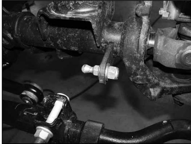
35. Connect the sway bar links to the ball studs on the axle. Adjust the sway bar link ends so that they are square on the ball stud and lock off the jam nut securely.
