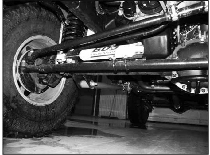
40. Cycle steering and check for proper clearance, adjust as necessary. Tighten 1/2" hardware to 65 ft-lbs, u-bolts to 25 ft-lbs, and stabilizer OE 12mm hardware to 55 ft-lbs.
