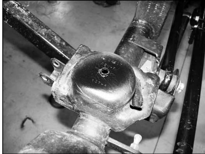
27. Tap hole threads by using the 3/8" x 1-1/4" self-tapping bolt provided in bolt pack 438. Remove and reuse for the other coil pad.
