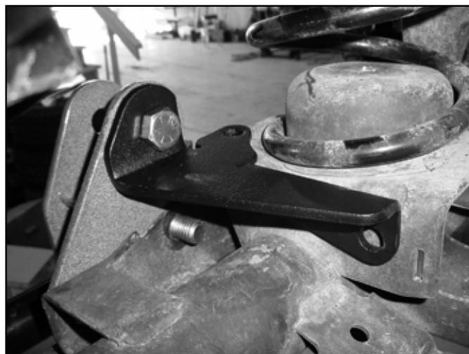
24. Make sure the support bracket is setting flush to all mounting surfaces and mark the two holes to be drilling in the coil mount. Remove the support bracket and drill 3/8" holes at the marks.
