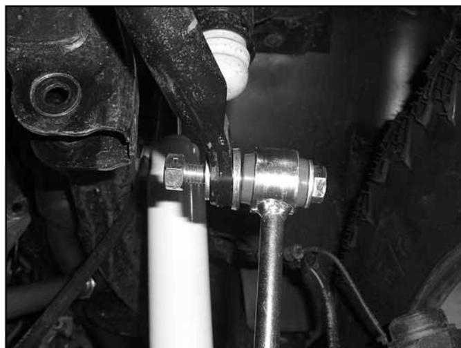
33. Locate the new sway bar link assemblies. Ensure that they are adjusted to equal length. The links should be adjusted between 8-1/2" and 8-3/4" from the center of the bushing to the very end of the disconnect. Do not lock off the jam nuts at this point.
