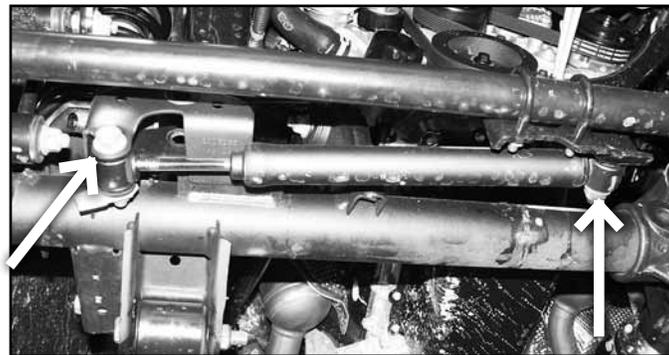
9. Disconnect the sway bar links from the axle and sway bar. (Fig 5)
