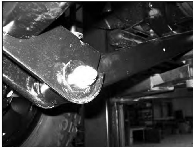
16. Repeat cam bolt installation on the driver's side.
