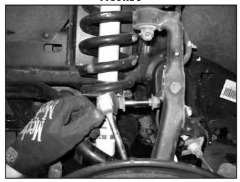
8. Remove the sway bar from the vehicle; remove the hardware that attaches the horse shoe shaped brackets to the frame. These 4 bolts will not be reused. (Fig 6)
