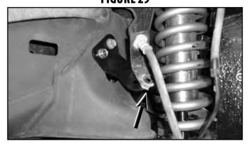
61. Attach the ABS wire to the upper control arm with new wire clamp and factory bolt. Attach to the bracket on the side of the steering knuckle with OE clip, adjust the clip as needed. Attach to the backside of the knuckle with new clamp and factory bolt. (Clamp is located in bolt pack #666) (Fig 30a, 30b)
