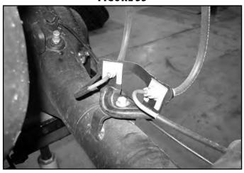
76. Disconnect the emergency brake from the frame, disconnect the bracket from the leaf spring clamp, remove the clamp from the cable. Retain hardware. (Fig 34)
