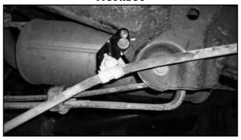
83. Install new rear brake line relocation bracket with 1/4" hardware (Bolt pack #668) (Fig 37) Tighten to 15 ft-lbs.
