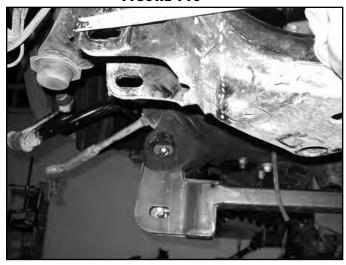
22. Measure over 7-1/4" from the first cut line and make another mark around the entire cross member. This should be on the center of the large circles. Make a vertical cut and remove the section from the vehicle. (Fig 14d, 14e)
