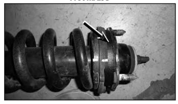
47. 4" & 6" kits: Install the strut spacers on top of the struts with factory nuts, tighten to 47 ft-lbs. The flat edge will face 'out' when installed in the vehicle. (Fig 24a, 24b)
