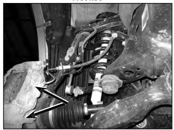
6. Disconnect the ABS wire from the upper control arm, backside of the steering knuckle, and steering knuckle bracket. Disconnect the ABS sensor from the steering knuckle. Use care not to damage the sensor. If it is difficult to remove, wait until the hub is removed and press from the inside of the hub bore. Retain hardware. (Fig 4a, 4b)
