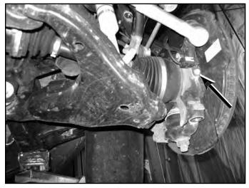
7. Disconnect the sway bar link from the steering knuckle. Do not damage the threads or the hex that is in the end of the sway bar link. (Fig 5)
