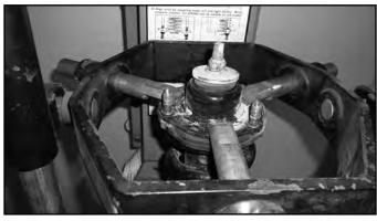
46. 6" kit only: Place the preload spacer between the rubber isolator and the top hat. Reassemble the entire strut assembly with factory hardware. (Fig 23b)
