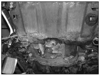
4. Remove the skid plate mounting bracket rails; keep all hardware (7 bolts) (Fig 2).
