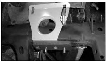
28. Disconnect the sway bar link from the sway bar. Cut out the template at the end of the instruction sheet. Place over the end of the sway bar. Trim / grind away approximately ¼" of material to give enough clearance between the sway bar and new steering knuckle. (Fig 17a, 17b)
