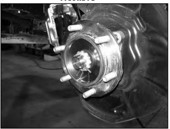
10. Remove the cotter pins on the upper balljoint and tie rod end. Remove nut, then loosely reinstall several turns by hand. Dislodge the taper by striking the side of the knuckle with a hammer as shown. (Fig 8)
