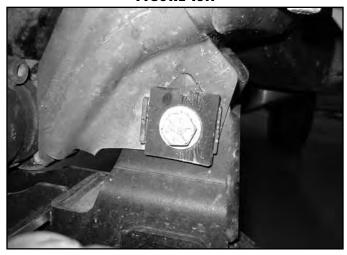
25. Mark the factory crossmember at the center of the slots on the back side of the BDS rear crossmember. Temporarily remove the BDS rear crossmember to drill 11/16" holes at the marks in the factory crossmeber. A step drill is highly recommended. (Fig 15b & c)
