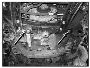
21. Measure ¼" inside of the factory weld seam (or about 3-1/4" from the inside edge of the cam slot) and make a cut line all around the factory crossmember. Make a vertical cut. (Fig 14a, 14b, 14c)
