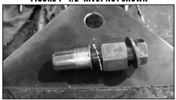
FIGURE 1 - 1/2" RIVET NUT SHOWN
