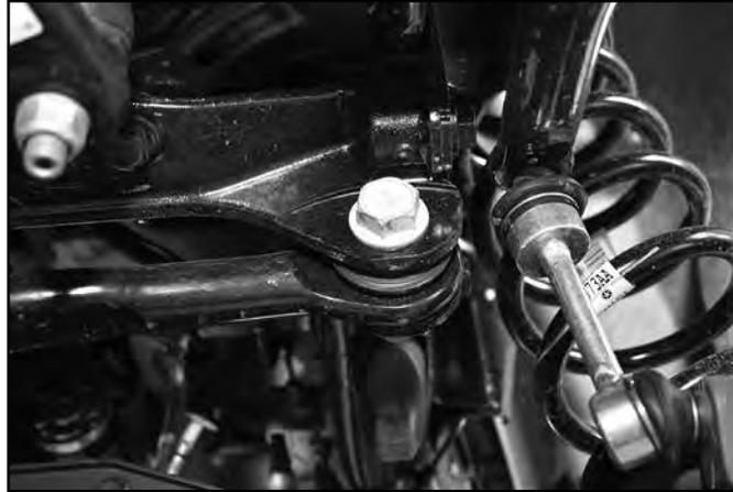
3. Raise the front of the vehicle and support the frame rails with jackstands. Note: The radius arms will be removed during this installation; do not support the weight of the truck on the radius arms.
