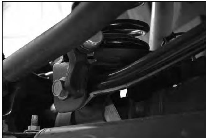
6. Remove the factory sway bar links, they will not be reinstalled. (Fig 3)
