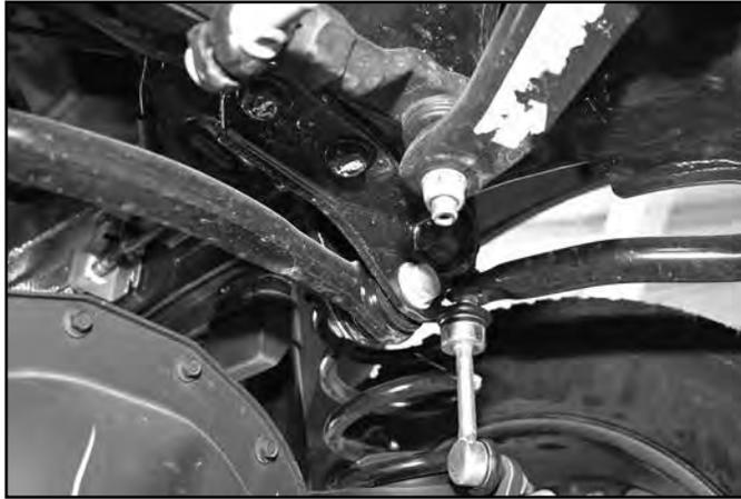
10. Detach the ABS and Central Axle Disconnect wires from retaining clips to allow for extra slack when new coils will be installed.
