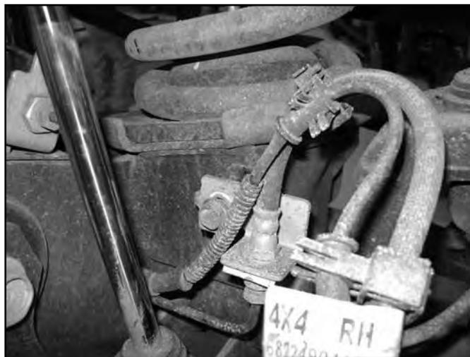
9. It is recommended to disconnect the drag link from the pitman arm at this time. This will prevent the joint from binding while installing new coils. Use care not to damage the drag link joint boot. (Fig 6)
