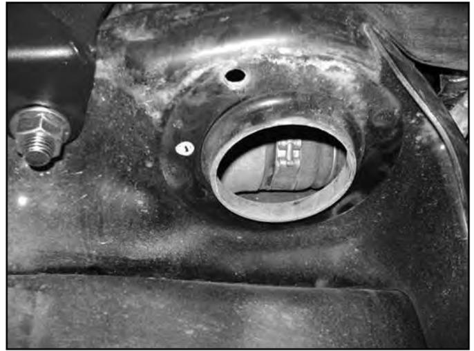
21. Install new coils with the factory isolator on top of the coil. The end of the spring with the windings closer together will go at the top, do not install upside down. Use hydraulic jack to raise the axle to seat the coils. Ensure that the coils are seated properly. Driver's side – Figure 11, Passenger's side Figure 12a, 12b.
