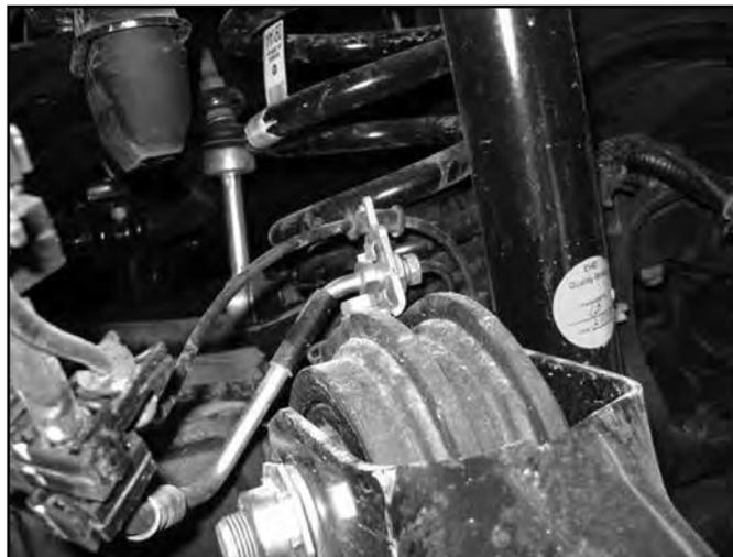
8. Disconnect the brake line from the backside of the axle. Retain hardware (Fig 5)
