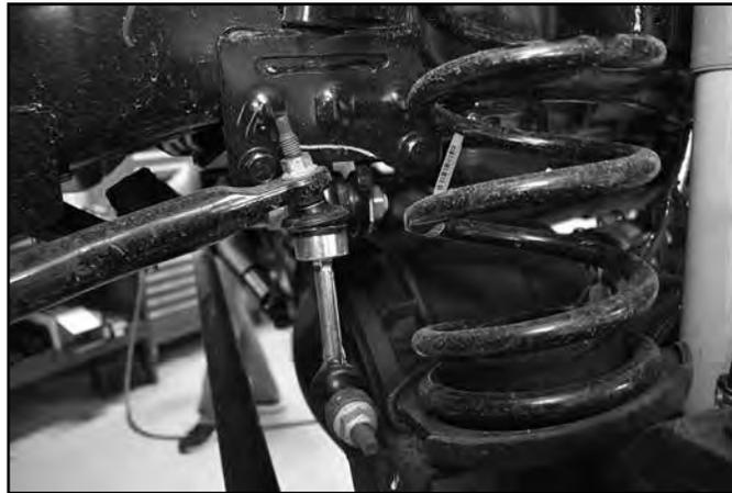
7. Disconnect the brake line bracket from the top of the axle. Retain hardware (Fig 4)
