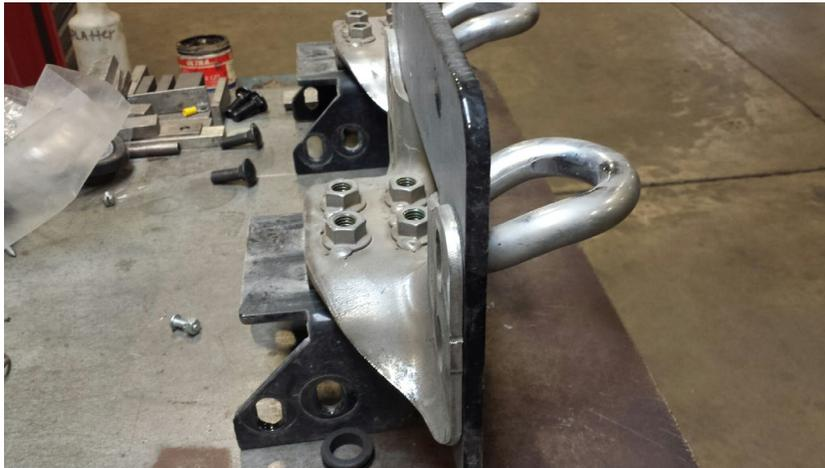
7. Make sure the holes of the tow hook bracket and the holes of the mounting plate line up.
