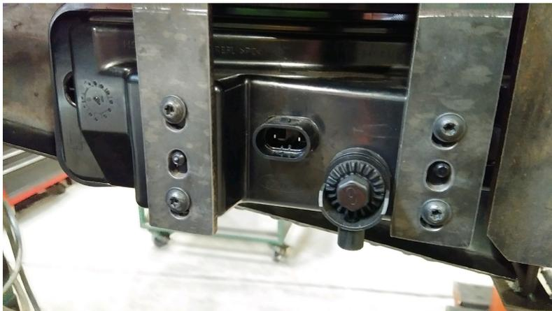
4. There is a driver (LBF171MBDBL) and passenger (LBF171MBPBL) mounting bracket. Mount the fog light mounting bracket to the hole located in the mounting bracket of the replacement bumper. Use 1/2" hardware. Hand tighten only.
