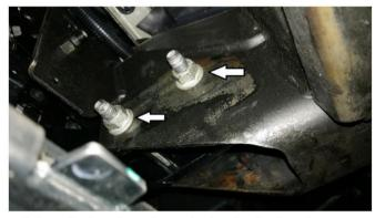
2. Install the bottom brackets by sliding the brackets from the back. The bracket mounts to the outer side of the frame. Reinsert the tow hook and use the 5"  $\times$  ½" bolts to install. If no tow hooks use 1 ½"  $\times$  ½" bolts. You may have to trim the plastic where the brackets come through the tow hook opening.
