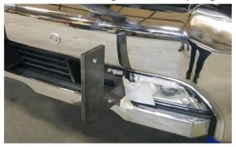
3. To install the top brackets, you will need to remove the factory grille. You will need to remove the side panels first. Start by removing the inner fender well screws. This will allow to get to the back side of the plastic clips. There will also be a small screw in the corner that need to be removed before the side panel can be pulled off.
