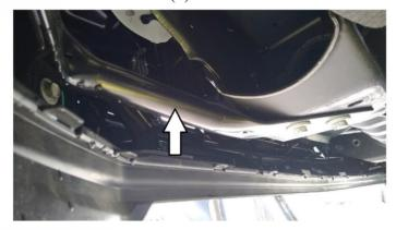
5. On vehicle is with diesel motors, unplug the block heater plug.
