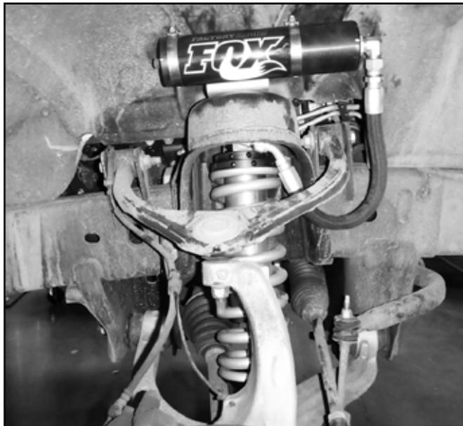
15. Connect the shock assembly to the lower control arm, reusing the stock bolt and nut. Leave hardware loose.
