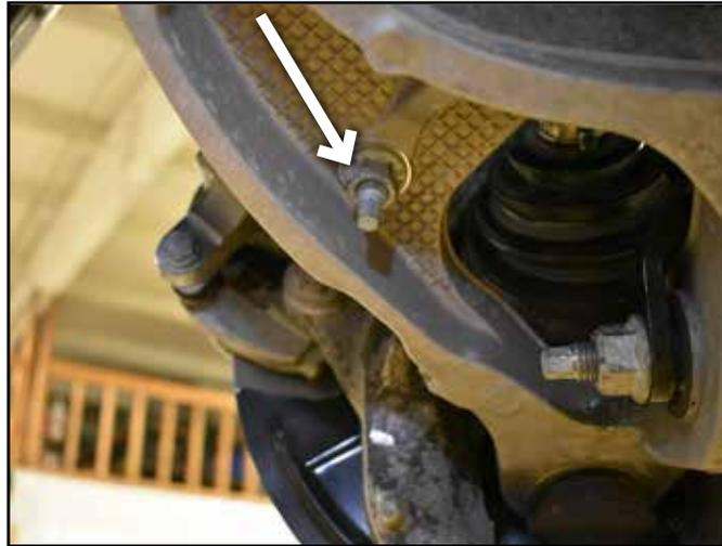
7. Disconnect both outer tie rod ends from spindle steering arm. Save hardware.
