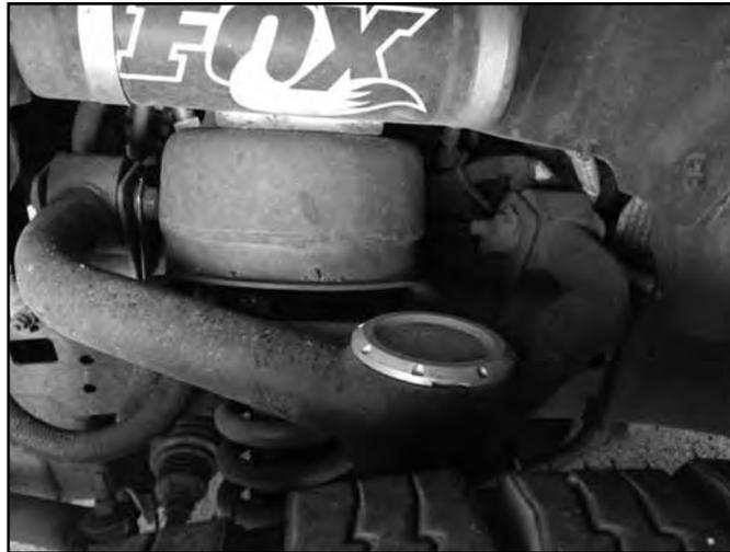
21. 2006-2018 Model year trucks (2019+ skip this step): Attach the ABS wire to the upper control arm with the included ¼" hardware with rubber coated clamp. Note the rubber grommet on the ABS wire can be slid on the main cable. Use silicone spray to aid in movement of grommet if necessary. Tighten to 18 ft-lbs.
