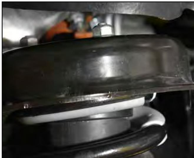
10. Remove the (1) bolt and nut connecting the shock to the lower control arm. (Do not discard bolt and nut as it will be used with your new FOX coil-over kit)
