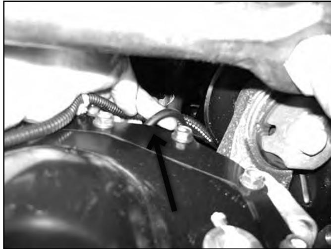
27. Loosen but do not remove all of the front differential mounting bolts/nuts. There are two nuts on the passenger's side (Fig. 20A) and three bolts on the driver's side (Fig 20B - two mount from the bottom up and one from the top down). Remove the rear-most bolt mounting from the top.
