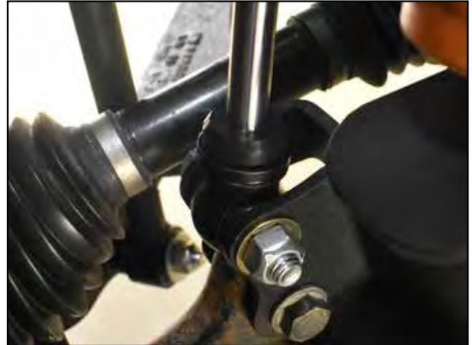
46. With the front shocks installed, torque the front shock bolt at the new torsion bar bracket to 90 ft-lbs. Apply thread locker to the main 1" bolt threads and torque the bolt to 200 ft-lbs.
