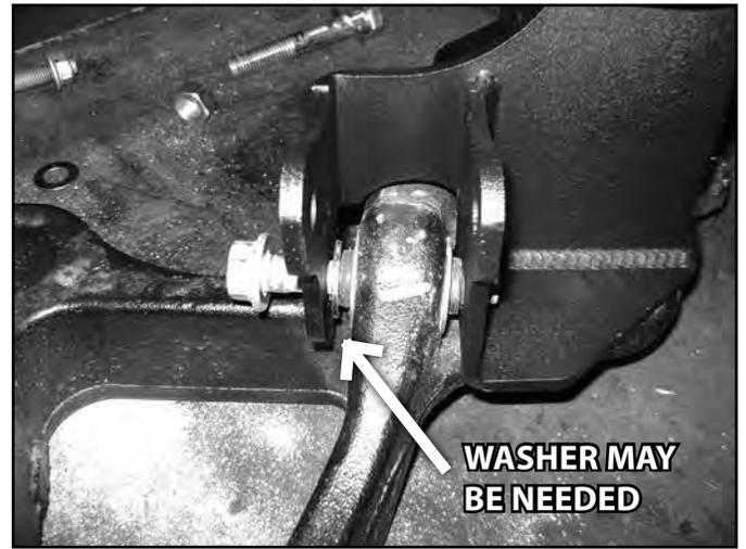
44. With both new torsion bar bracket installed on the factory control arms, install the control arms in the cross members. Fasten the control arms with the provided 18mm x 120mm (front) and 18mm x 140mm (rear) bolts, nuts and 3/4" SAE flat washers (BP #585). Run the front bolts front-to-rear and the rear bolts rear-to-front (Fig. 31). Leave hardware loose. These bolts will be torque with the weight of the vehicle on the suspension.
