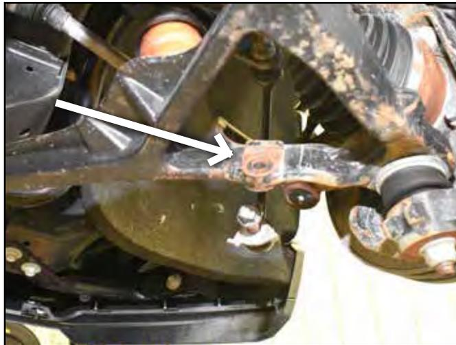
11. Disconnect the tie rod ends from the steering knuckles (Fig. 4). Remove the tie rod end nuts and save. Strike the knuckle near the tie rod end to dislodge the tie rod end taper. Remove the tie rod ends from the knuckles.
