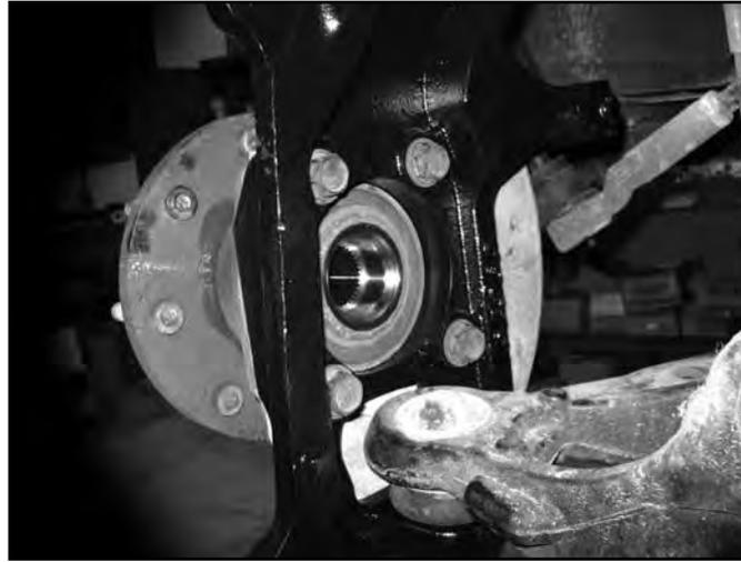
58. Run the ABS line around the back side of the tie rod of the steering knuckle and up to the wire connector on the frame. Reconnect the wire and reattach it to the original place on the frame. Attach the ABS line to the back side of the knuckle near the tie rod end using a wire clamp and a 1/4" x 5/8" bolt, flat washer and lock washer (BP# 877) (Fig. 40).
