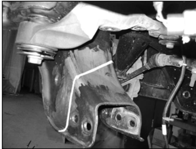
30. Using a reciprocating saw (recommended), cut-off wheel, or plasma cutter, cut the pocket along cut lines. Remove any burrs or rough edges and paint any bare metal to prevent corrosion.
