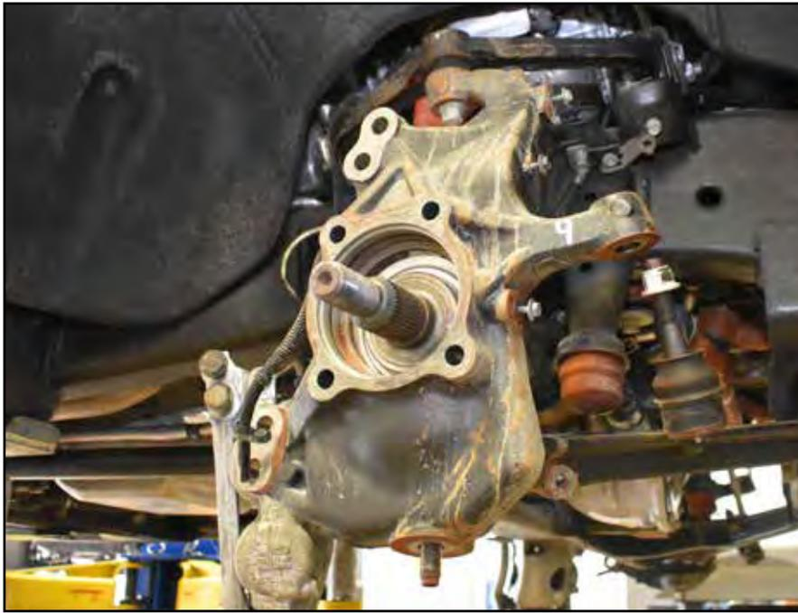
19. Remove the CV axle flange bolts at the differential (Fig. 13). There are 8 bolts per side. Remove the CV shafts from the vehicle and set aside. Save bolts.
