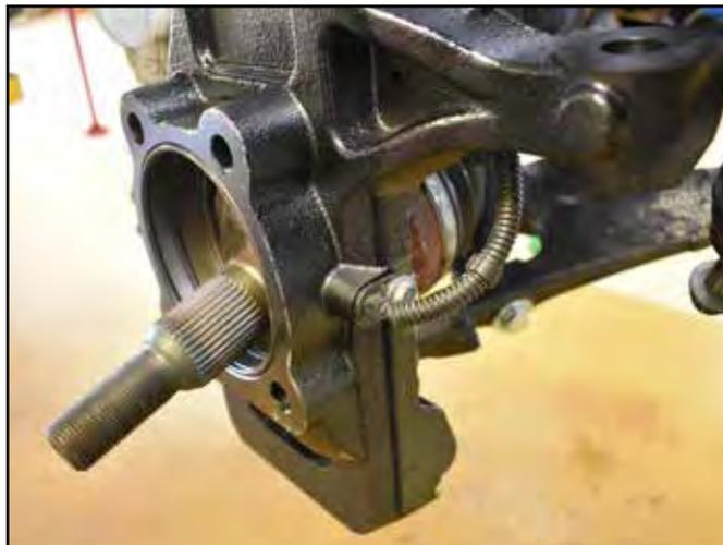
57. Install the hub assembly, O-rings, and dust shield into the appropriate steering knuckle (Fig. 39). Fasten the hub to the knuckle with the factory bolts. Apply thread locker to the threads and torque the bolts to 125 ft-lbs.
