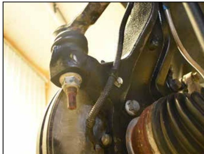
59. Install the torsion bar through the no torsion bar drop bracket, through the factory middle cross member and into the torsion bar keys in the torsion bar cross member. Do not load the torsion bars at this time. Check for clearance to the torsion bar and the middle cross member. Clearance out the middle cross member 1/4" in the area shown in Figure 41. Slide the torsion bar out for ease of access to grind the middle cross member for clearance.
