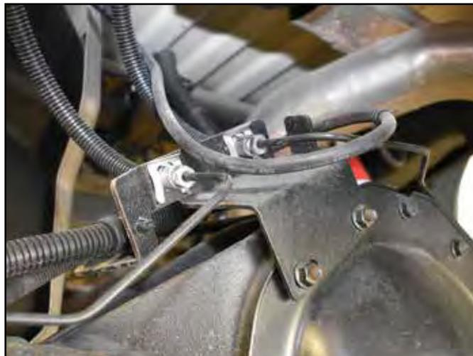
6. Remove the ABS mount from the top of the differential housing. Save hardware, it will be reinstalled later (Fig. 2).
