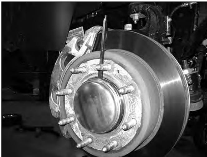
15. Remove the rotor retaining bolt using a T30 torx bit (Fig. 10). Remove the brake rotor and set aside. Save retaining bolt.
