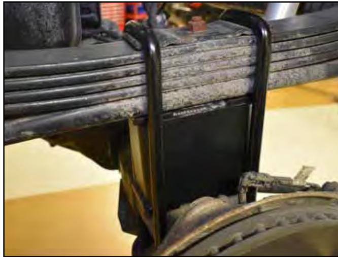
10. Repeat block installation of the driver's side.
