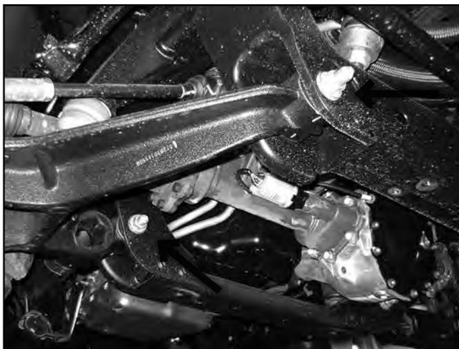
22. There are two factory bump stops per side. Remove front rubber bump stop from the frame mounts on each side. They can be removed with a pair of channel-lock pliers or by striking them with a rubber mallet. Leave the rear bump stop installed in the frame mount.
