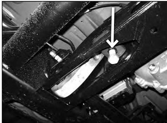
5. Unload the torsion bars but do not remove. Remove and save adjuster bolt/retainer block.
