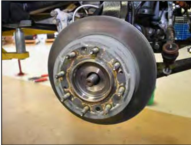
61. Install the original CV axle nut and washer and torque to 155 ft-lbs. Reinstall the hub dust cap.
