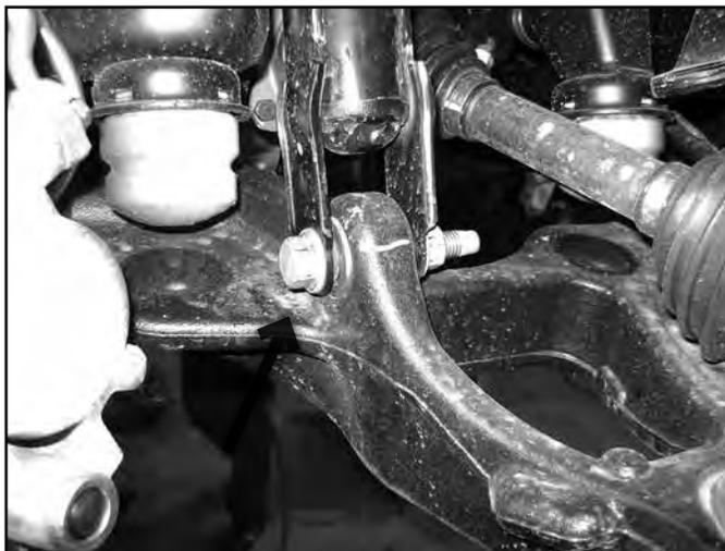
21. Remove the front and rear lower control arm bolts and remove the control arms from the vehicle (Fig. 16). Save the control arms and mounting hardware.
