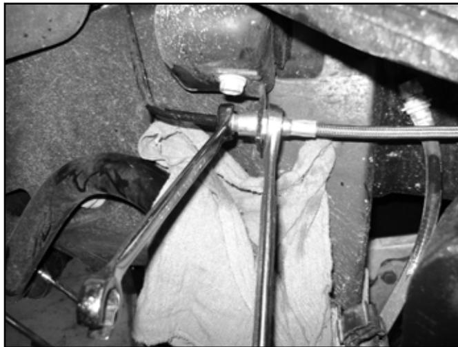
68. There are two threaded holes near the top of the steering knuckle neck on the back side. Using a provided wire clamp, 1/4" x 5/8" bolt, flat washer and lock washer (BP #870) loosely fasten the brake line to the lower threaded hole on the steering knuckle. Using the same fastener combination, attach the ABS line and brake sensor wire to the upper threaded hole. The hardware will be tightened once the line slack is set (Fig. 46).
