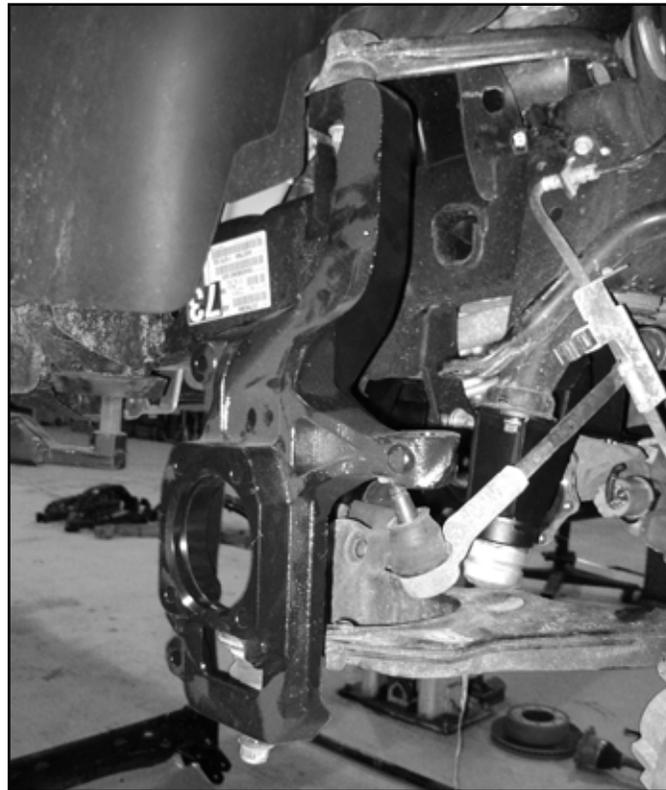
54. Locate the hub o-rings in the factory steering knuckle hub bores. Carefully remove the o-rings (Fig. 36) and install into the new steering knuckles.
