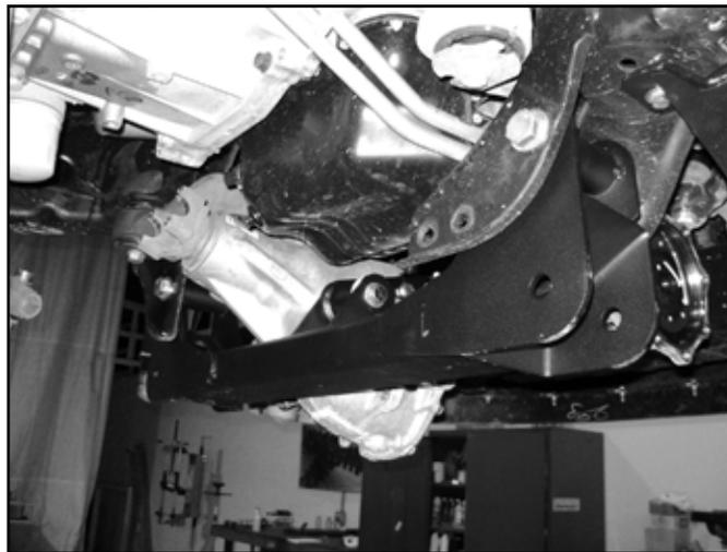
38. With the differential and rear cross member installed, tighten all the differential mount hardware. Torque the (4) 1/2" bolts to 65 ft-lbs and (1) 9/16" bolt to 95 ft-lbs.
