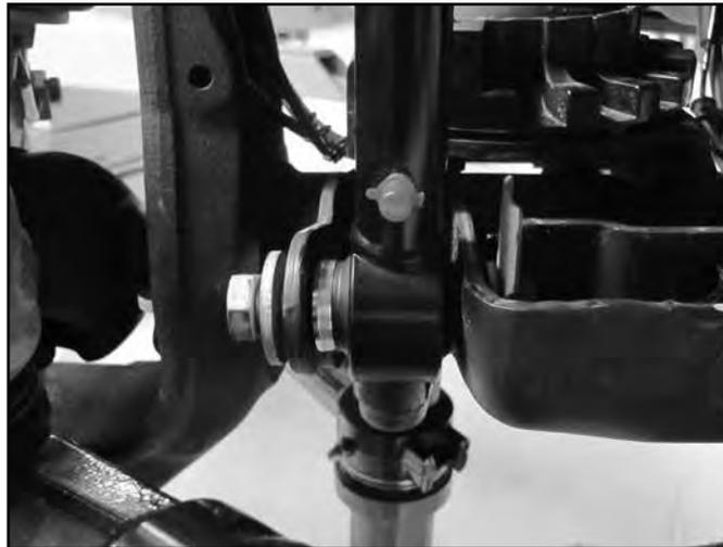
19. Install the remaining longer sleeve on the driver side and slide the polyurethane spacer onto the sleeve so it will mount towards the axle mount tab. Install the quicker disconnect to the inboard side of the axle tab with the original sway bar link hardware.
