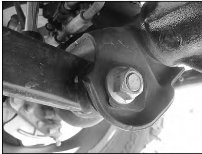
29. Repeat cam washer installation on the passenger side.
