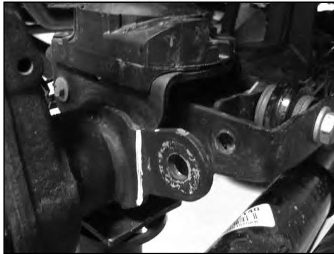
22. Attach the short mounting post into the original sway bar link mount hole on the track bar bracket. Tighten the post ensuring the click pin hole is horizontal or parallel with the ground. Tighten to 65 ft-lbs. (Fig 8)
