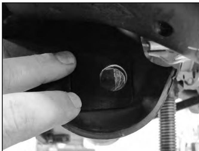
28. When the perforated sections are removed from the lower control arm mount, reinstall the control arm to the axle with cams on factory bolt. Rotate the cams so that the bolt is as far towards the 'rear' of the slot as possible. Just snug the cam hardware so that the cam washers are retained within the stops. Final cam bolt torque will be completed with the weight of the vehicle on the suspension. (Fig 4)
