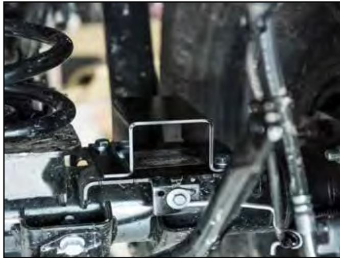
45. Install the hourglass bushings and sleeves into the shocks. Fox shocks install with the body up, NX<sup>2</sup> shocks install with the body down. Install using the factory hardware, torque the upper and lower bolts to 89 ft-lbs
