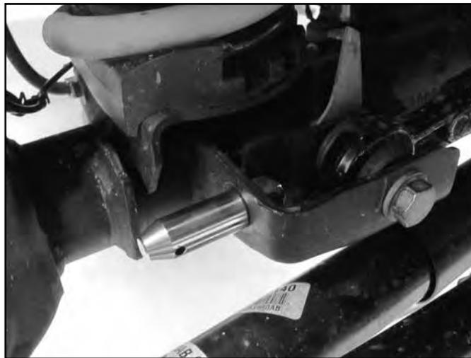
23. Attach the long mounting post with polyurethane spacer into the factory sway bar link mount. The stud should point towards the center of the vehicle. Tighten the post ensuring the click pin hole is horizontal or parallel with the ground. Tighten to 65 ft-lbs. (Fig 9)
