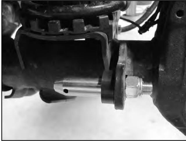
24. Torque the quicker disconnect to sway bar mounting bolts to 65 ft-lbs.
