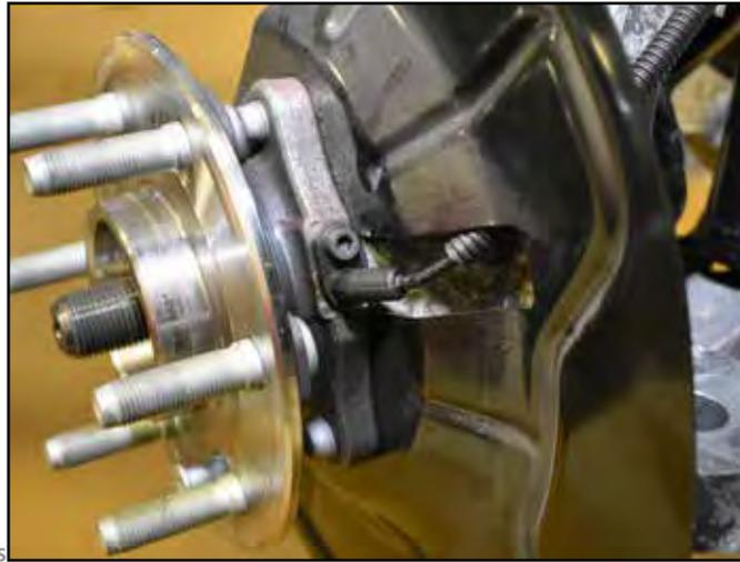
16. Remove ABS sensor from hub (Figure 4). Route the wires and sensor away from the knuckle and tuck out of the way.
