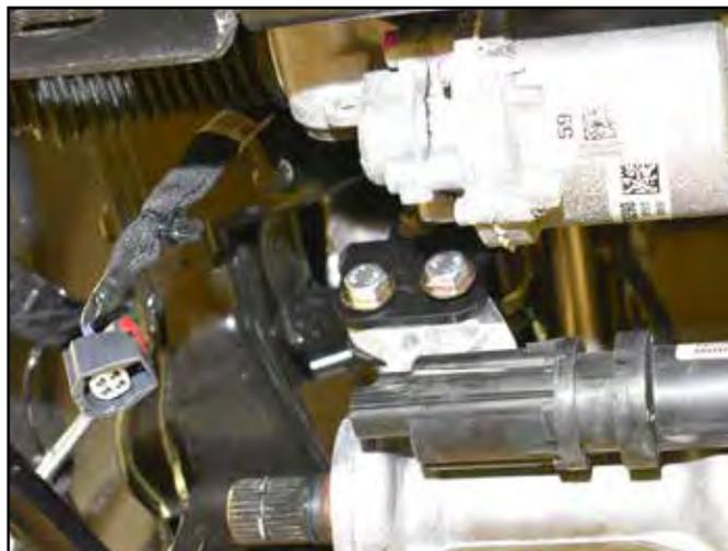
44. Torque all 14 differential mounting bolts. Torque the ½" hardware to 65 ft-lbs and the 12mm hardware to 50 ft-lbs.
