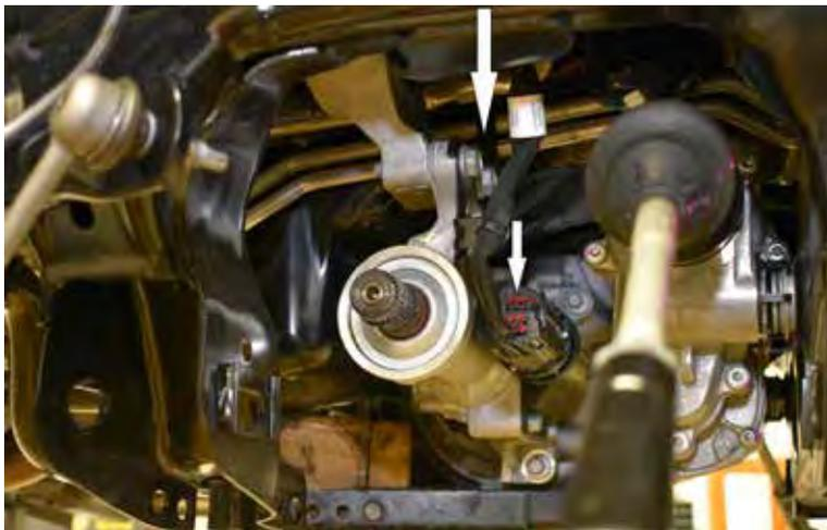
34. With the differential securely supported, remove the remaining bolts and lower the differential from the vehicle.
