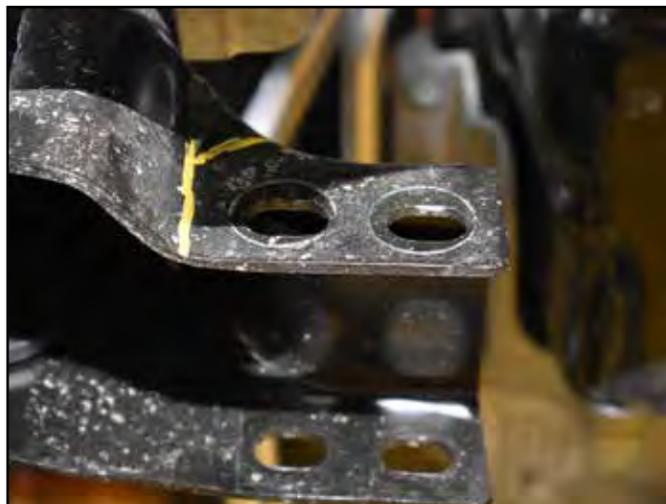
37. Install the provided passenger's side differential drop bracket (03658) to the original frame mount with OE hardware. The brackets should be installed offset forward as shown (Fig 14). Leave hardware loose.
