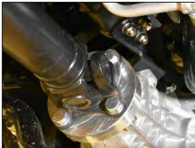
54. On some new vehicles it is necessary to trim a splash guard located on the transmission shift linkage to clear the drive shaft. (Figure 27)
