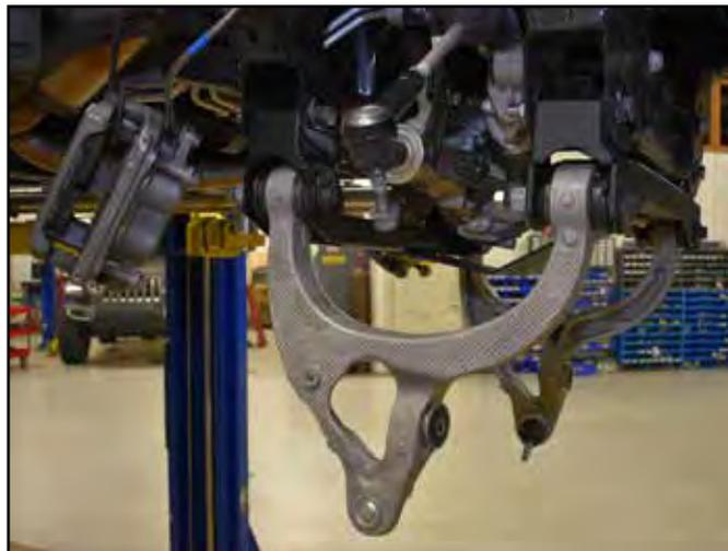
52. With the lower control arms installed, torque the 18mm crossmember mounting bolts to 220 ft-lbs. Torque the ½" differential skid plate hardware to 65 ft-lbs.
