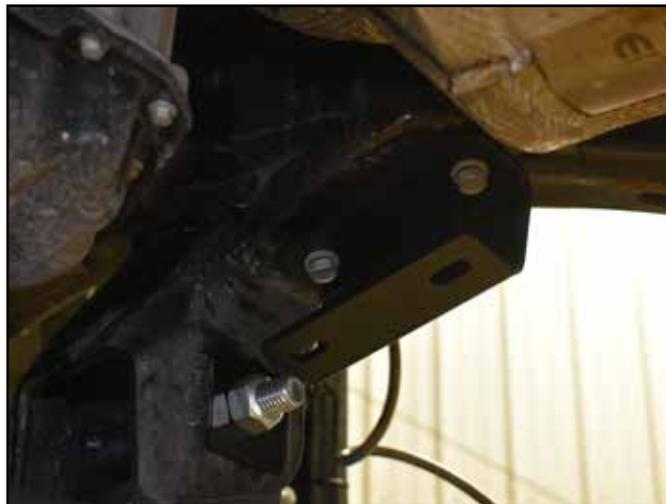
49. Install the new rear crossmember (01296B) in the OE rear lower control arm pockets and loosely fasten with the provided 18mm x 150mm bolts, nuts in conjunction with the provided cam slot washers (03982). Run the bolts from front to rear and leave loose at this time. (Figure 243)
