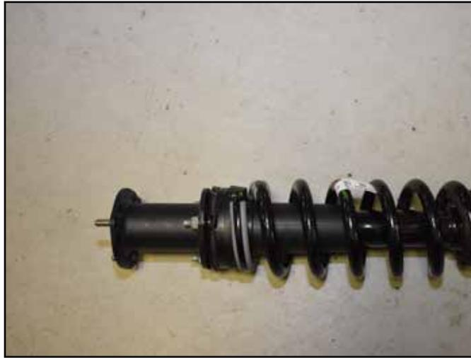
61. Loosely install the strut assemblies on the appropriate sides of the truck with the provided 10mm nuts and washers (BP #481) on the strut spacer studs.
