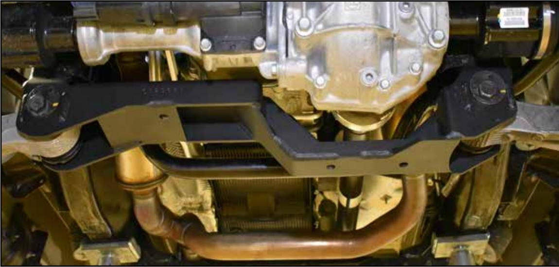
50. Install the new differential skid plate to the front crossmember with  $\frac{1}{2}$ " x  $1\text{-}1/4$ " bolts and  $\frac{1}{2}$ " SAE washers (BP #480) into the welded nuts in the crossmember. Install the back of the skid plate to the rear crossmember with  $\frac{1}{2}$ " x  $1\text{-}1/4$ " bolts and  $\frac{1}{2}$ " SAE washers (BP #480) into the welded nuts in the crossmember. Leave hardware loose. (Figure 24)
