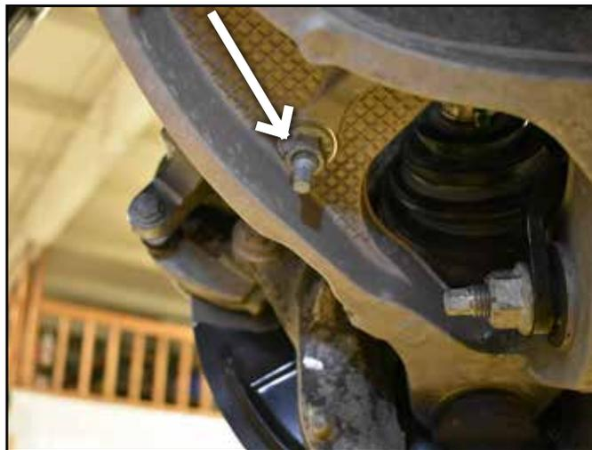
5. Remove and discard the OE front skid plate, if equipped.
