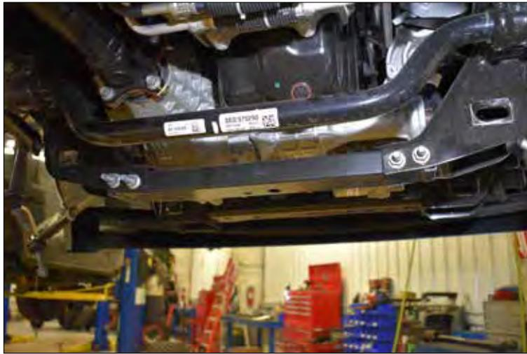
32. Using a jack, support the differential. Loosen and remove the two forward-most differential mounting bolts on the driver's side (Figure 9) you may need to manipulate the wiring harness location in order to give enough clearance for these bolts to come loose.
