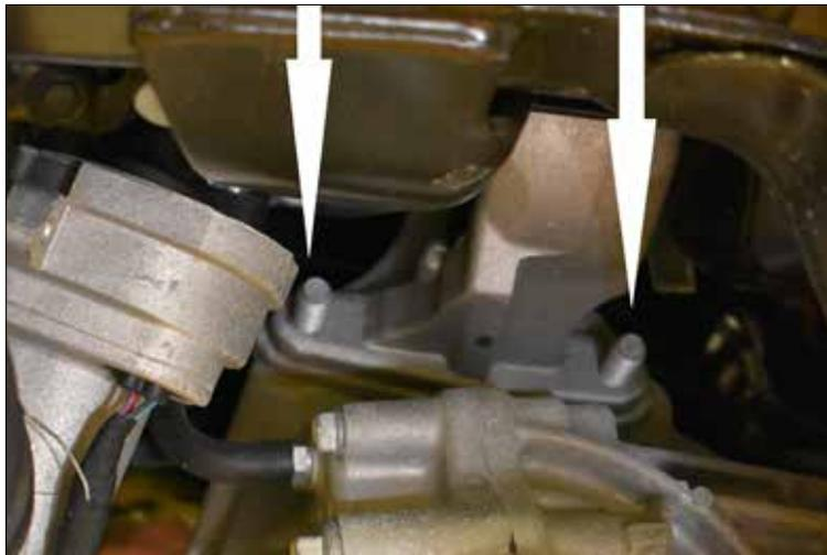
33. Loosen but do not remove the three rear driver's side bolts (Figure 10) and the two passenger's side bolts (Figure 11). On the passenger's side, if equipped, remove the differential actuator cable bracket, it will not be reused. Disconnect the wiring connector from the differential.
