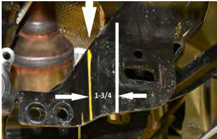
36. Cut the rear passenger side as shown in Figure 13B. Mark 3" from inside edge, cut up to bend in stamped bracket and then cut straight out perpendicular to the angled surface. Cut using a sawsall or equivalent.
