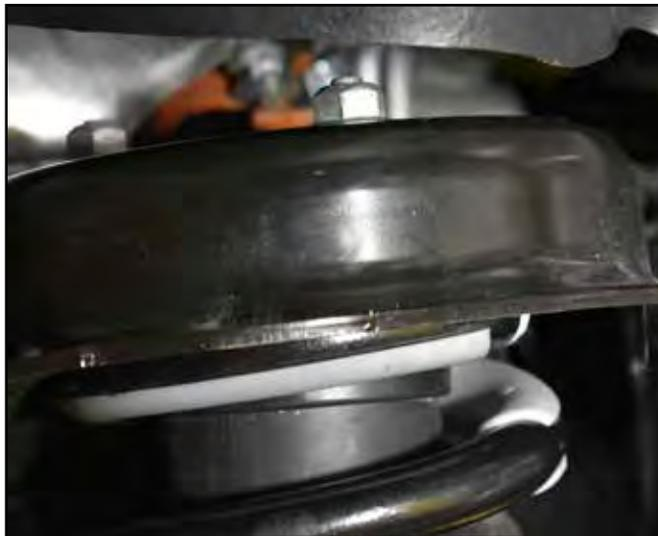
21. Loosen the strut-to-lower control arm hardware. Remove the nut from the bolt and leave the bolt in place to temporarily retain the strut to the lower control arm. Retain the nut.
