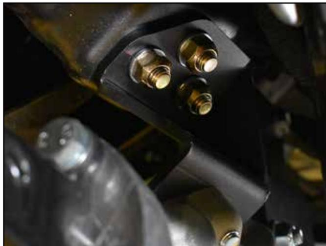
40. Using a jack (and an assistant to aid in balancing) raise the differential up to the new brackets.
