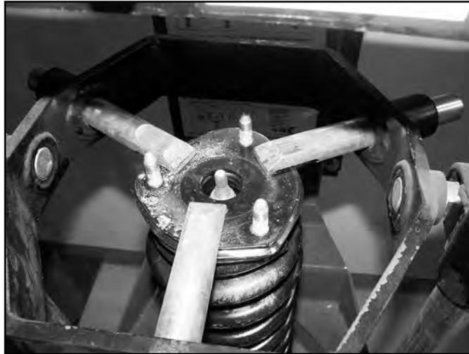
58. Place the provided preload spacer (01278) between the plastic coil seat and the rubber isolator (Figure 31).
