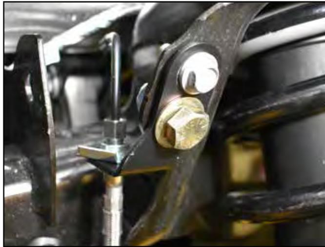
11. Route the new stainless steel brake line through the relocation bracket and attach it to the hard line. Tighten the fitting securely. Fasten the line to the bracket with the provided retaining clip. (Figure 2). Carefully bend the factory hard brake line so that it points downward into the new provided brake line.
