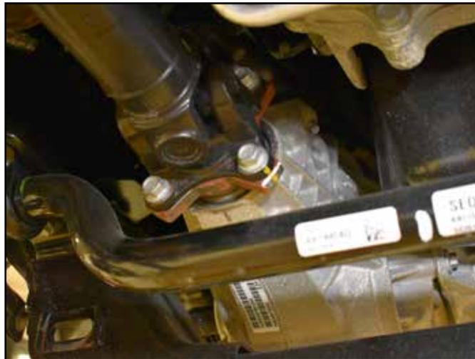
30. Remove sway bar mounts from frame and remove sway bar assembly. Retain Hardware
