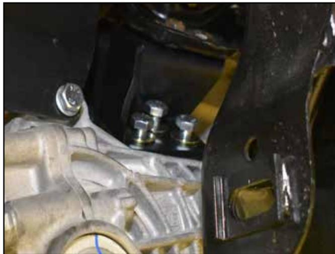
43. Attach the Passenger side differential to the bracket using 12mm x 60mm bolts and washers. (BP 480) (Figure 20)
