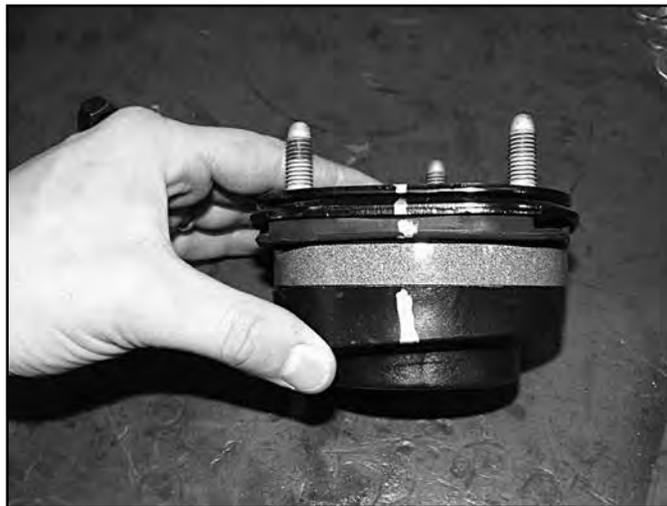
59. Reassemble the strut as it was taken apart by aligning the index marks made earlier. Fasten the assembly with the OE strut nut. Torque nut to 50 ft-lbs.
