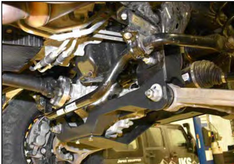
69. Remove stock tie rod ends and replace with provided replacement tie rod ends (401-2038). Attach the tie rod ends to the new steering knuckles with the included nut. Torque to 55 ft-lbs. Securely lock off the jam nut. It is recommended to have approximately 2 threads left exposed past the jam nut for ease of alignment adjustment.
