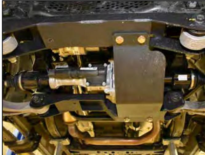
51. Install the lower control arms in the front and rear crossmembers. Attach the control arms to the crossmembers with the OE cam bolts, washers and nuts running from front to rear. Leave hardware loose. (Figure 25)
