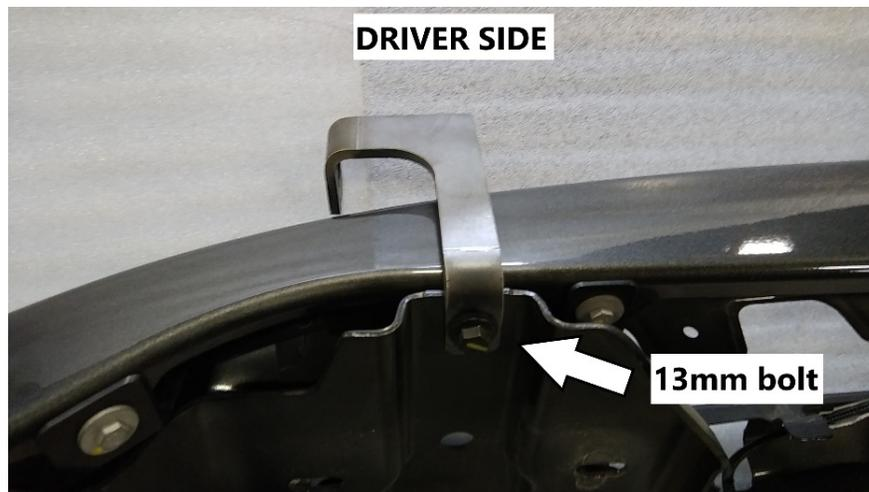
11. Set the top mounting brackets so that they are minimum of 36 ¾" and maximum of 36 7/8" apart.
