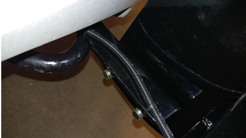
8. Use the two black plugs to cover the holes of the factory sensor holder.
