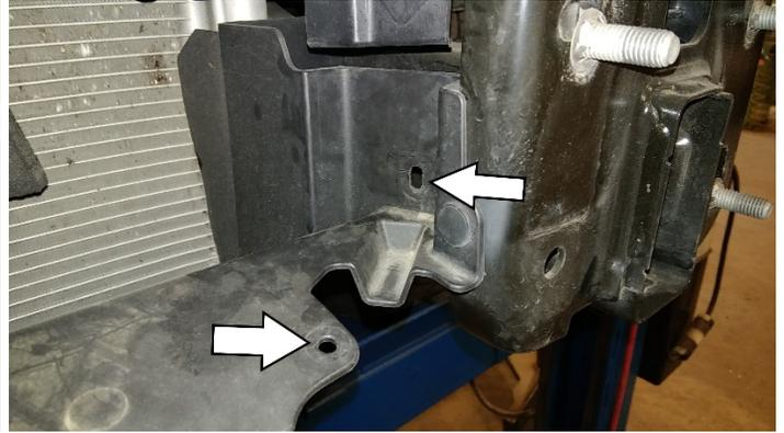
8. Unbolt the bumper by removing the (2) 8mm bolts, *one on each side*, front splash guard bolts and (6) 21mm bumper nuts, *three on each side*.
