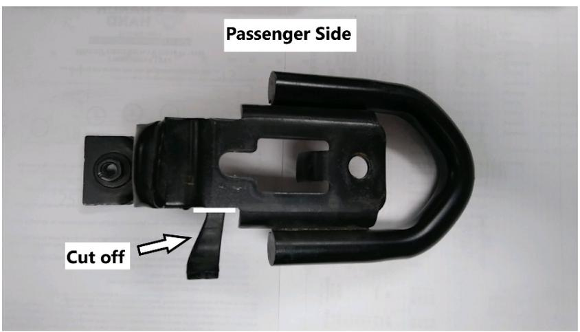
15. Install the bottom brackets and tow hooks (if equipped).
