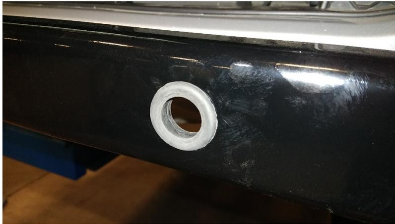
6. Insert sensors into the grommets. You may want to wipe a little WD-40 into the grommet opening to help insert the sensor. (DO NOT TWIST SENSOR).
