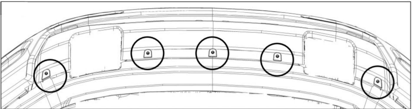
3. Remove the (2) 10mm license plate bolts and unclip license plate bracket from bumper.
