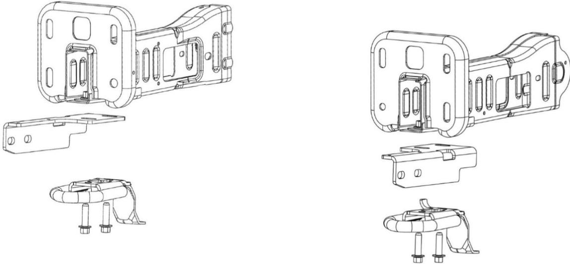
16. Loosely mount the grill guard to the bottom and top brackets using black carriage bolts, washers, and nuts.
