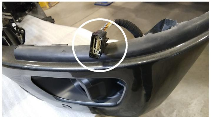
7. On models with sensors and/or adaptive cruise, you will need to unhook the connector from its location to remove the bumper.
