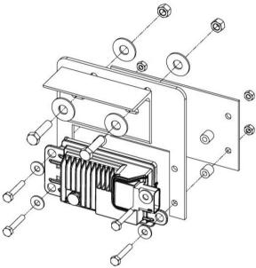
11. **2020-up models**: Mount the Adaptive Cruise Control Module to the Adaptive Cruise Bracket
