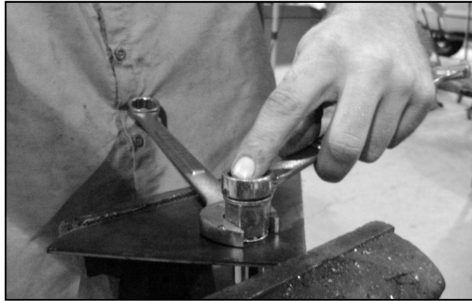
FIGURE 2 - 1/2" RIVET NUT SHOWN
